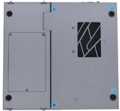
Secure Cassette with screws
