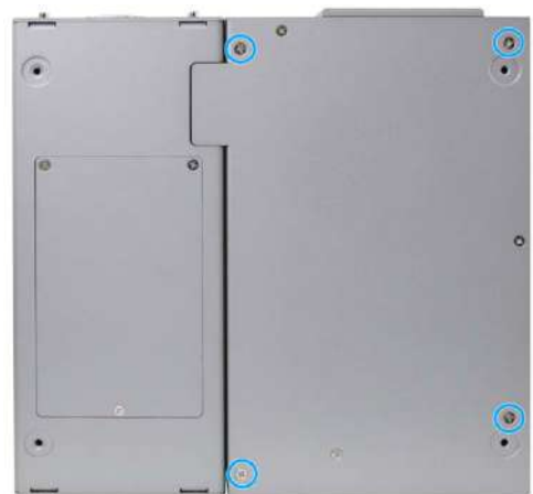
Secure Cassette with screws
