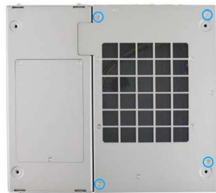
Secure Cassette with screws
