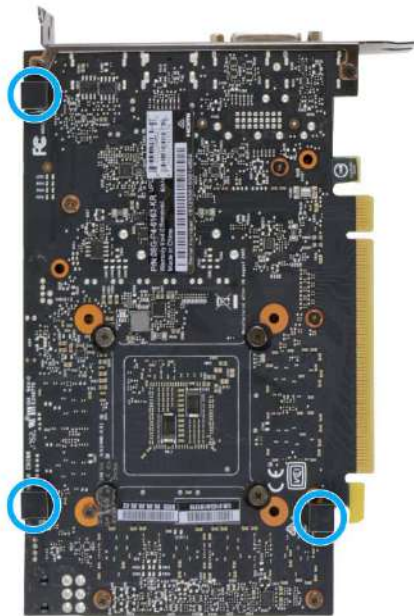
3 rubber stands on back of graphics card
