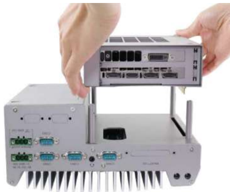
Lower Cassette module onto system
