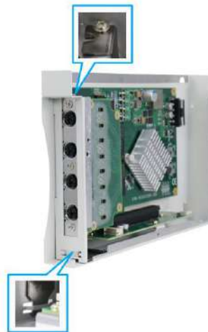
Make sure the card is inserted into the notch and secured with a screw
