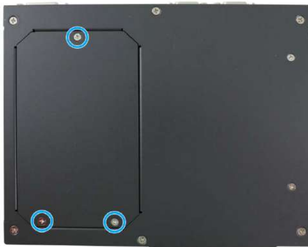
Remove screws indicated
