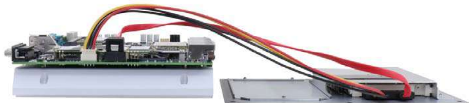
SATA/ power cables connected
