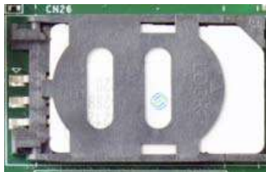
Slide and lift SIM card holder
