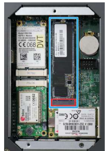
M.2 slot in red, SSD in blue
