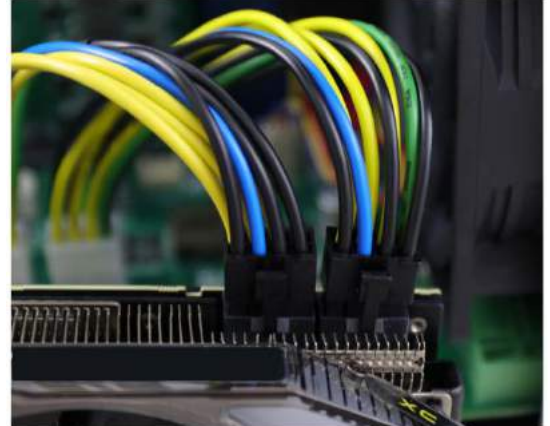
6 or 8/ 8-pin power connector on graphics card
