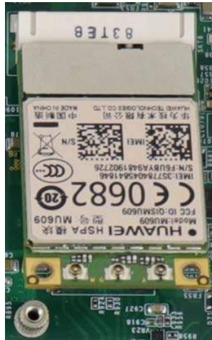
Insert on 45 degree angle
