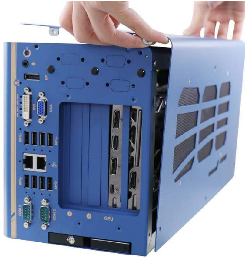
Place L-shape side panel onto the enclosure
