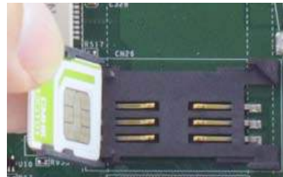
Insert Mini-SIM card with pins facing up
