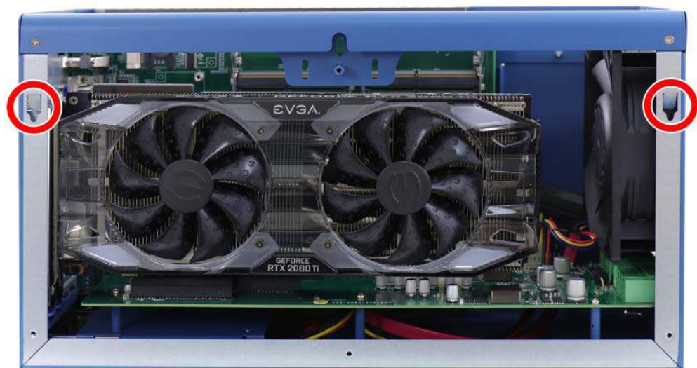
Slide-and-lock into the indicate hinges
