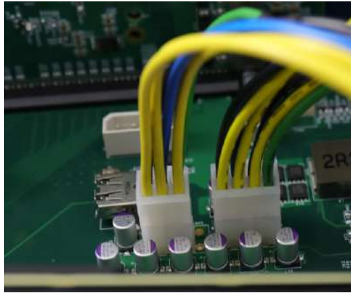
6/ 8-pin power connector on daughter board
