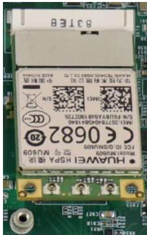
Insert on 45 degree angle
