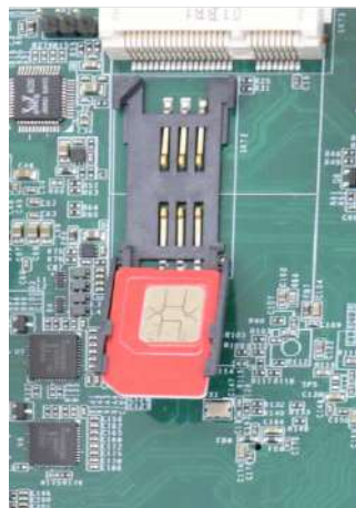
Insert SIM with pins facing upward
