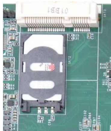
Close and slide the holder to secure SIM
