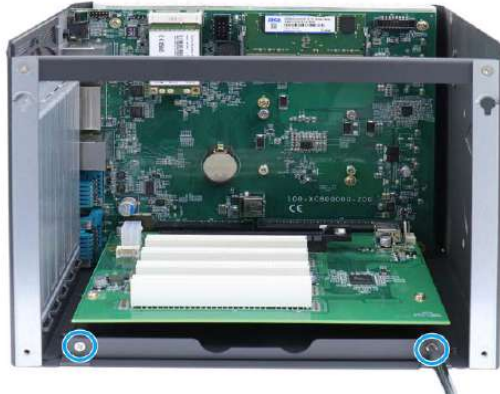
Remove the screws indicated
