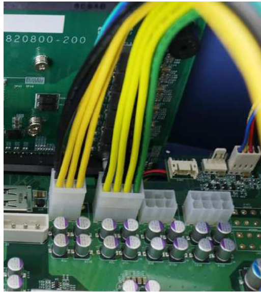
6/ 8-pin power connector on daughter board
