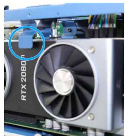
Make sure bracket DOES NOT OBSTRUCT graphics card's fan
