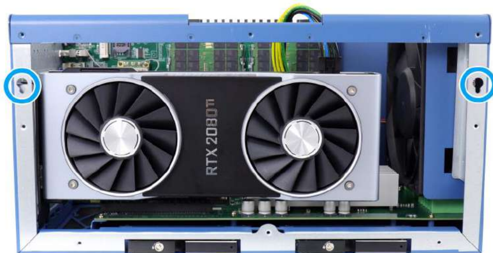
Slide-and-lock into the indicate hinges
