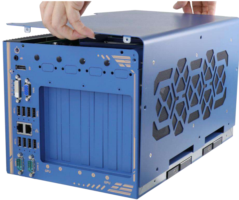
Place L-shape side panel onto the enclosure
