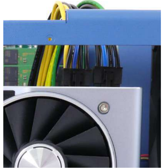
6 or 8/ 8-pin power connector on graphics card
