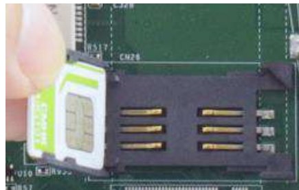
Insert Mini-SIM card with pins facing up
