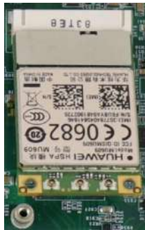
Insert on 45 degree angle
