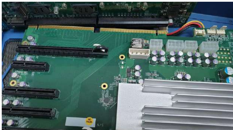
Disengage the daughter-board from the motherboard
