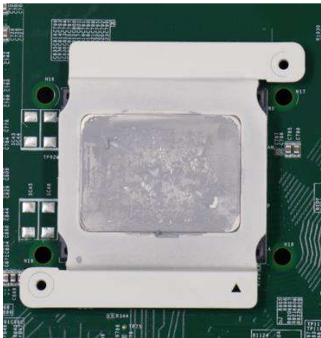
CPU retention bracket (holder)
