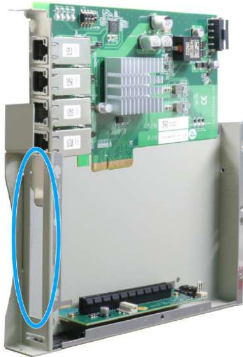
Remove bezel cover and insert the card
