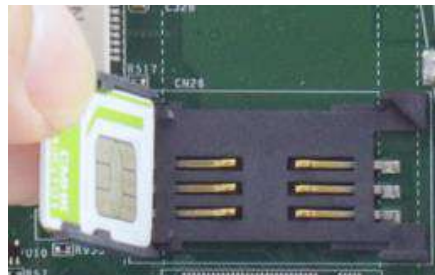
Insert Mini-SIM card with pins facing up
