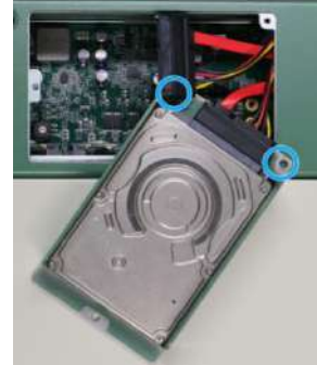
HDD/SSD tray installation orientation
