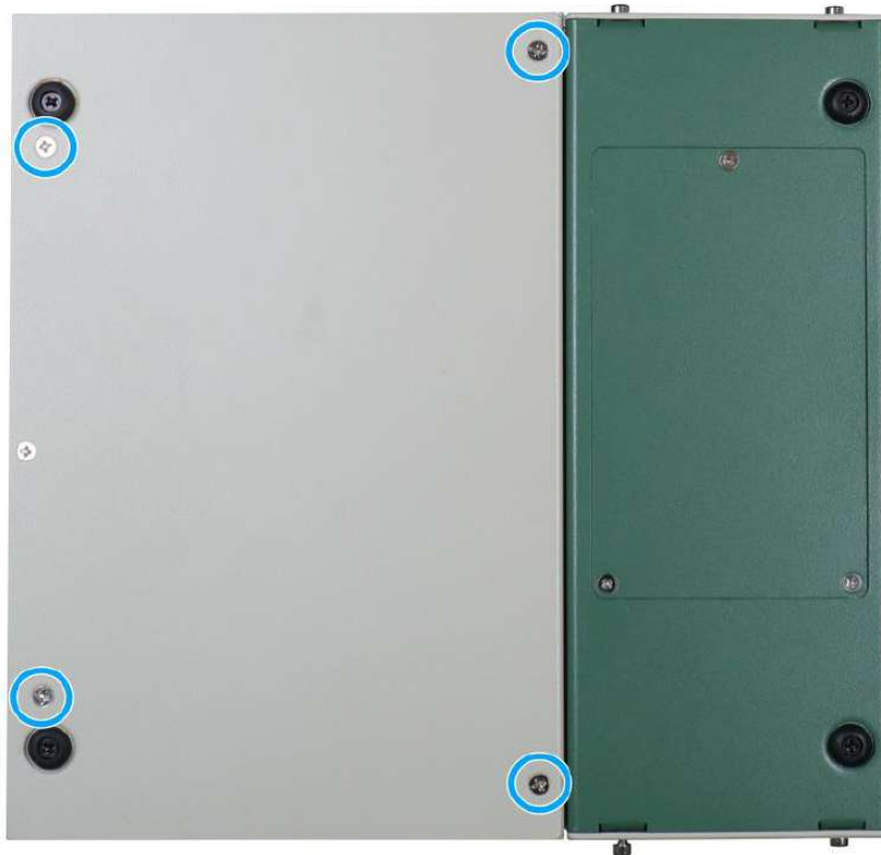
Secure the screws indicated
