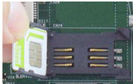
Insert Mini-SIM card with pins facing up
