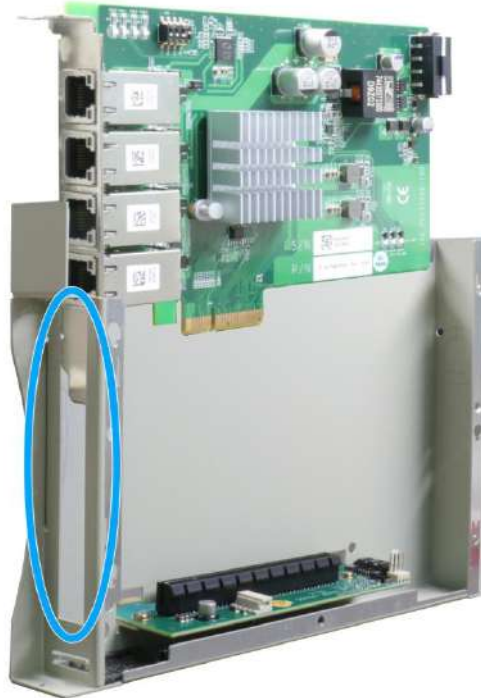
Remove bezel cover and insert the card
