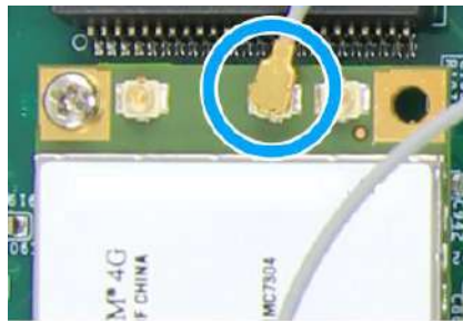
Clip on IPEX-to-SMA cable
