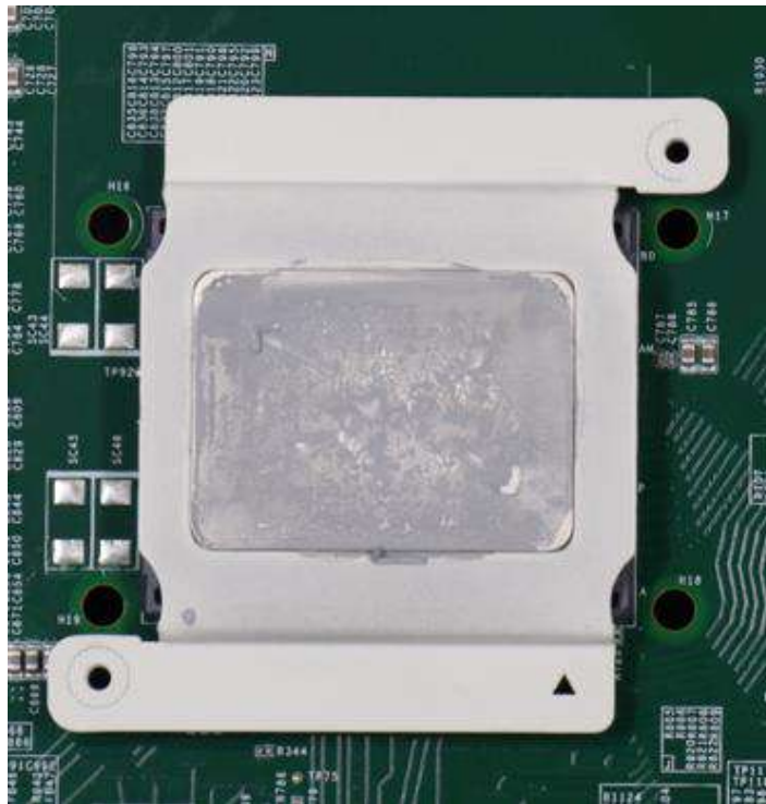
CPU retention bracket (holder)
