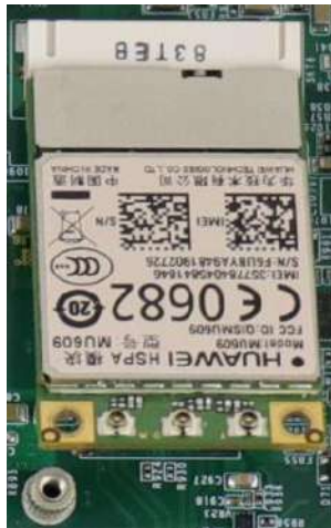
Insert on 45 degree angle
