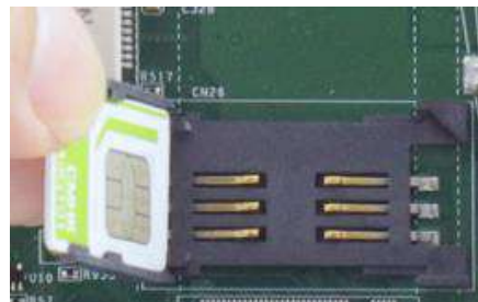
Insert Mini-SIM card with pins facing up
