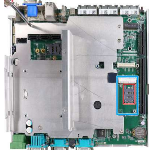
mini-PCIe slot on motherboard (underneath MezIO™ card)
