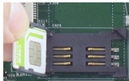
Insert Mini-SIM card with pins facing up
