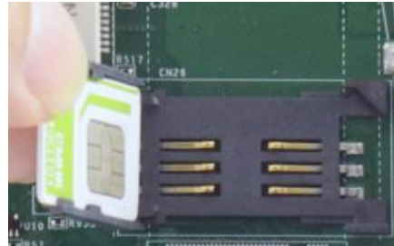
Insert Mini-SIM card with pins facing up
