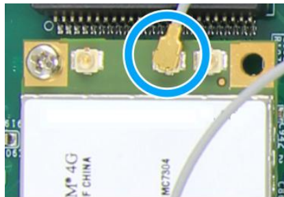
Clip on IPEX-to-SMA cable
