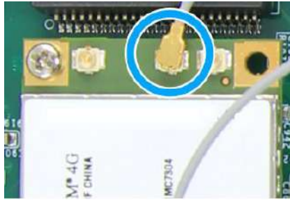
Clip on IPEX-to-SMA cable
