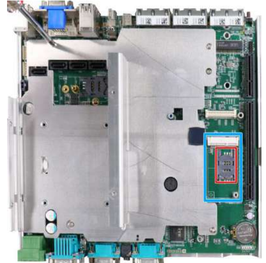
mini-PCIe slot on motherboard (underneath MezIO™ card)
