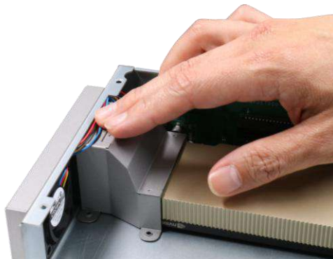
Reinstall the duct
