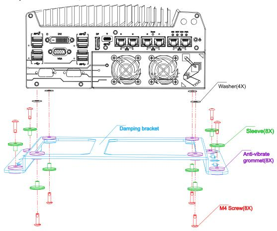
The damping bracket performs best when the system is installed horizontally.
