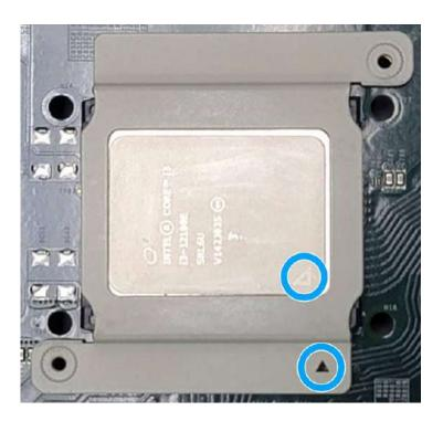
7. Turn the motherboard around while holding the CPU retention bracket in-place, and secure the bracket by tightening two M3 P-head screws on the other side of the motherboard.
