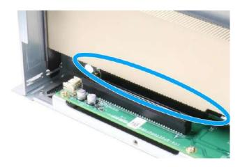
Properly inserted into the PCle slot
