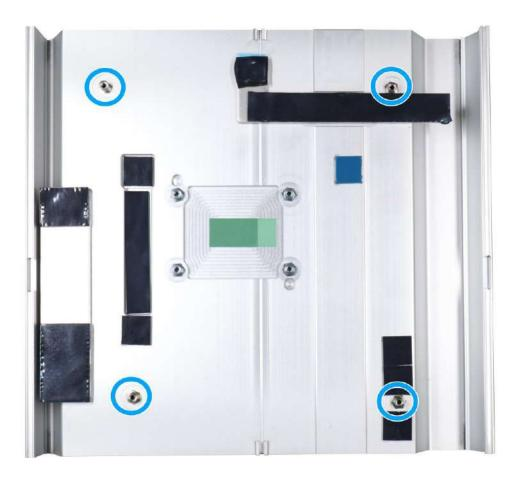
12. Once the motherboard has been installed, you're ready to secure the four screws that help the heatsink apply pressure to the CPU/ chipset die. You'll want to apply even pressure to the corners by gradually tightening each screw. Please refer to the recommended order when tightening the screws.
