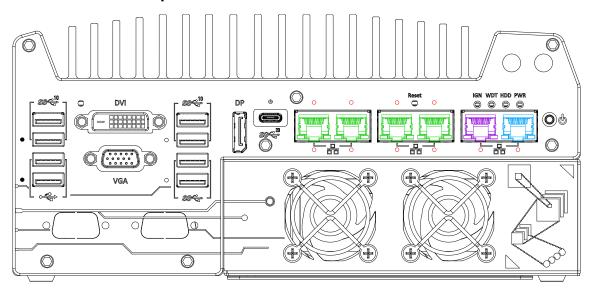
The system offers one GbE port (in blue) and five 2.5GbE ports (in green and purple) with four optional Power over Ethernet ports (in green). All Ethernet ports feature panel screw fix holes for a firm connection (indicated in red). The port marked in blue is implemented using Intel® I219-LM controller that supports Wake-on-LAN and is also compatible with Intel® AMT (Active Management Technology) to support advanced features such as remote SOL desktop and remote on/ off control.
