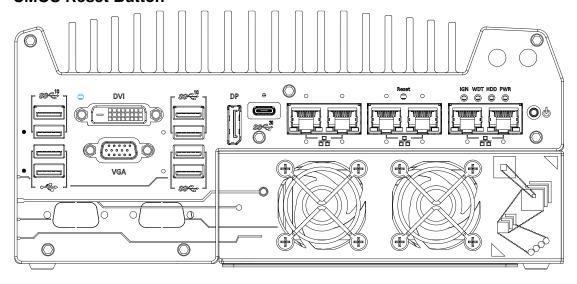
The CMOS Reset button is used to manually reset the motherboard BIOS in case of system halt or malfunction. To avoid unexpected operation, it is purposely placed behind the panel. To reset, disconnect the DC power input, and use the tip of a pen to press and hold for at least 5 seconds to reset the BIOS.
