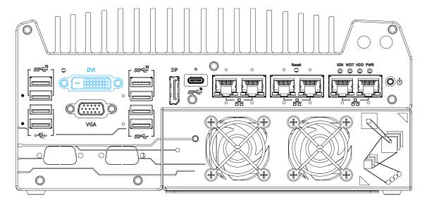
DVI-D transmits graphics data in digital format and therefore can deliver better image quality at high resolution. The DVI connector on the front panel can either output DVI signals or other digital signals (via an adapter/ cable) depending on the display device connected. It supports resolutions up to 1920x1200@60Hz.
