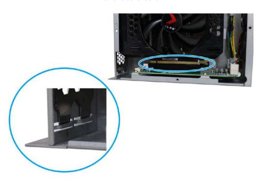
Make sure the card is inserted into the notch and PCle slot
