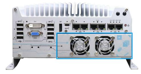
The Cassette module compartmentalizes the heat generated and effectively manages thermal conditions of both the system and graphics card. The modular design reduces the complexity of installing and replacing graphics cards in the fanless controller. In addition, the mechanical design creates a sealed wind tunnel to bring in cold air and expels hot air via system fans to offer the system extreme stability and reliability.
