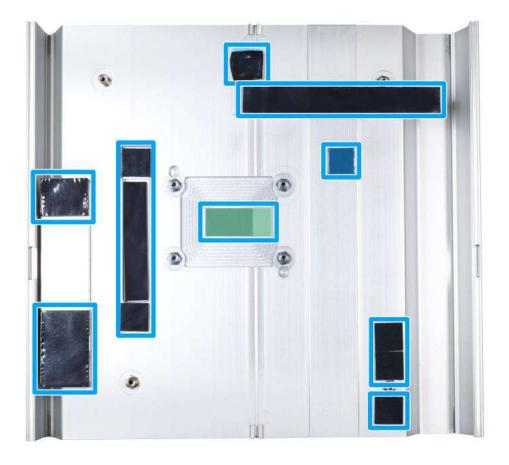
With the four motherboard standoffs aligned, gently lower the motherboard onto the heatsink and secure the four screws. Please remember to remove the protective film (indicated in red) on the CPU's thermal pad as well.
