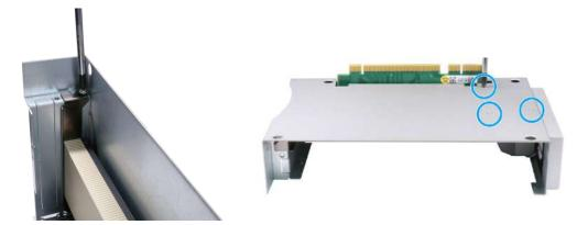
Remove the screws securing the graphics card
