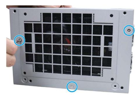
10. Gently lower the Cassette module back onto the system enclosure and secure the module onto the system enclosure by securing the following screws.
