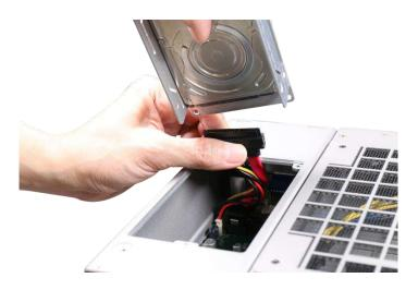
6. Gently put the tray back into the system with the connector side being inserted into the system first and secure the tray with three screws.
