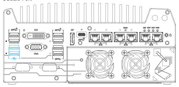
The USB2.0 ports are implemented via native xHCI (eXtensible Host Controller Interface) and are backward compatible with USB 1.1 and USB 1.0 devices. UEFI USB support is also provided so you can use USB keyboard/ mouse in UEFI shell environment. Indicated in red is a screw-lock hole for the corresponding USB port.
