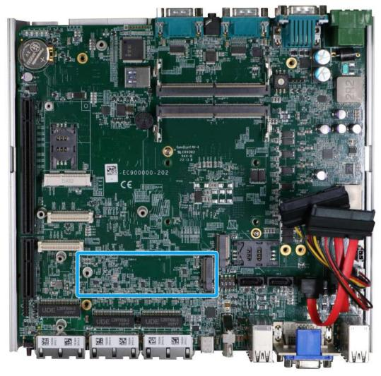
The system has a Gen4 x4 PCIe M.2 2280 slot for you to install an NVMe SSD. For installation, please refer to the following instructions.
