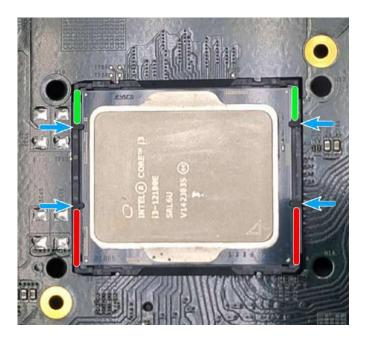
9. Make sure all thermal pad residues have been cleaned on both sides of the retention bracket. Place the CPU retention bracket (holder) on top of the CPU and hold it in place. Make sure the indicator triangle engraved on the CPU's integrated heat spreader (HIS) and the triangle indicator on the retention bracket are positioned in the same corner (indicated by blue circles).
