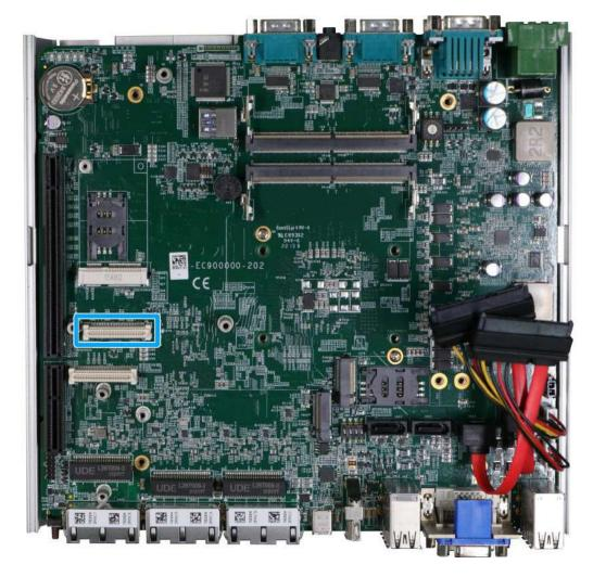
MezIO<sup>™</sup> is an innovative interface designed for integrating application-oriented I/O functions into an embedded system. It offers computer signals, power rails and control signals via a high-speed connector. MezIO<sup>™</sup> is also mechanically reliable benefited from its 3-point mounted mezzanine structure. A MezIO<sup>™</sup> module can leverage these signals to implement comprehensive I/O functions.
