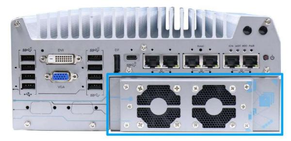
The Cassette module compartmentalizes the heat generated and effectively manages thermal conditions of both the system and graphics card. The modular design reduces the complexity of installing and replacing graphics cards in the fanless controller. In addition, the mechanical design creates a sealed wind tunnel to bring in cold air and expels hot air via system fans to offer the system extreme stability and reliability.
