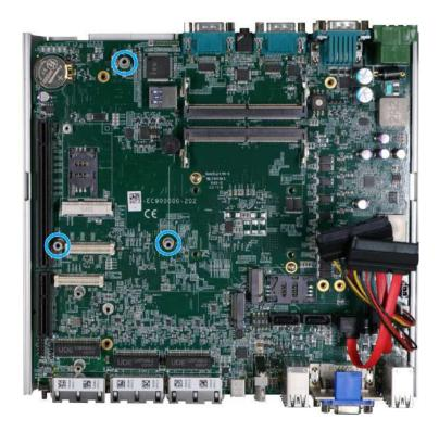
Gently lower the MezIO<sup>™</sup> module onto the three stand-mounts while matching the MezIO<sup>™</sup> interface. Secure the module using three screws supplied.
