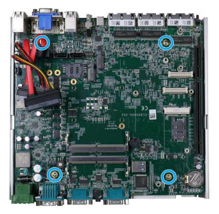
Secure motherboard with four screws
