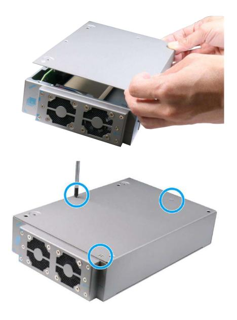
10. Gently lower the Cassette module back onto the system enclosure and secure the module onto the system enclosure by securing the following screws.
