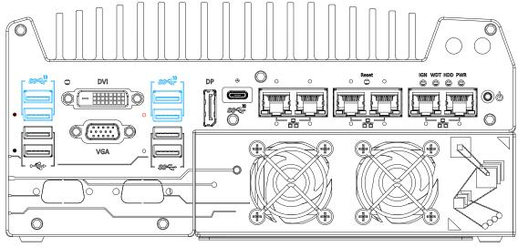
The system's USB 3.2 Gen2x1 ports (10Gbps) are implemented via native xHCI (eXtensible Host Controller Interface) controller and are backward compatible with USB3.2 Gen.1 USB 2.0, USB 1.1 and USB 1.0 devices. UFEI USB is also supported so you can use USB keyboard/mouse in UEFI shell environment. Indicated in **red** are screw-lock holes for the corresponding USB port.
