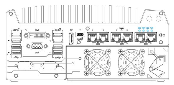
There are four LED indicators on the I/O panel: IGN, WDT, HDD and PWR. The descriptions of these four LED are listed in the following table.
