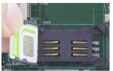
Insert Mini-SIM card with pins facing up
