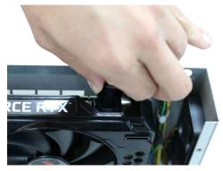
Remove the screws securing the graphics card
