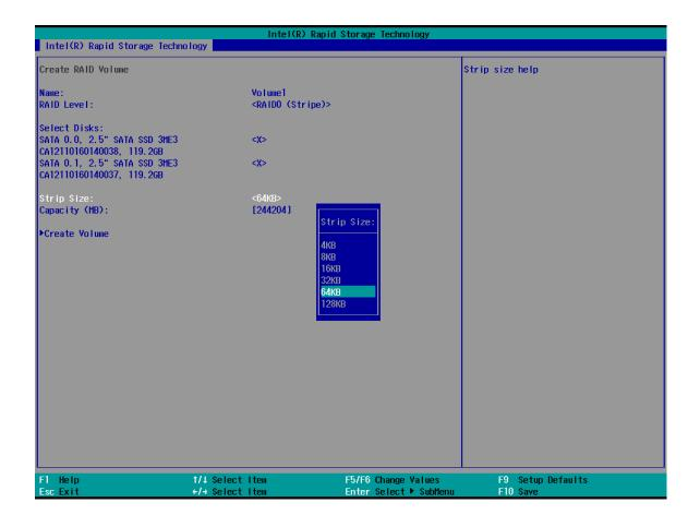
7. The Capacity (MB) option allows you to configure the storage capacity of your RAID volume. By default, the full storage capacity will be applied. Once you have entered a capacity, press ENTER to confirm.
