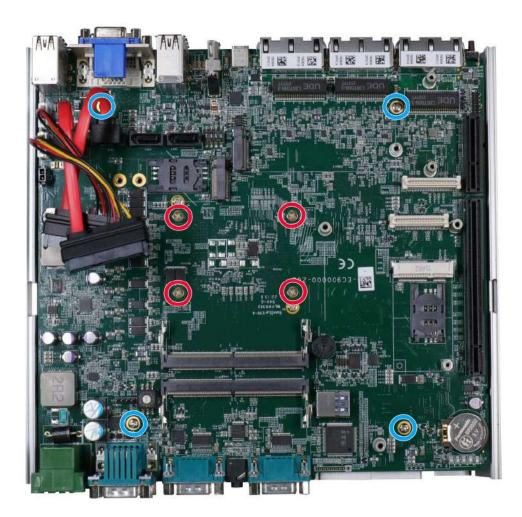
4. Remove the screws indicated once you separate the heatsink from the motherboard to remove the CPU holder.
