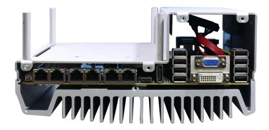
5. On the rear I/O panel, remove the hexa-screws indicated below.
