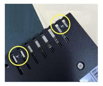
For Sparkle graphics card, remove the two screws at the back of the graphics card (towards the end). Once the graphics card is installed into the Cassette module, these two screw holes will be used to secure the graphics card in place.
