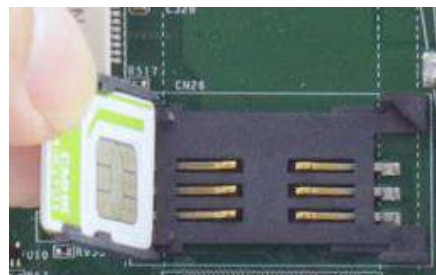
Insert Mini-SIM card with pins facing up
