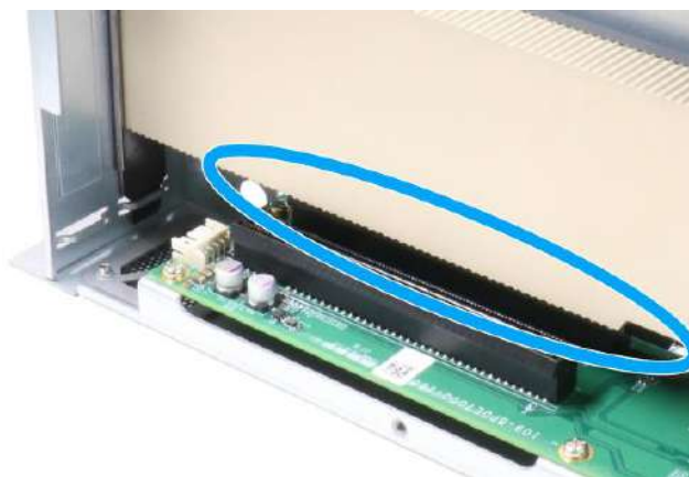
Properly inserted into the PCIe slot
