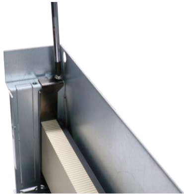
Remove the screws securing the graphics card
