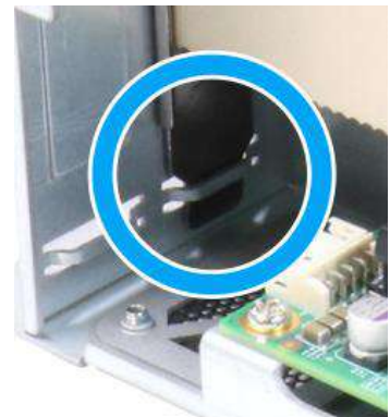
Bezel inserted into the notch
