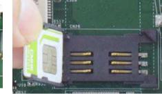
Insert Mini-SIM card with pins facing up
