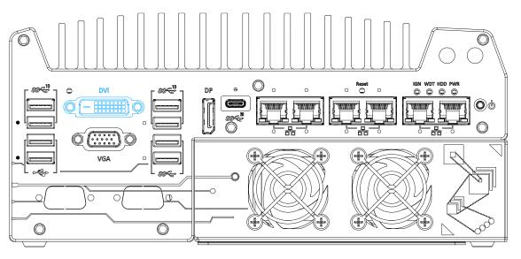
DVI-D transmits graphics data in digital format and therefore can deliver better image quality at high resolution. The DVI connector on the front panel can either output DVI signals or other digital signals (via an adapter/ cable) depending on the display device connected. It supports resolutions up to 1920x1200@60Hz.
