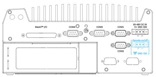
The "Remote On/ Off" 3-pin connection allows for the connection of an external non-latched switch to turn on/ off the system. It is useful when the system is placed in a cabinet or a not easily accessed location. You may connect an external status LED (20mA) indicator by connecting to PWR LED and GND.
