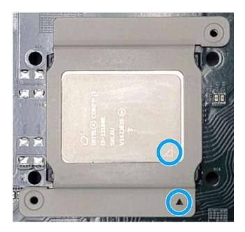
10. Turn the motherboard around and secure the bracket by tightening two M3 P-head screws.
