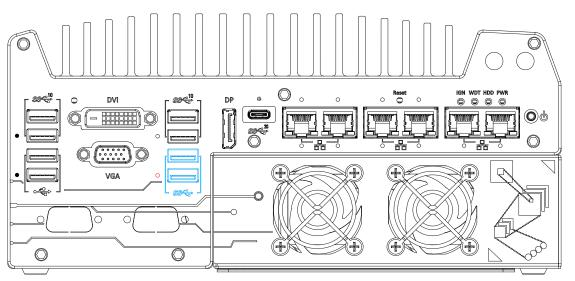
The system's USB 3.2 Gen1x1 ports (5Gbps) are implemented via native xHCI (eXtensible Host Controller Interface) controller and are backward compatible with USB 2.0, USB 1.1 and USB 1.0 devices. UEFI USB is also supported so you can use USB keyboard/mouse in UEFI shell environment. Indicated in **red** is a screw-lock hole for the corresponding USB port. xHCI driver is supported natively in Windows 10, therefore you do not need to install the xHCI driver prior to utilizing USB functions.
