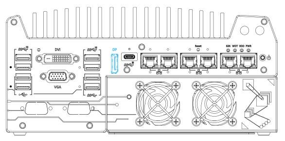
The system has a DisplayPort (DP) output which is a digital display interface that mainly connect video source and carry audio to a display device. When connecting a DP, it can deliver up to 4K UHD (4096 x 2304 @ 60Hz) in resolution. The system is designed to support passive DP adapter/ cable. You can connect to other display devices using DP-to-HDMI cable or DP-to-DVI cable.
