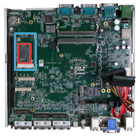
Before installing the mPCIe module, you need to insert the Mini-SIM card. Slide the SIM slot holder and lift the SIM card holder. Insert the Mini-SIM card (pins facing up), shut the SIM holder and slide it to lock the SIM card in-place.
