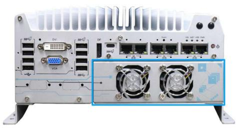
The Cassette module compartmentalizes the heat generated and effectively manages thermal conditions of both the system and graphics card. The modular design reduces the complexity of installing and replacing graphics cards in the fanless controller. In addition, the mechanical design creates a sealed wind tunnel to bring in cold air and expels hot air via system fans to offer the system extreme stability and reliability.
