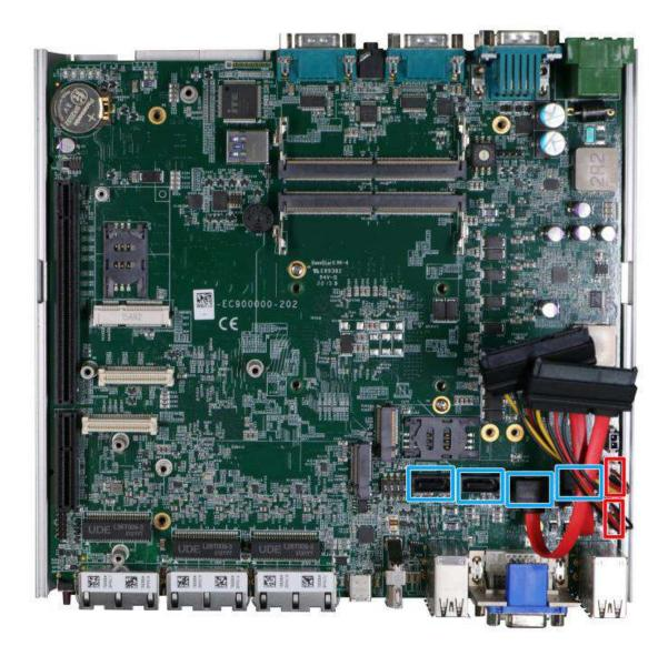
The system has four SATA ports which support Gen3, 6 Gb/s SATA signals. Each SATA port (indicated in **blue**) features a 7-pin SATA connector. However, due to mechanical restrictions, only two SATA ports can be accommodated inside the Nuvo-9000 series.
