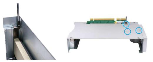
Remove the screws securing the graphics card
