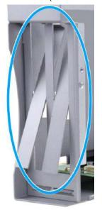
7. Insert and secure the graphics card into the PCIe slot while making sure graphics card's bezel is properly inserted into the notch and the gold fingers are properly inserted.
