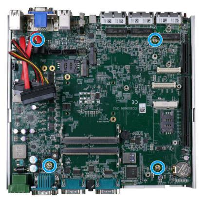
Secure motherboard with four screws
