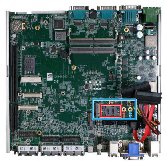
3. Insert the module on a 45 degree angle.
