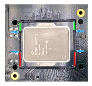
6. Locate the CPU retention bracket (holder) from the accessory box. Place the retention bracket on the CPU and hold it in place. Make sure the indicator triangle engraved on the CPU's integrated heat spreader (HIS) and the triangle indicator on the retention bracket are positioned in the same corner (indicated by blue circles).
