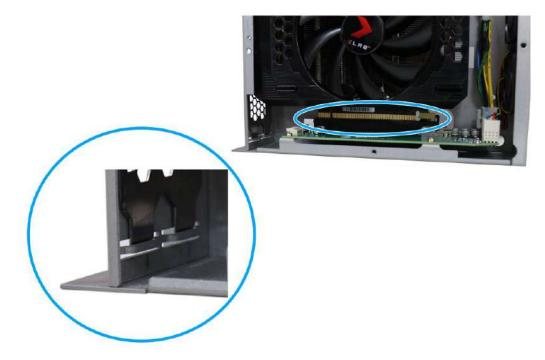
Make sure the card is inserted into the notch and PCIe slot
