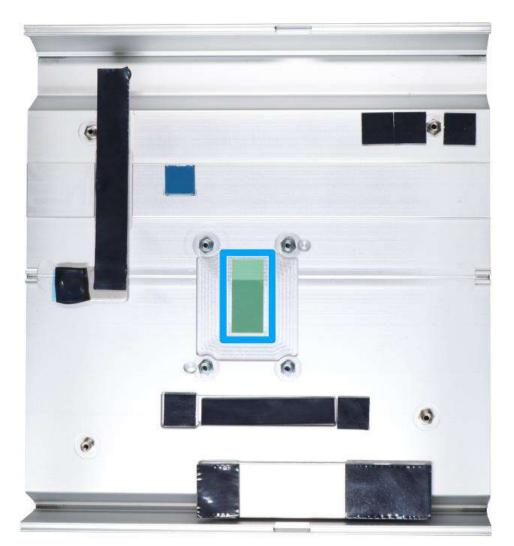
7. Place a new CPU thermal pad (indicated in **blue**) onto the heatsink for the new CPU.
