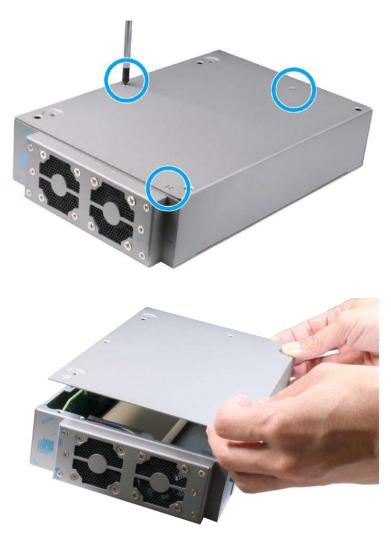
4. If you are replacing the existing graphics card, remove the screws holding the graphics card's I/O panel and remove the three screws holding the duct.
