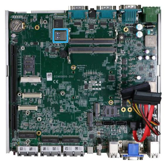
The system's motherboard has an internal USB2.0 port on the PCBA. You can utilize this USB port to connect a USB protection dongle inside the chassis of the system.
