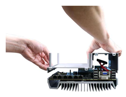
8. Once the bottom panel has been removed, you should have access to the system's internal I/O interfaces.
