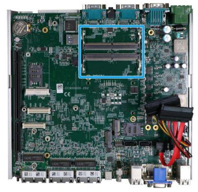
3. To install the memory module, insert gold fingers into the slot at 45-degree angle, push down on the memory module to clip the module into position.
