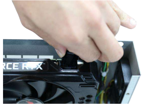
Connect the 8-pin power cable
