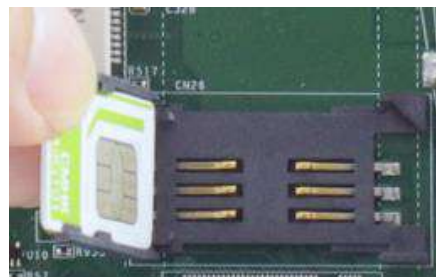
Insert Mini-SIM card with pins facing up
