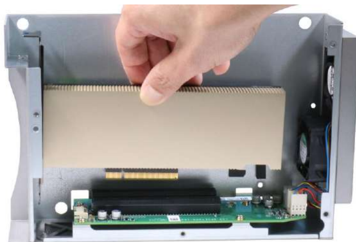
Gently lift the graphics card out of the PCIe slot
