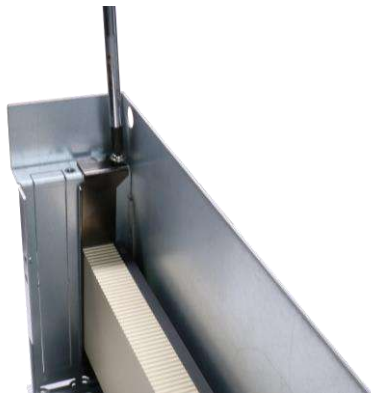
Remove the screws securing the graphics card
