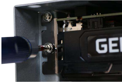
Remove the screws securing the graphics card
