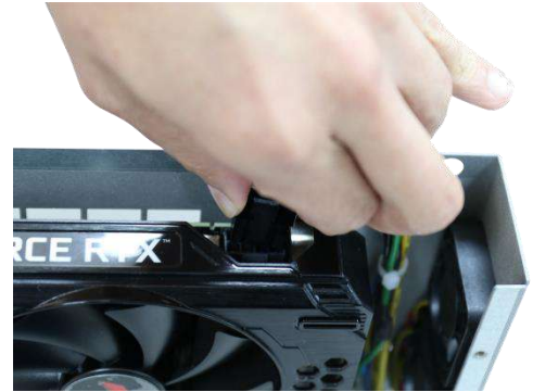
Unplug the 8-pin power cable
