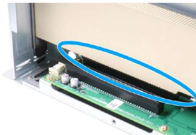
Properly inserted into the PCIe slot
