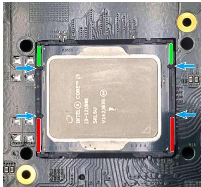
9. Make sure all thermal pad residues have been cleaned on both sides of the retention bracket. Place the CPU retention bracket (holder) on top of the CPU and hold it in place. Make sure the indicator triangle engraved on the CPU's integrated heat spreader (HIS) and the triangle indicator on the retention bracket are positioned in the same corner (indicated by **blue circles**).
