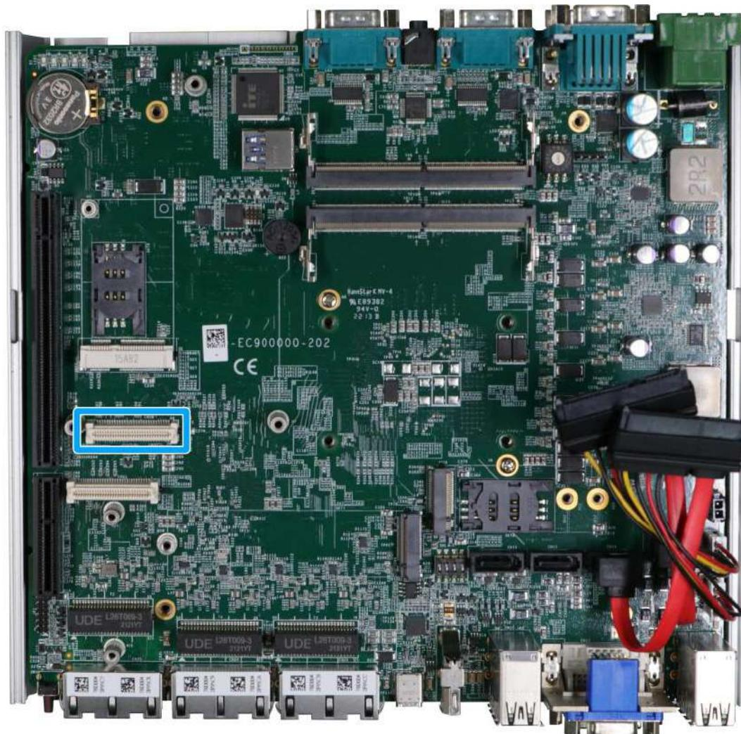
MezIO™ is an innovative interface designed for integrating application-oriented I/O functions into an embedded system. It offers computer signals, power rails and control signals via a high-speed connector. MezIO™ is also mechanically reliable benefited from its 3-point mounted mezzanine structure. A MezIO™ module can leverage these signals to implement comprehensive I/O functions.
