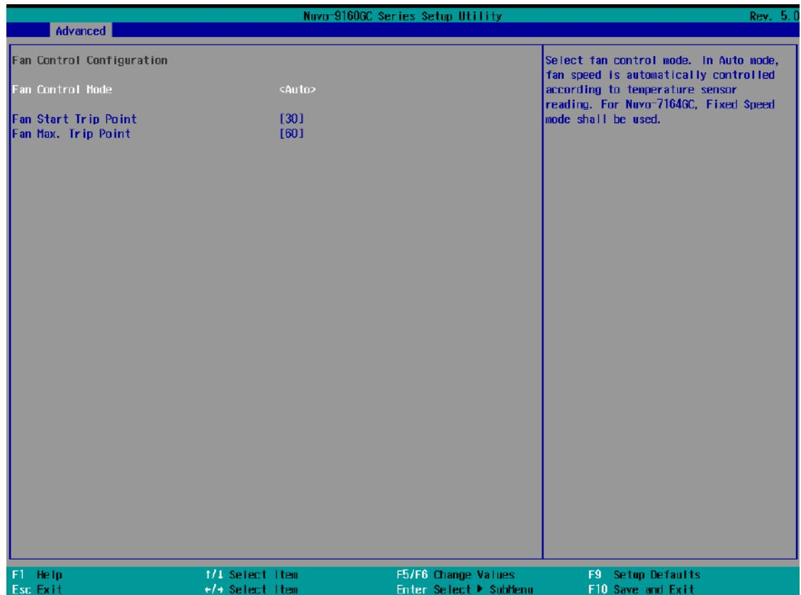
4. Use the up/ down arrow keys to highlight Fan Start Trip Point or Fan Max. Trip Point and press ENTER, a window appears and you may enter the temperature in degree Celsius.
