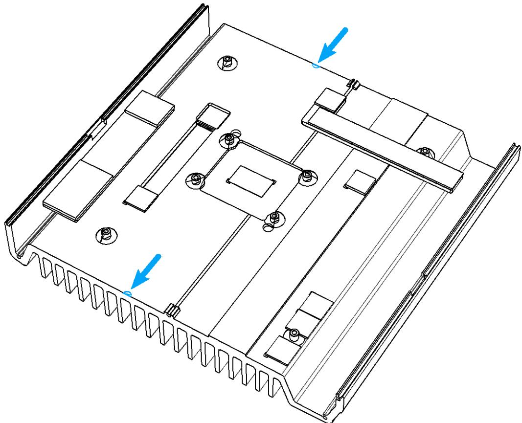
11. Place the washers onto the four screw holes for spring-screws to secure the CPU socket to the heatsink.
