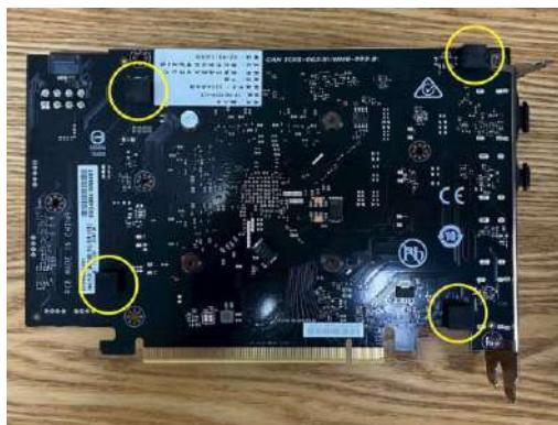
For Gigabyte RTX 4060, stick four 8 x 8 x 6 mm rubber cubes onto the back of the graphics card
