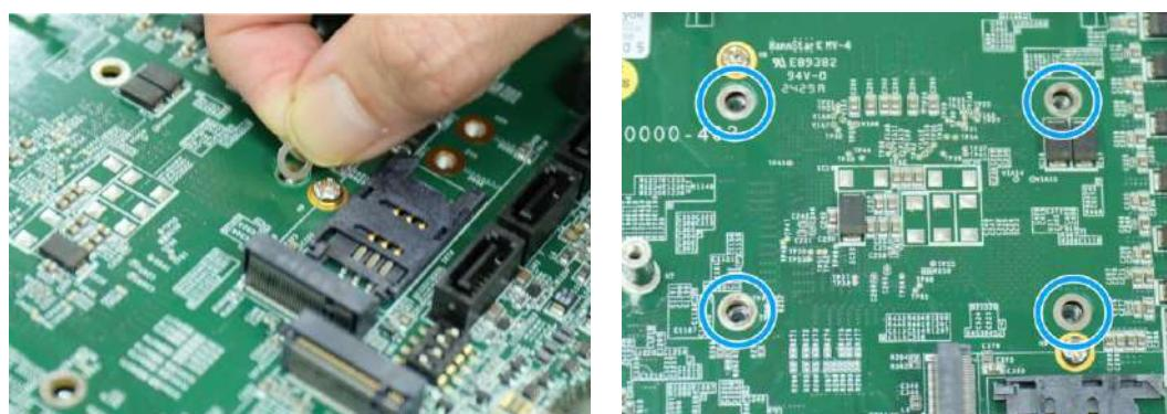
14. Once the motherboard has been installed, you're ready to secure the four screws that help the heatsink apply pressure to the CPU/ chipset die. You'll want to apply even pressure to the corners by gradually tightening each screw. Please refer to the recommended order when tightening the screws.
