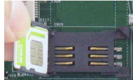
Insert Mini-SIM card with pins
