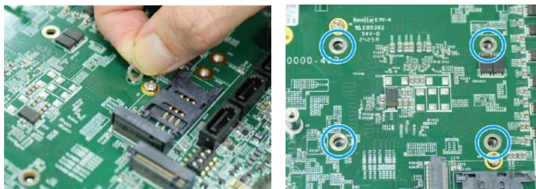
12. Once the motherboard has been installed, you're ready to secure the four screws that help the heatsink apply pressure to the CPU/ chipset die. You'll want to apply even pressure to the corners by gradually tightening each screw. Please refer to the recommended order when tightening the screws.
