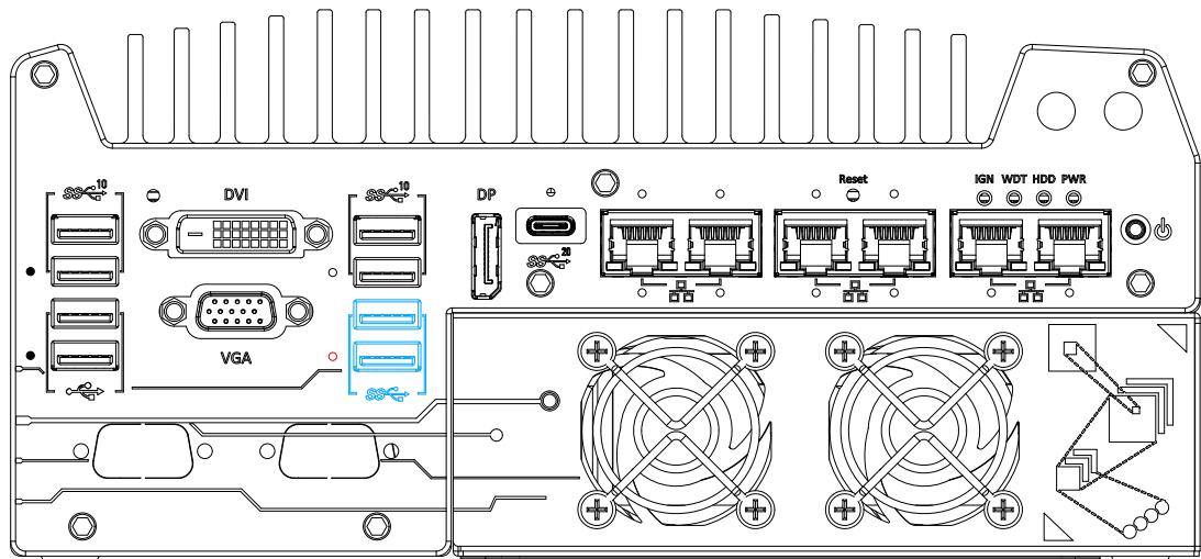
The system's USB 3.2 Gen1x1 ports (5Gbps) are implemented via native xHCI (eXtensible Host Controller Interface) controller and are backward compatible with USB 2.0, USB 1.1 and USB 1.0 devices. UEFI USB is also supported so you can use USB keyboard/mouse in UEFI shell environment. Indicated in red is a screw-lock hole for the corresponding USB port. xHCI driver is supported natively in Windows 10, therefore you do not need to install the xHCI driver prior to utilizing USB functions.
