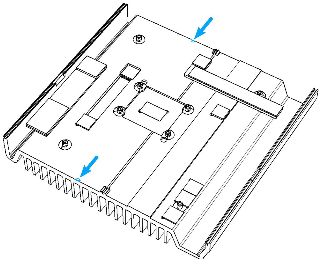
13. Place the washers onto the four screw holes for spring-screws to secure the CPU socket to the heatsink.
