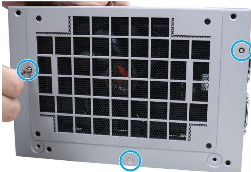
9. Gently lower the Cassette module back onto the system enclosure and secure the module onto the system enclosure by securing the following screws.
