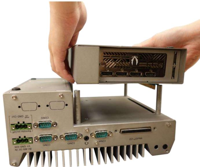
14. Secure the module onto the system enclosure by securing the following screws.
