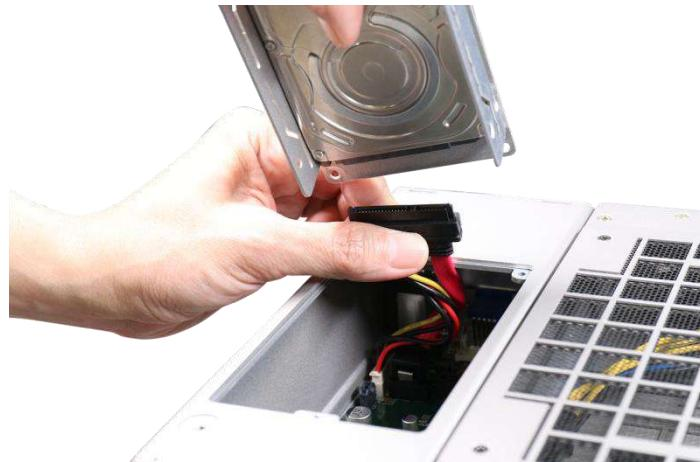
6. Gently put the tray back into the system with the connector side being inserted into the system first and secure the tray with three screws.
