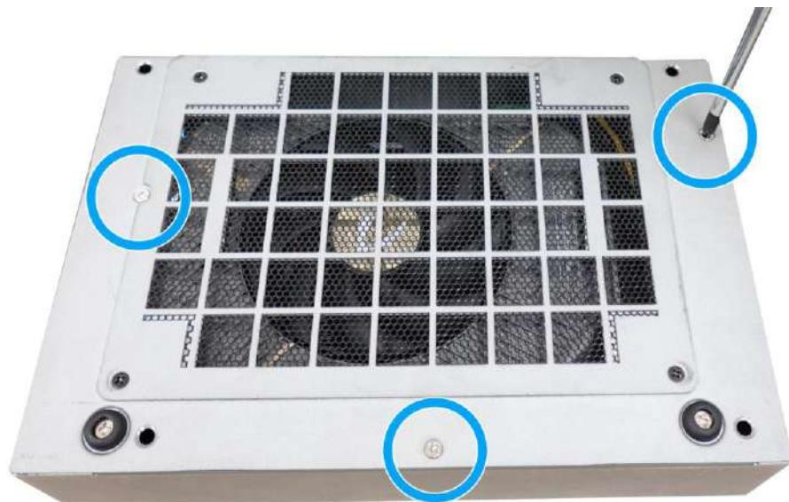
13. Gently lower the Cassette module back onto the system enclosure.
