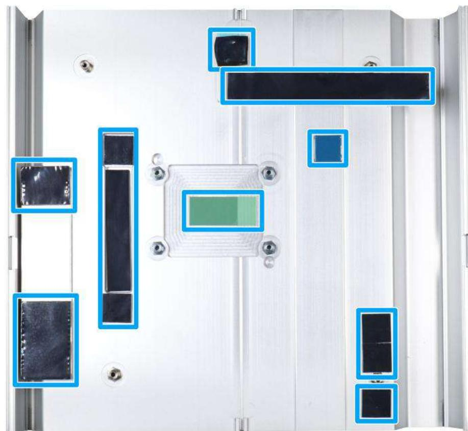
9. With the four motherboard standoffs aligned, gently lower the motherboard onto the heatsink and secure the four screws. Please remember to remove the protective film (indicated in red) on the CPU's thermal pad as well.
