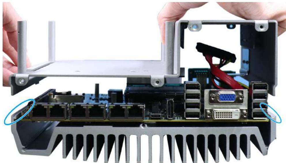
2. Install the front panel and secure screws indicated in **blue**.
