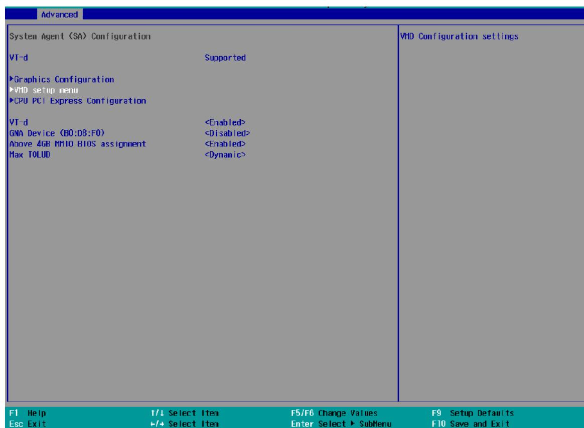
3. Highlight **[Enable VMD controller]**, press ENTER to bring up Options, Enabled/ Disabled, select Enabled and press ENTER.
