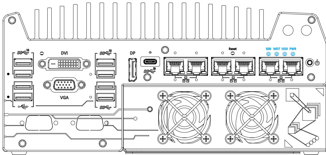
There are four LED indicators on the I/O panel: IGN, WDT, HDD and PWR. The descriptions of these four LED are listed in the following table.
