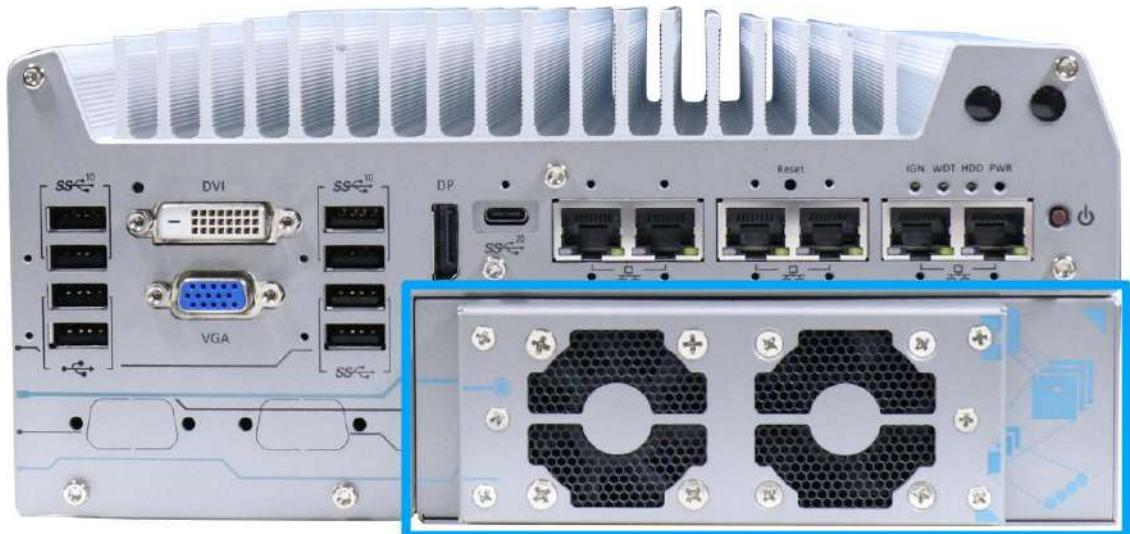
The Cassette module compartmentalizes the heat generated and effectively manages thermal conditions of both the system and graphics card. The modular design reduces the complexity of installing and replacing graphics cards in the fanless controller. In addition, the mechanical design creates a sealed wind tunnel to bring in cold air and expels hot air via system fans to offer the system extreme stability and reliability.
