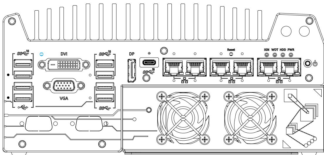
The CMOS Reset button is used to manually reset the motherboard BIOS in case of system halt or malfunction. To avoid unexpected operation, it is purposely placed behind the panel. To reset, disconnect the DC power input, and use the tip of a pen to press and hold for at least 5 seconds to reset the BIOS.
