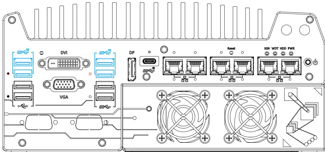
The system's USB 3.2 Gen2x1 ports (10Gbps) are implemented via native xHCI (eXtensible Host Controller Interface) controller and are backward compatible with USB3.2 Gen.1 USB 2.0, USB 1.1 and USB 1.0 devices. UEFI USB is also supported so you can use USB keyboard/mouse in UEFI shell environment. Indicated in red are screw-lock holes for the corresponding USB port.
