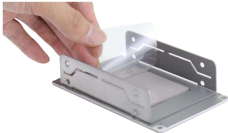
4. Place the HDD/ SSD (with labels facing up), match the SATA connector end to the side with two screw holes (indicated in blue), secure the HDD/ SSD with the supplied flathead screws (4 per drive).
