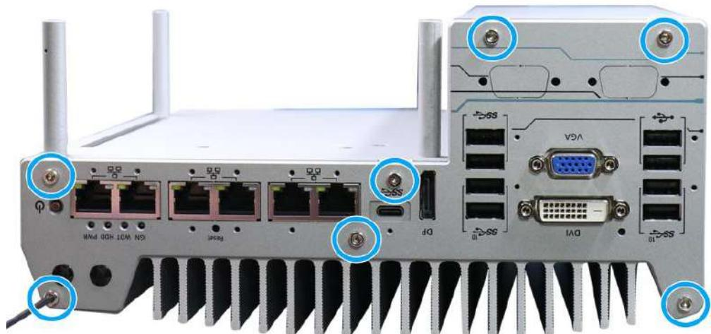
3. Install the rear panel and secure screws indicated in **blue**.
