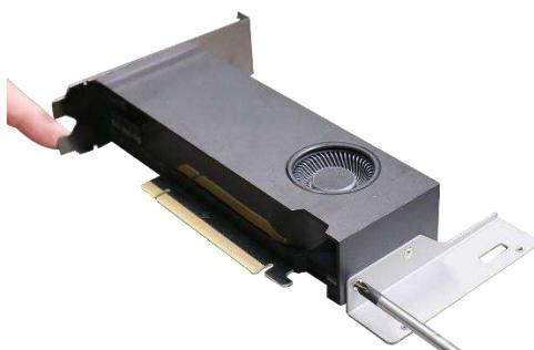
For NVIDIA A2000, 2000 ADA or SFF 4000 ADA, secure the dedicated bracket onto the card's heat spreader cover.
