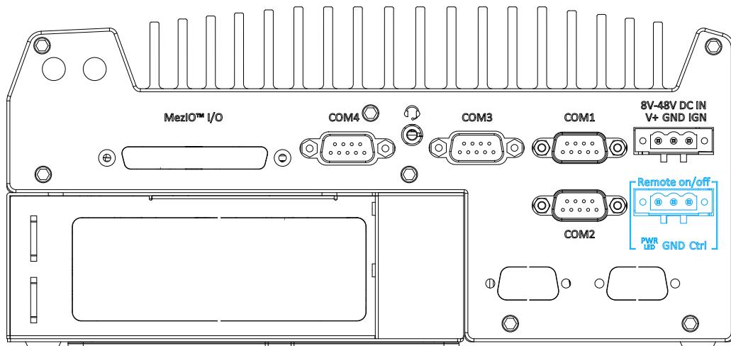
The “Remote On/ Off” 3-pin connection allows for the connection of an external non-latched switch to turn on/ off the system. It is useful when the system is placed in a cabinet or a not easily accessed location. You may connect an external status LED (20mA) indicator by connecting to PWR LED and GND.
