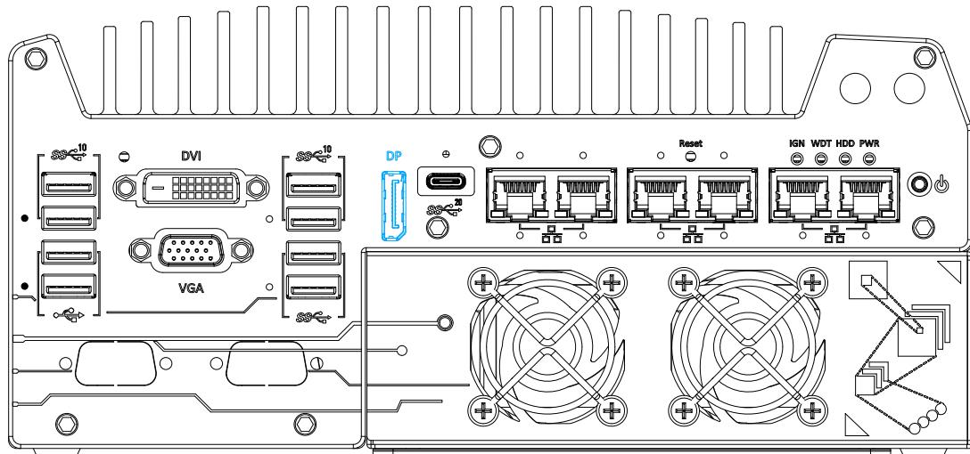
The system has a DisplayPort (DP) output which is a digital display interface that mainly connect video source and carry audio to a display device. When connecting a DP, it can deliver up to 4K UHD (4096 x 2304 @ 60Hz) in resolution. The system is designed to support passive DP adapter/ cable. You can connect to other display devices using DP-to-HDMI cable or DP-to-DVI cable.
