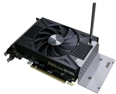
For Leadtek WinFast RTX 4060 graphics card, secure the dedicated bracket onto the card's heat spreader cover
