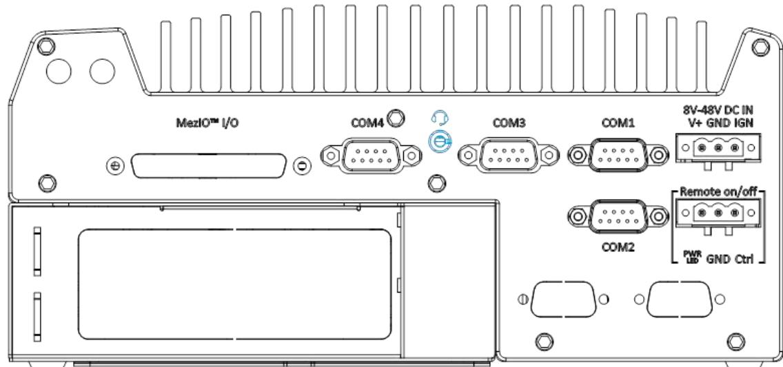
The system audio function uses high definition audio. There is a female 4-pole
