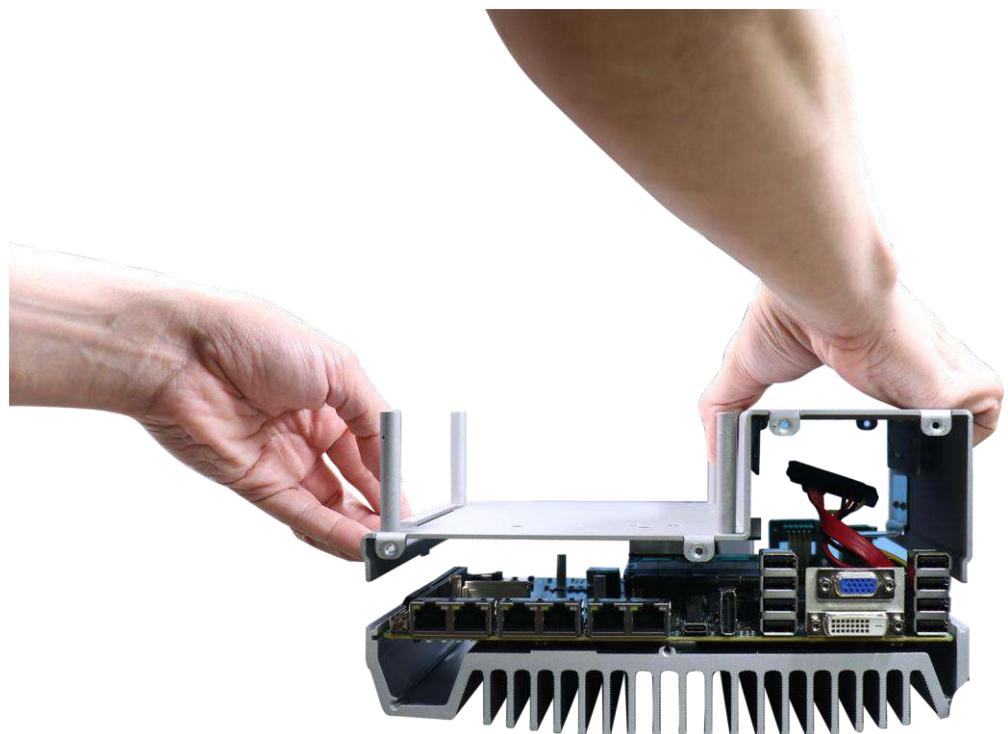
8. Once the bottom panel has been removed, you should have access to the system's internal I/O interfaces.
