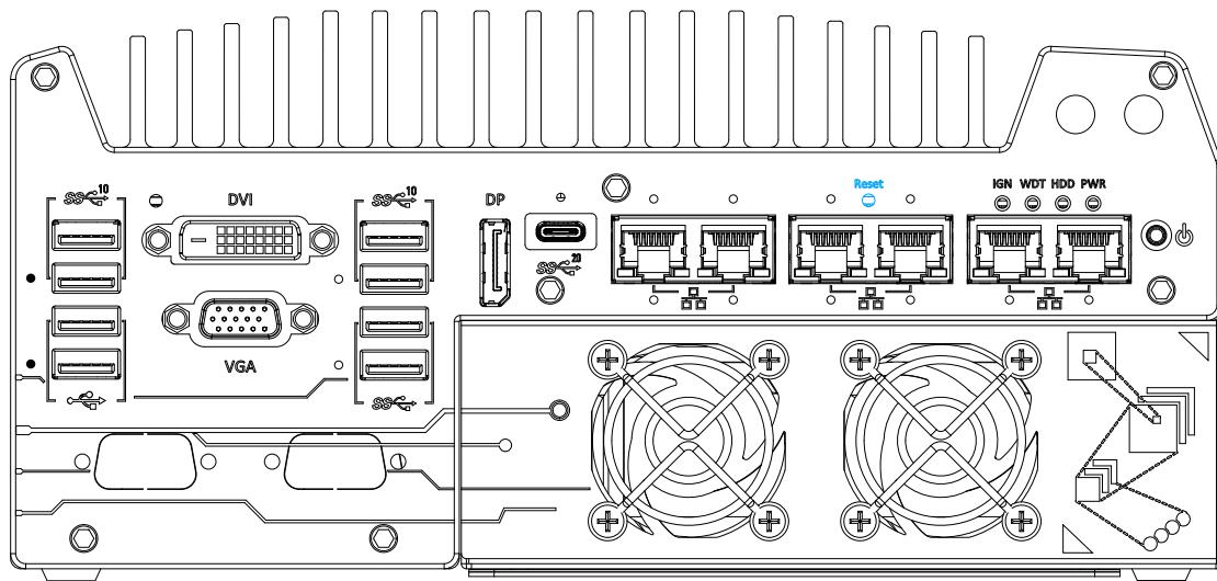
The reset button is used to manually reset the system in case of system halt or malfunction. To avoid unexpected reset, the button is purposely placed behind the panel. To reset, please use a pin-like object (eg. tip of a pen) to access the reset button
