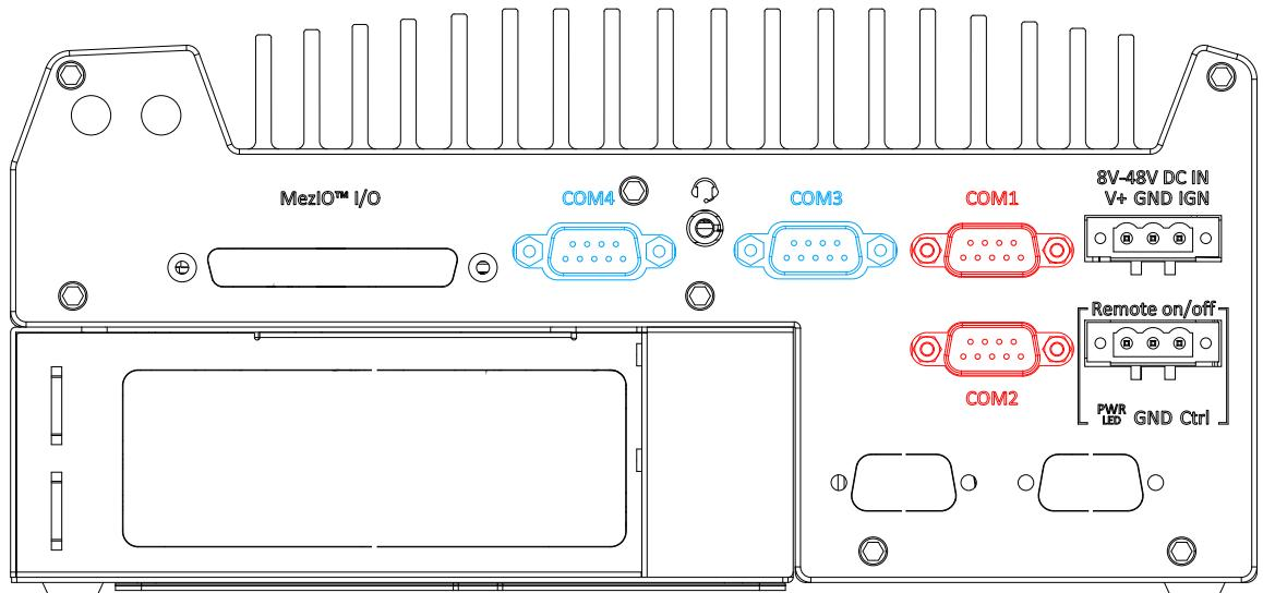
The system provides four COM ports for communicating with external devices. These COM ports are implemented using industrial-grade ITE8786 Super IO chip (-40 to 85°C) and provide up to 115200 bps baud rate.
