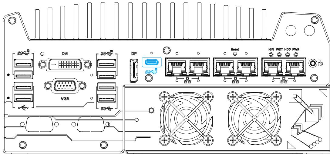
The system's USB 3.2 Gen2x2 type-C port offers up to 20Gbps of data transfer bandwidth, and is implemented via the native xHCI (eXtensible Host Controller Interface) controller. The port is backward compatible with USB3.2 Gen.1 USB 2.0, USB 1.1 and USB 1.0 devices via a USB hub (not included) to connect to external devices.
