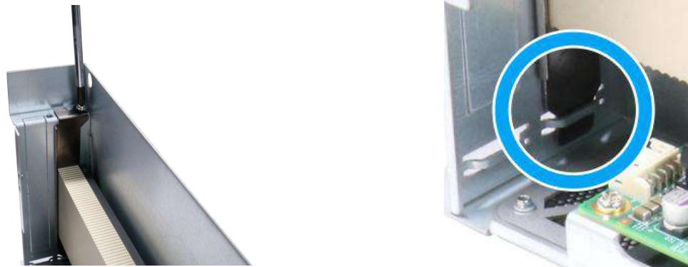
**Insert and secure graphics card into PCIe slot    Bezel inserted into the notch**
