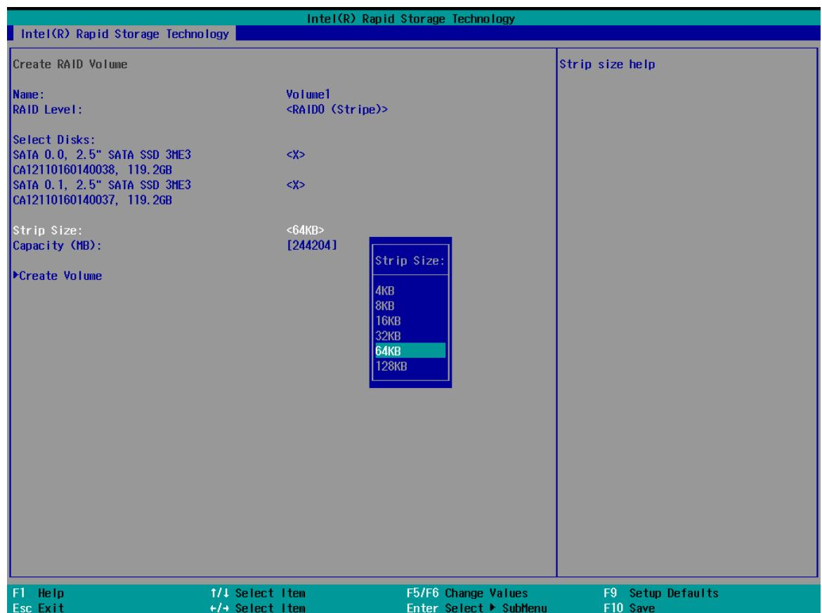
7. The Capacity (MB) option allows you to configure the storage capacity of your RAID volume. By default, the full storage capacity will be applied. Once you have entered a capacity, press ENTER to confirm.
