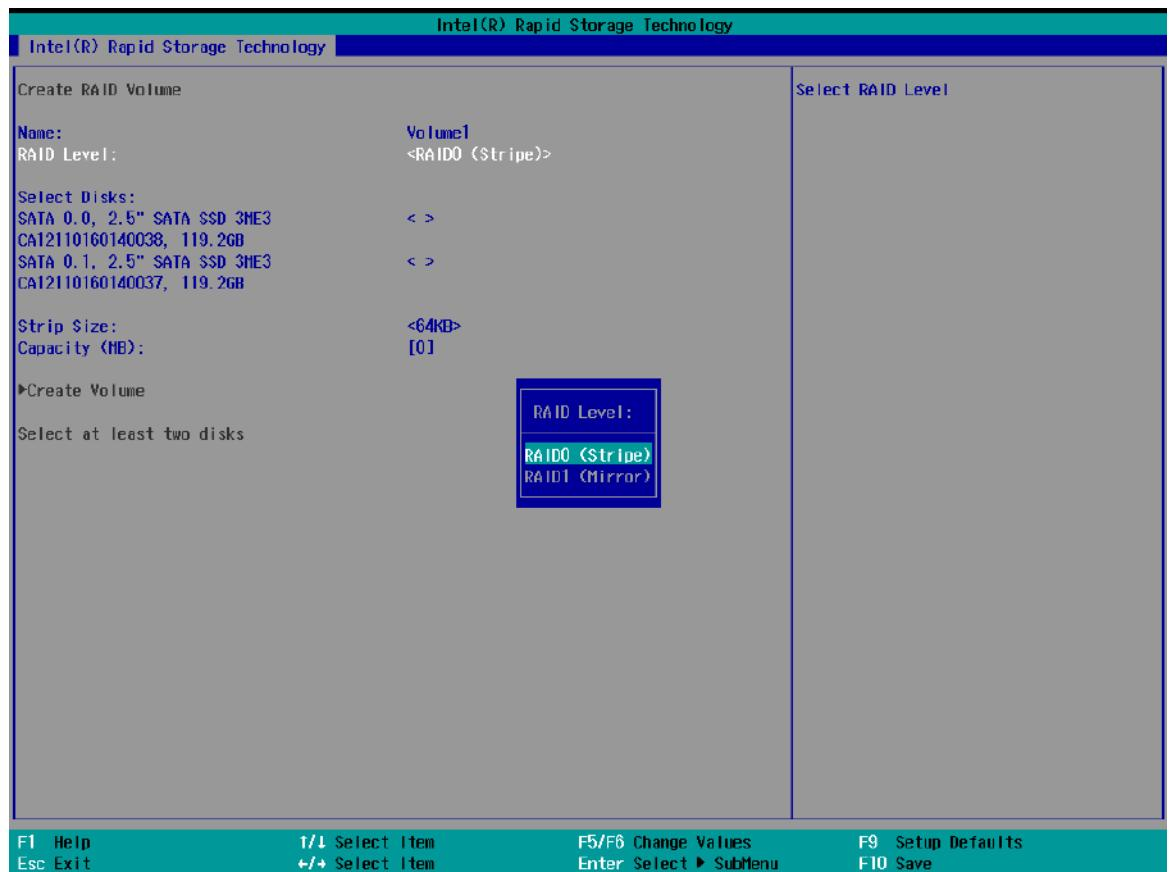
5. The Select Disks option allows you to select disk drives for your RAID volume. Highlight a drive and press ENTER, use up/ down arrow keys to highlight “x” and press ENTER to confirm the selection. A minimum of two disk drives must be selected for RAID-0 or RAID-1 configuration. Press ENTER when ready.
