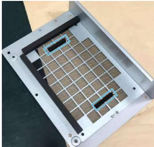
For MSI RTX 3050, PNY RTX 3050, and Gigabyte RTX 4060 graphics cards, stick two 36 x 6 x 6mm Porons onto the Cassette module cover
