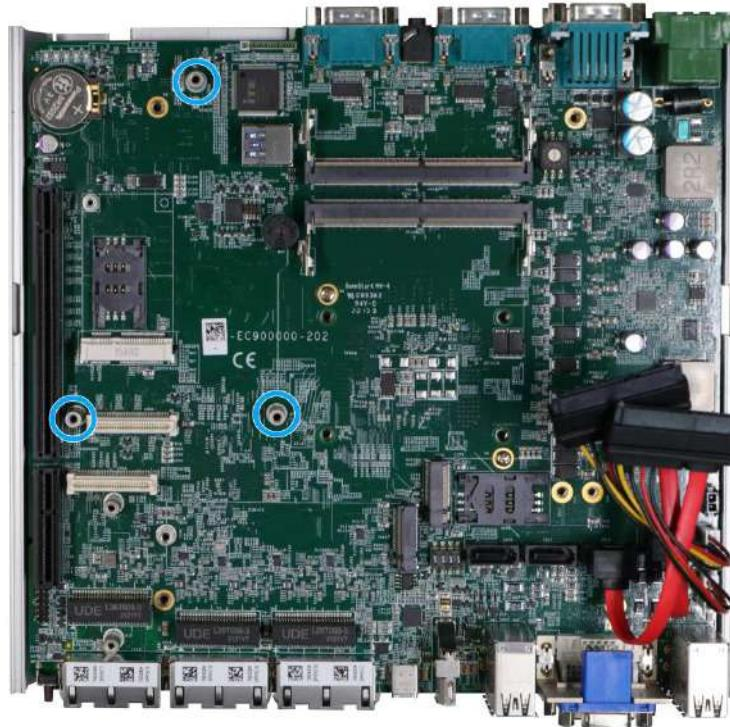
3. Gently lower the MezIO™ module onto the three stand-mounts while matching the MezIO™ interface. Secure the module using three screws supplied.
