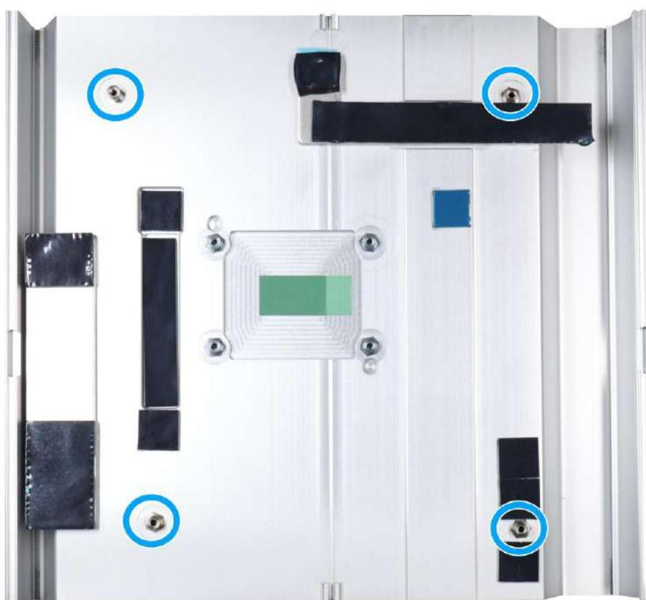
12. Note if there are **grooves** on the heatsink, skip the next step and go to step 14. If your heatsink does not have the grooves, please continue onto the following step.
