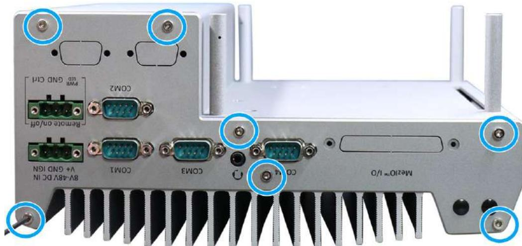
4. Gently lower the Cassette module back onto the enclosure and secure it with screws (indicated in **blue**).
