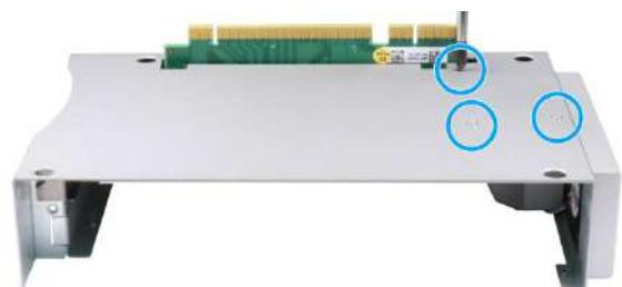
**Remove the screws securing
