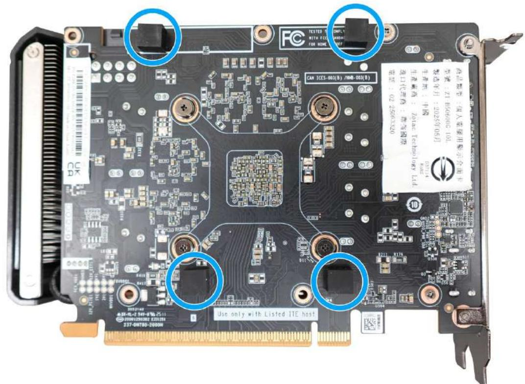
7. If you are installing the graphics card for the first time, remove the bezel cover (indicated in **blue circle**).
