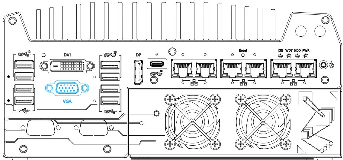
VGA connector is the most common video display connection. The VGA output supports up to 1920x1200@60Hz resolution.
