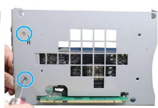
Secure NVIDIA A2000, 2000 ADA, and SFF 4000 ADA graphics card's backplate to the Cassette module enclosure
