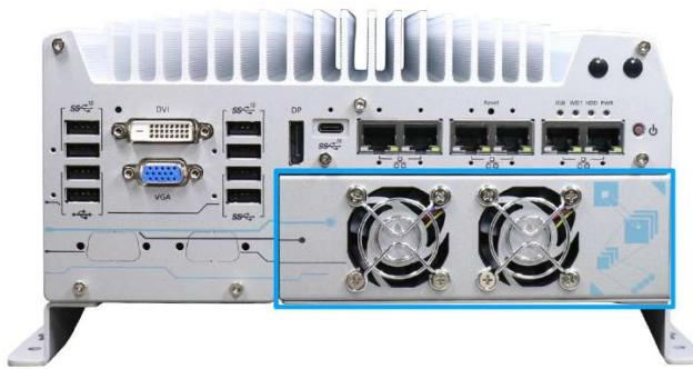
The Cassette module compartmentalizes the heat generated and effectively manages thermal conditions of both the system and graphics card. The modular design reduces the complexity of installing and replacing graphics cards in the fanless controller. In addition, the
