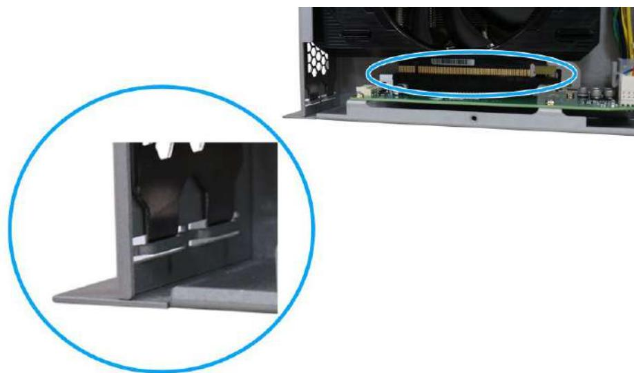
10. Secure the graphics card with screws and connect the 8-pin power cable.
