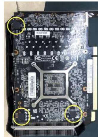
For PNY RTX 3050 graphics card, stick three 8 x 8 x 6mm rubber cubes onto the back of the graphics card
