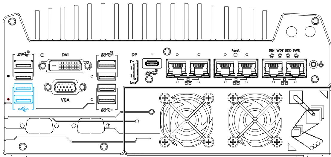
The USB2.0 ports are implemented via native xHCI (eXtensible Host Controller Interface) and are backward compatible with USB 1.1 and USB 1.0 devices. UEFI USB support is also provided so you can use USB keyboard/ mouse in UEFI shell environment. Indicated in red is a screw-lock hole for the corresponding USB port.
