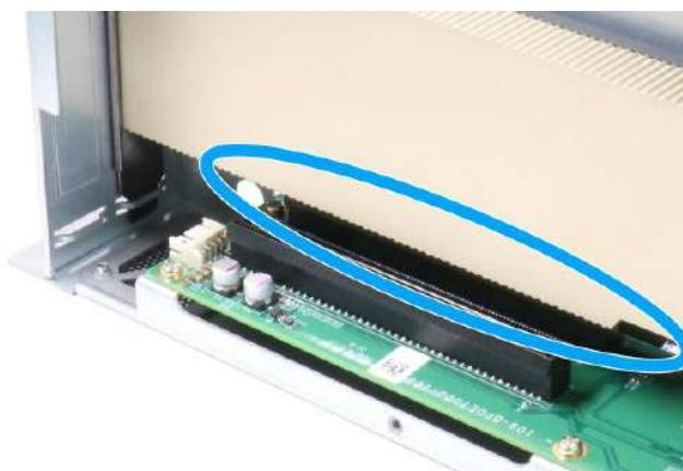
**Properly inserted into the PCIe slot**
