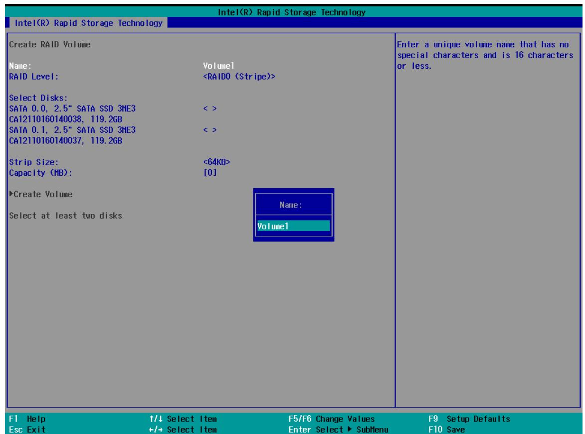
4. The RAID Level option allows you to select RAID-0 (stripping) or RAID-1 (mirror) for your RAID volume. Press ENTER when ready.
