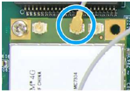
Clip on IPEX-to-SMA cable
