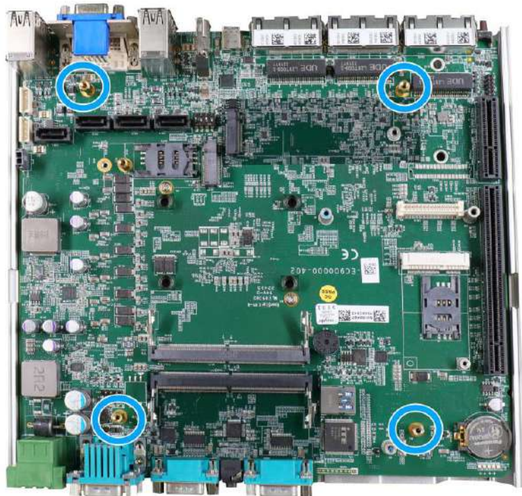
Secure motherboard with four screws
