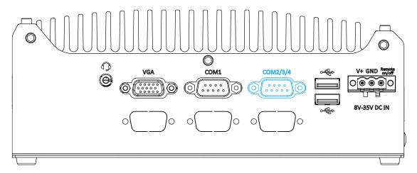
Implemented using industrial-grade ITE8786 Super IO chip (-40 to 85°C) and provide up to 921600 bps baud rate, the D-Sub male connector (COM2/ 3/ 4) can be configured in the BIOS as single RS-422/ 485 port (COM2) or three 3-wire RS-232 ports (COM2/COM3/COM4). Please refer to COM2/ 3/ 4 Port Configuration for configuring operation mode. An optional 1-to-3 Y-cable is available to connect three RS-232 devices.
