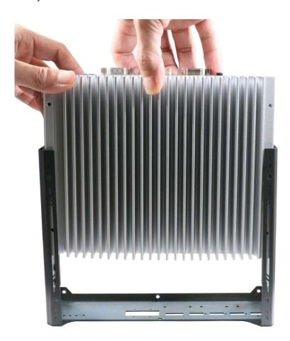
2. Secure the heatsink onto enclosure by securing screws indicated on the heatsink.
