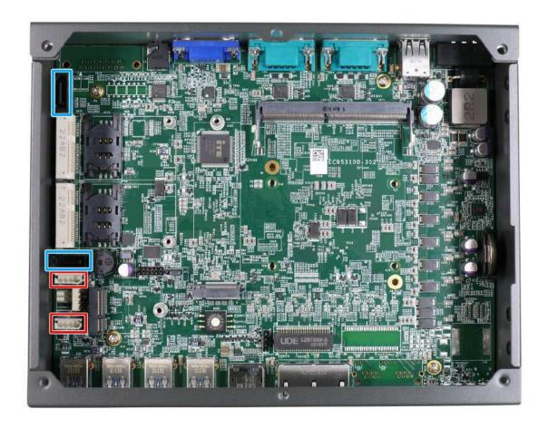
The system provides two SATA ports which support Gen3, 6 Gb/s SATA signals. The SATA port is composed of a 7-pin SATA connector (indicated in **blue**) and a 4-pin power connector (indicated in **red**). A dedicated cable is shipped with the system to provide a standard 22-pin SATA connector to the installed device.
