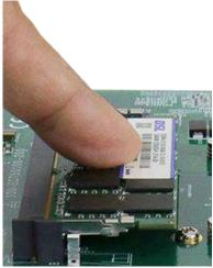
Insert module into slot
