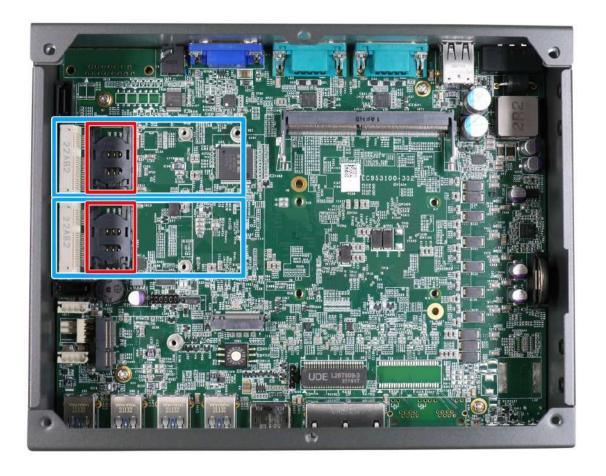
The system provides a mini-PCle socket (indicated in **blue**) that is in compliance with mini-PCle specification rev. 1.2. This mini-PCle socket is designed with SIM card (slot indicated in **red**) support. With a SIM card installed, your system can access the internet via your network provider's 4G/3G network.
