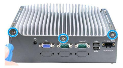
5. Place the four rubber stand and secure the four (4) screws at the bottom of the system panel.
