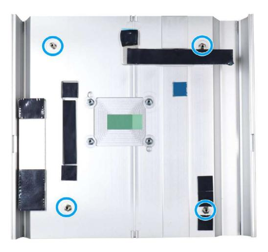
12. Secure the four (4) M3 P-head motherboard screws (indicated in blue).
