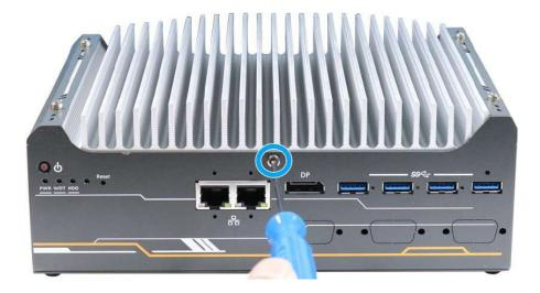
4. Attach the VGA/ COM/ 3-pin panel and secure with the screws indicated.
