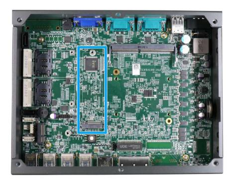
4. Insert the module on a 45 degree angle.
