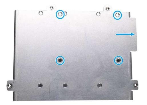
6. Secure 2.5" HDD/ SSD on the HDD/SSD bracket with 4 M3 flat-head screws.
