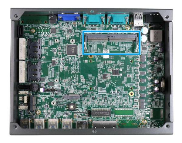
The system motherboard supports one 260-pin SODIMM socket for installing one DDR4-3200 memory module up to 32GB capacity.
