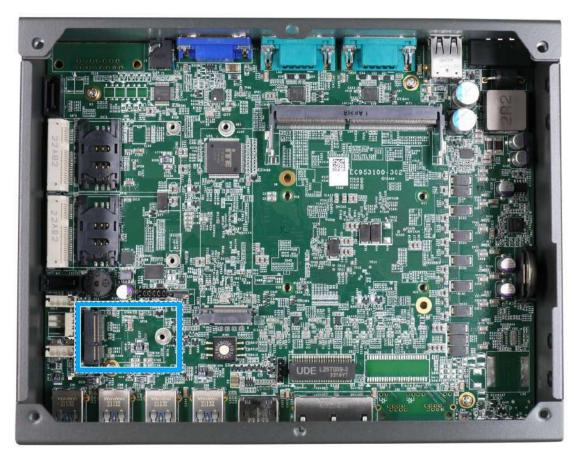
The system has an M.2 2230 E key socket that offers PCIe Gen3 x1 and USB2.0 signal for WiFi 5/ 6 or Google TPU module installation.
