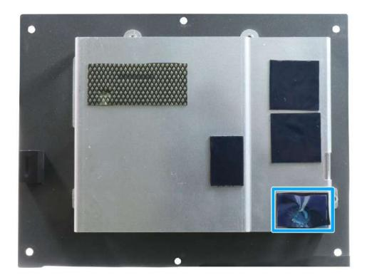
8. Reinstall the system enclosure, panel and attach the external antenna.
