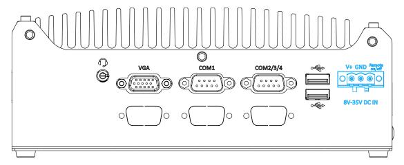
The system accepts a wide range of DC power input from 8 to 35V via a 3-pin pluggable terminal block, which is fit for field usage where DC power is usually provided. The screw clamping mechanism on the terminal block offers connection reliability when wiring DC power. The Remote On/ Off connection allows for external switch extension. It is useful when the system is placed in a cabinet or a not easily accessed location.
