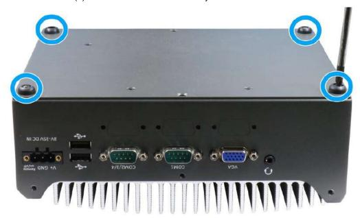
2. Gently lift and remove the bottom panel to access to internal expansion slots.
