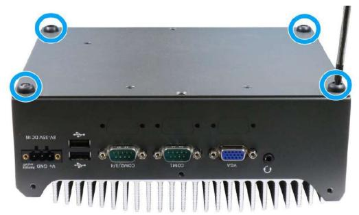
2. Gently lift and remove the bottom panel to access to memory slot.
