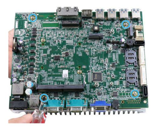
Use the four (4) M3 spring screws (indicated in blue) to secure the CPU area to the heatsink. Gradually tighten the four spring-screws in the following order for even pressure.
