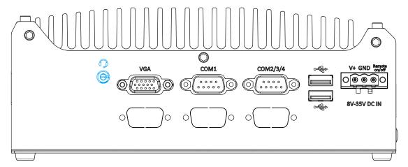
There is a female 4-pole audio jack for headphone (speaker) output and microphone input. To utilize the audio function in Windows, you need to install corresponding drivers. Please refer to the section, <u>Driver Installation</u>.
