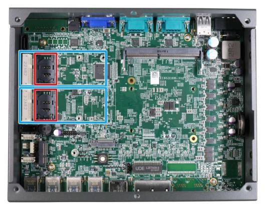
4. Before installing the mPCIe module, you need to insert the Mini-SIM card. Slide the SIM slot holder and lift the SIM card holder. Insert the Mini-SIM card (pins facing towards the motherboard), shut the SIM holder and slide it to lock the SIM card in-place.
