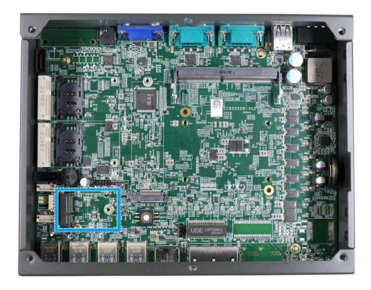
4. Insert the M.2 module on a 45 degree angle into the M.2 slot, and secure with a screw.
