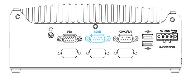
Implemented using industrial-grade ITE8786 Super IO chip (-40 to 85°C) and provide up to 921600 bps baud rate, COM1 is a software-configurable RS-232/422/485 port via 9-pin D-Sub male connector. The operation mode, slew rate and termination of COM1 can be set in BIOS setup utility. The following table describes the pin definition of COM ports.
