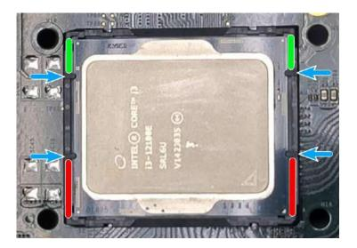
5. Locate the CPU retention bracket (holder) from the accessory box. Place the retention bracket on the CPU and hold it in place. Make sure the indicator triangle engraved on the CPU's integrated heat spreader (HIS) and the triangle indicator on the retention bracket are positioned in the same corner (indicated by blue circles).
