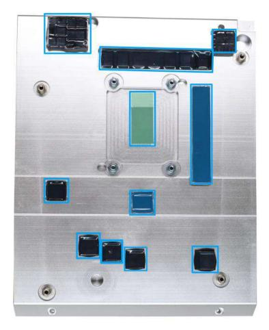
8. With the four motherboard standoffs aligned, gently lower the motherboard onto the heatsink and secure the four screws. Please remember to remove the protective film (indicated in red) on the CPU's thermal pad as well.
