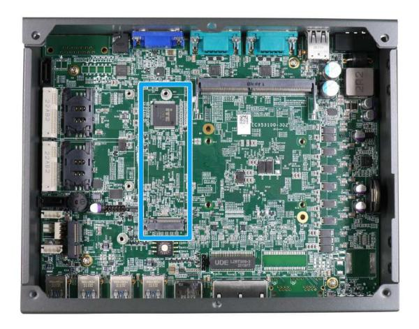
The system has a Gen4 x4 PCIe M.2 2280 slot for you to install an NVMe SSD. The M.2 NVMe SSD offers significantly better system performances when compared to a 2.5" SSD.
