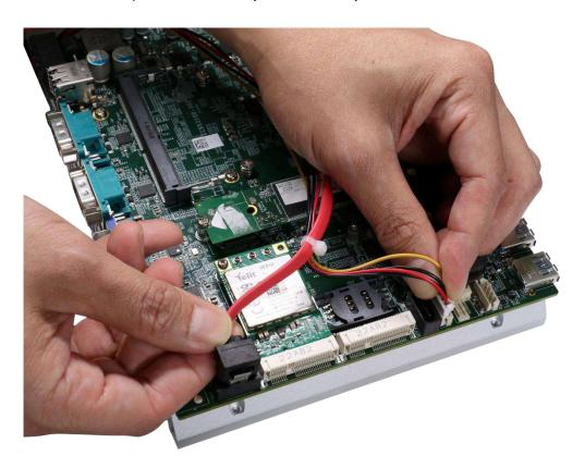
16. Re-secure the hard drive cage onto the bottom panel.
