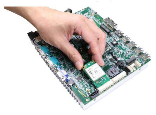
6. Gently press down and secure the module with two M2.5 P-head screws
