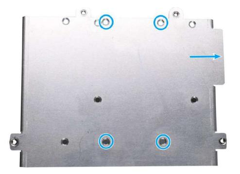
14. Secure 3.5" HDD on the HDD/SSD bracket with 4 M3 flat-head screws.
