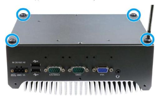
Gently lift and remove the bottom panel to access the hard drive cage and SATA/ power connectors on the motherboard.
