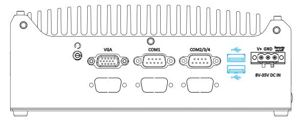
The USB2.0 ports are implemented via native xHCI (eXtensible Host Controller Interface) in the Intel 600 chipset and are backward compatible with USB 1.1 and USB 1.0 devices. UEFI USB support is also provided so you can use USB keyboard/mouse in UEFI shell environment. xHCI driver is supported natively in Windows 10, therefore you do not need to install xHCI driver to utilize USB functions.
