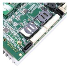
Insert SIM with pins facing the motherboard
