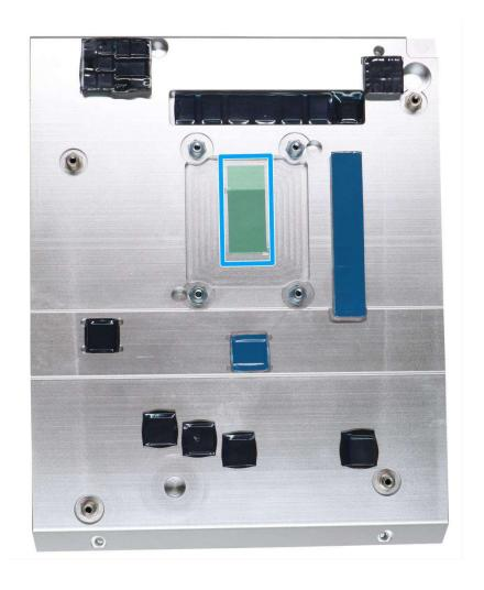
Remove and clean off any thermal pad residues around the socket/
