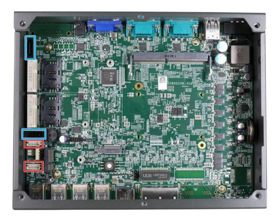
4. The hard drive installation cage is secured onto the bottom panel of the system. Separate the cage from the panel by removing the screws indicated in blue.
