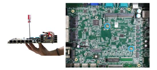
Hold CPU bracket firmly and turn the motherboard around
