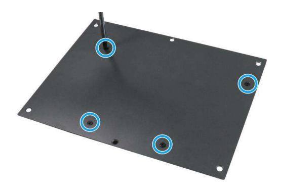
5. The screw holes to secure the 2.5" HDD/ SSD are indicated by blue circles. Please note the hard drive installation orientation by making sure the SATA connector is in the same direction as the blue arrow.
