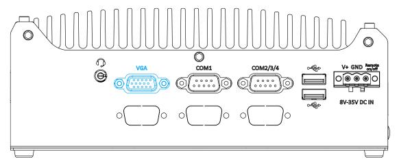
VGA connector is the most popular way for connecting a display. The VGA output on Nuvo-9501 series supports up to 1920 x 1200 resolution. To support multiple display outputs and achieve best VGA/ DP output resolution in Windows, you need to install corresponding graphics driver. Please refer to the driver installation section.
