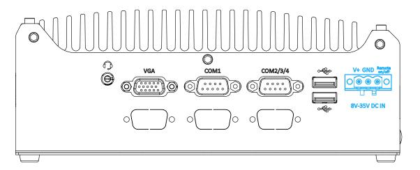
2. Simply short the V+ pin and the Remote on/off pin, and power-on the system to activate the Always On function.
