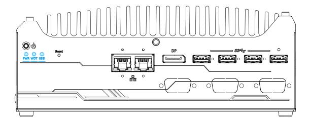
There are three LED indicators on the I/O panel: PWR, WDT and HDD. The descriptions of these three LED are listed in the following table.
