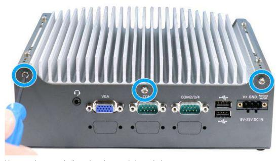
2. Unscrew the screw indicated on the panel shown below.
