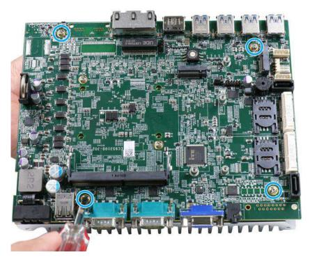
12. Once the motherboard has been installed, you're ready to secure the four screws that help the heatsink apply pressure to the CPU/ chipset die. You'll want to apply even pressure to the corners by gradually tightening each screw. Please refer to the recommended order when tightening the screws.
