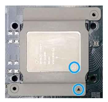
Turn the motherboard around and secure the bracket by tightening two M3
