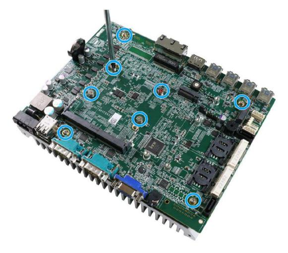
4. Remove the screws indicated once you separate the heatsink from the motherboard to remove the CPU holder.
