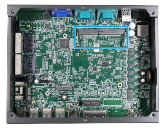
4. To install the memory module, insert gold fingers of the module into the slot at 45 degree angle, push down on the edge of the module and the clips on the side should clip the module into position.
