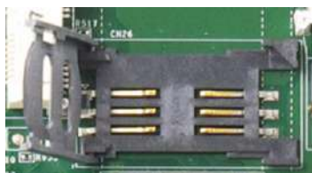
Slide and lift SIM card holder
