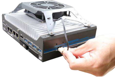
Locate 4-pin power plug location
