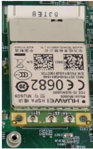
Insert on 45 degree angle
