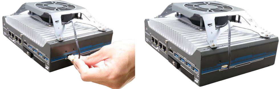
Locate 4-pin power plug location
