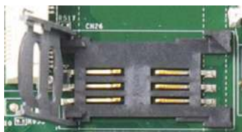
Slide and lift SIM card holder
