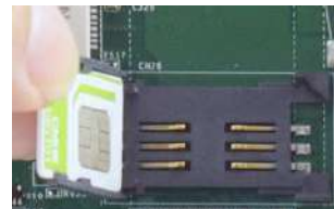
Insert SIM card with pins facing up
