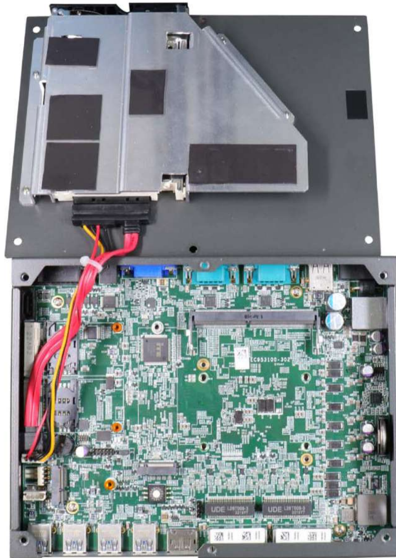
SATA/ power cables connected
