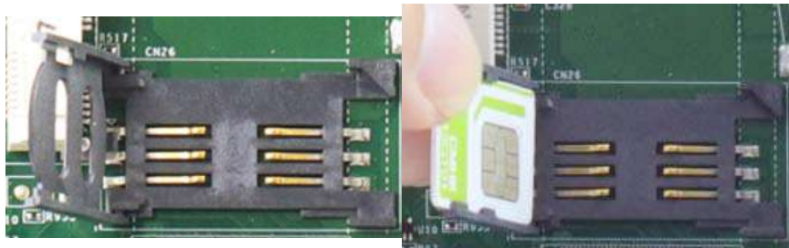
Slide and lift SIM card holder
