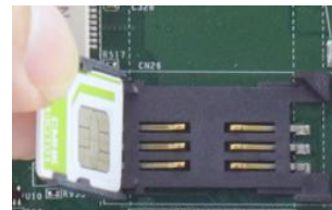
Insert SIM card with pins facing up
