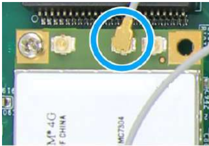
Clip on IPEX-to-SMA cable
