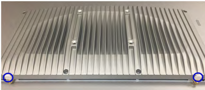
Figure 2.16 Removing plugs for the antennae
