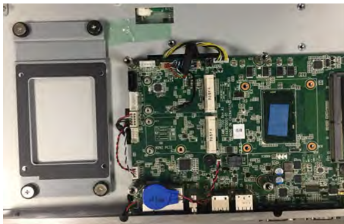
Figure 2.7 Retention screws on HDD bracket
