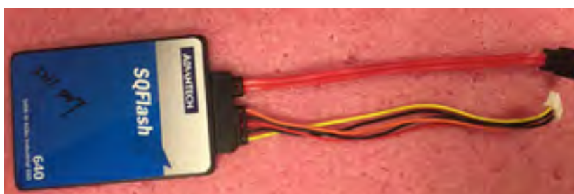
Figure 2.9 SATA cable connected to SATA HDD
