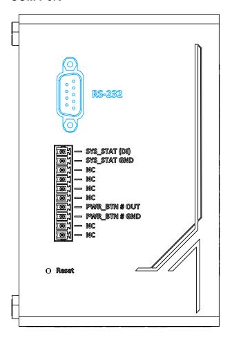
The 9-pin D-sub COM port can connect and communicate with the host computer to acquire PB-9250J/ 4600J information.
