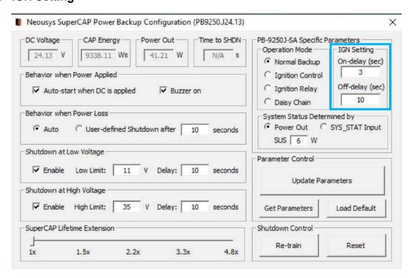
If PB-9250J/ 4600J is in Ignition Control Mode, user can set IGN on/off delay via IGN setting.
