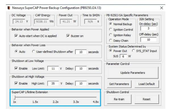
The SuperCAP lifetime extension setting is an automated setting when users only need to click on the bar, drag it to the desired lifetime extension setting, click on the "Update Parameters" and follow procedure instructions for settings to take effect.
