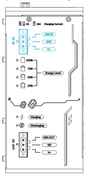
The system accepts a wide range of DC power input from 12 to 35V via a 3-pin pluggable terminal block, which is fit for field usage where DC power is usually provided. The screw clamping mechanism on the terminal block offers connection reliability when wiring DC power. In addition to DC power input, this terminal block can also accept ignition signal input (IGN) when PB-9250J/ 4600J is configured in Ignition Control Mode/ Ignition Relay Mode for in-vehicle applications.
