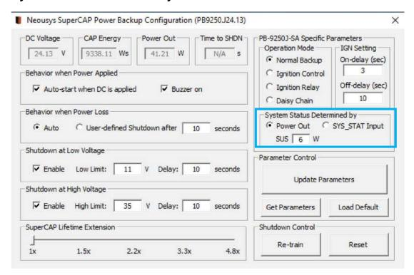
PB-9250J/ 4600J has to monitor back-end system status (whether it's on or off) in order to make the right operation in different situation.
