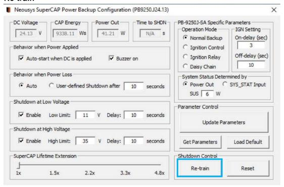
The Re-train function is to customize the PB-9250J/ 4600J to your system's required shutdown time! By clicking on "Re-train", a shutdown action will be initiated so the time required to shutdown can be memorized.
