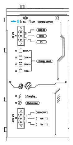
PB-9250J/ 4600J can be set to charge at 5A or 10A input. The different current input will result in different charging times from 0% to full. Please refer to the following table:
