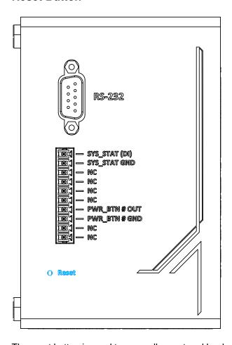
The reset button is used to manually reset and load system default configuration in case of a system halt or malfunction. To avoid unexpected operation, the button is purposely placed behind the panel. To reset the system, please use a pin to poke the button behind the panel for 5 seconds till one long beep heard.
