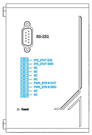
There are two signal pairs on the 10-pin I/O terminal block. One is power button signal output (PWRBTN#), the other is system status input (SYS\_STAT). Power button signal pair is sent by PB-9250J/ 4600J to turn on/off the back-end system. It should be linked to the remote control signal pair on the back-end system. The PWRBTN# signal pair is an open/ short signal. It is necessary to link the PWRBTN# signal pair in order for boot/ shutdown control.
