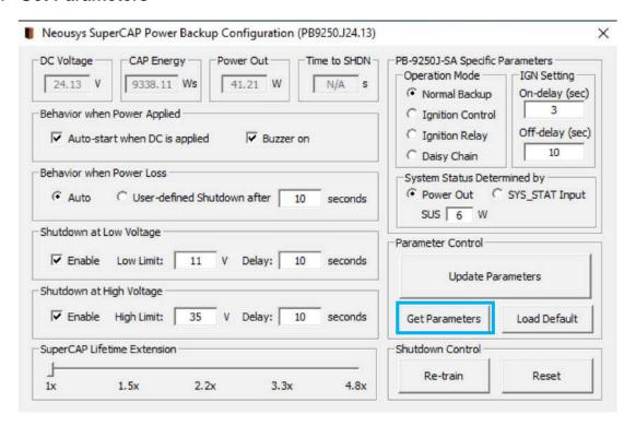
Click on "Get Parameters" to manually acquire the current PB-9250J/ 4600J status for DC voltage, current stored CAP energy and power output.
