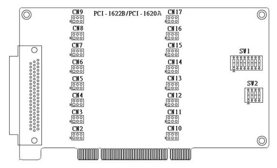
Figure 2.6 PCI-1622B/PCI-1620A/PCI-1620B Silk Screen
