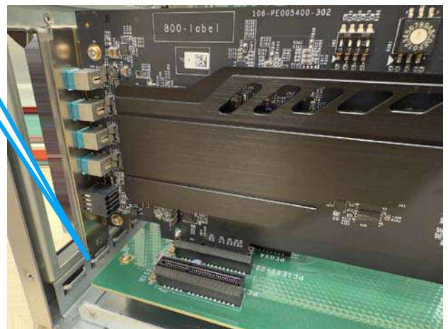
Make sure the card's panel is properly inserted into the enclosure hinge
