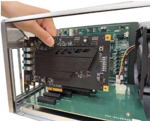
Align with PCIe slot
