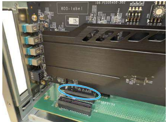
Insert gold fingers into PCIe slot
