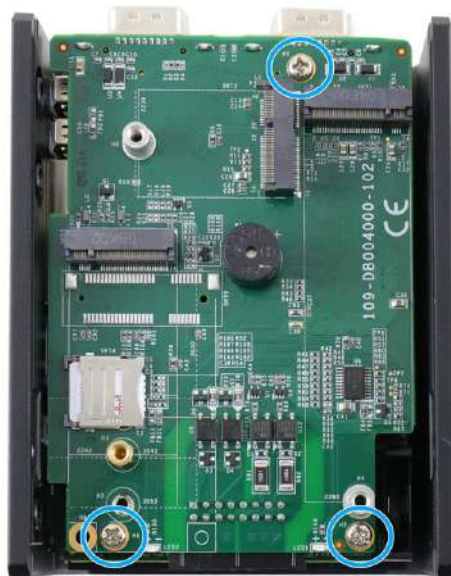
Remove the screws
