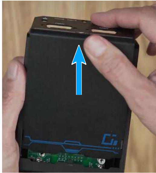
Slide open the L-shape panel
