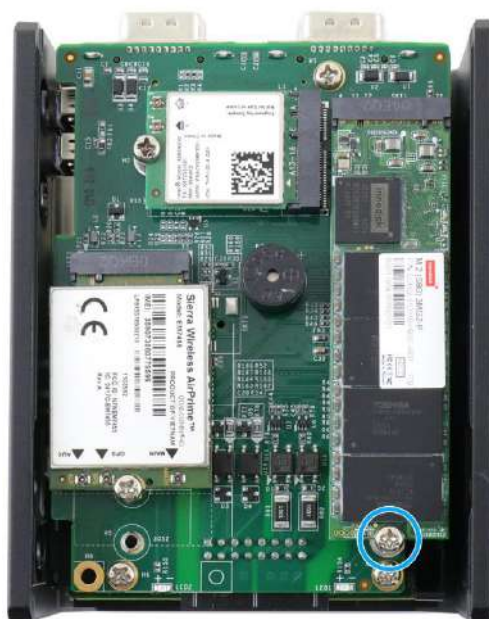
Secure with a screw
