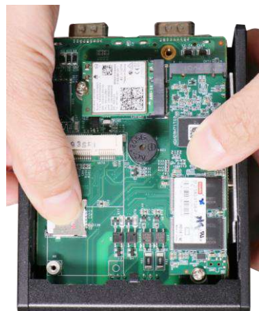
Secure micro SIM with cover
