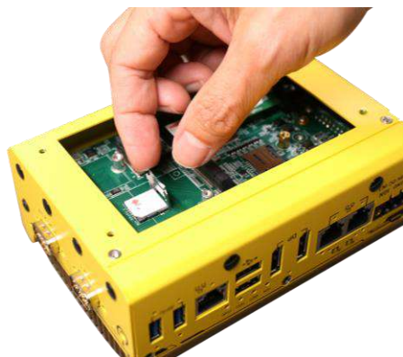
Place SIM into slot and close the bracket
