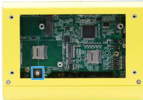
Remove bottom heatsink to locate ignition rotary switch
