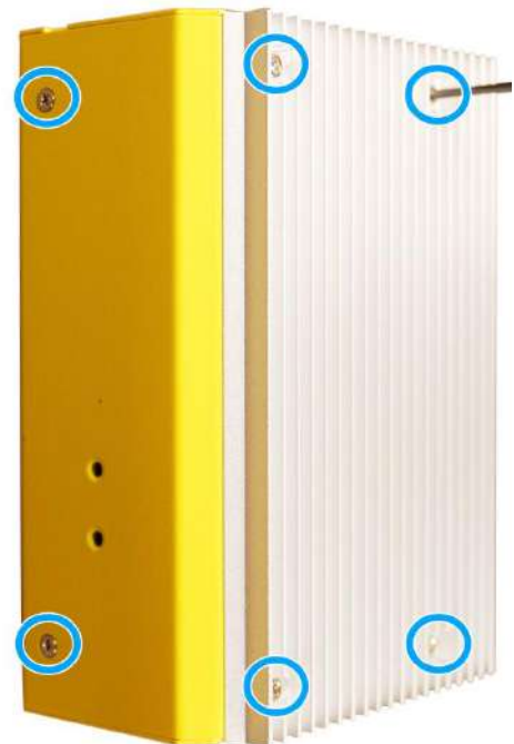
Screws on the bottom heatsink
