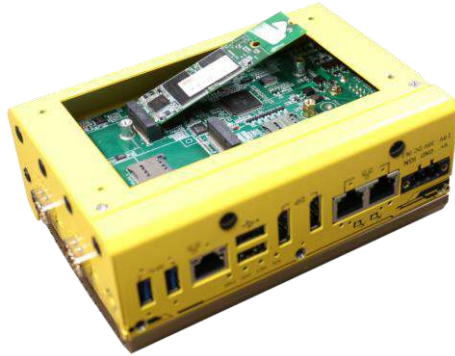
Insert on a 45 degree angle
