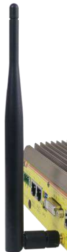
Secure antenna body on enclosure
