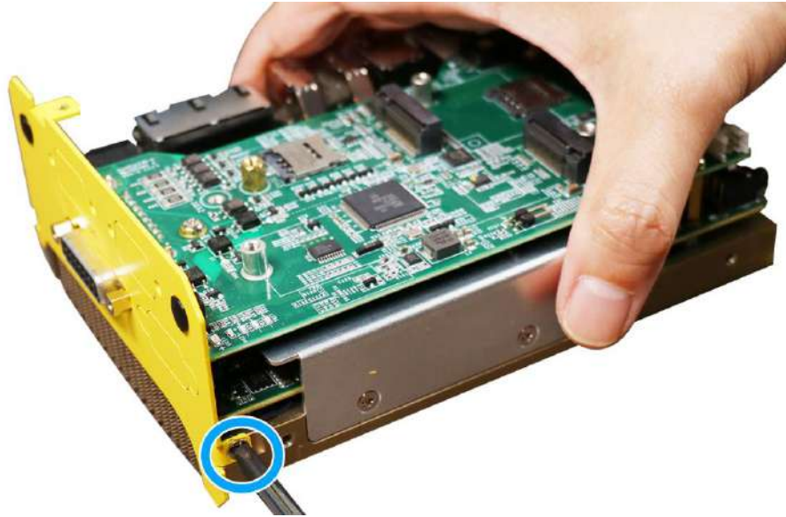
Remove the screw securing the DIO panel
