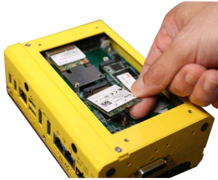
Insert on a 45 degree angle
