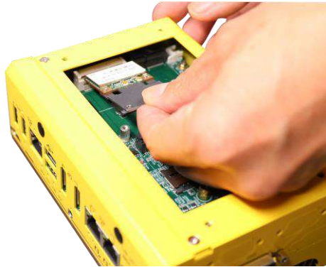
Insert on a 45 degree angle
