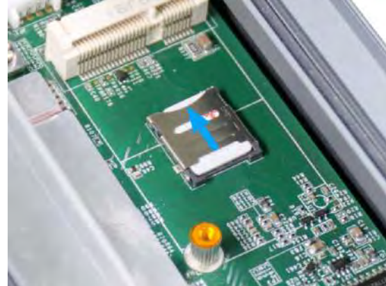
Slide to secure SIM and bracket
