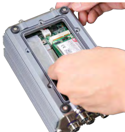
Insert at 45 degree angle
