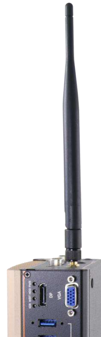
Attach external antenna
