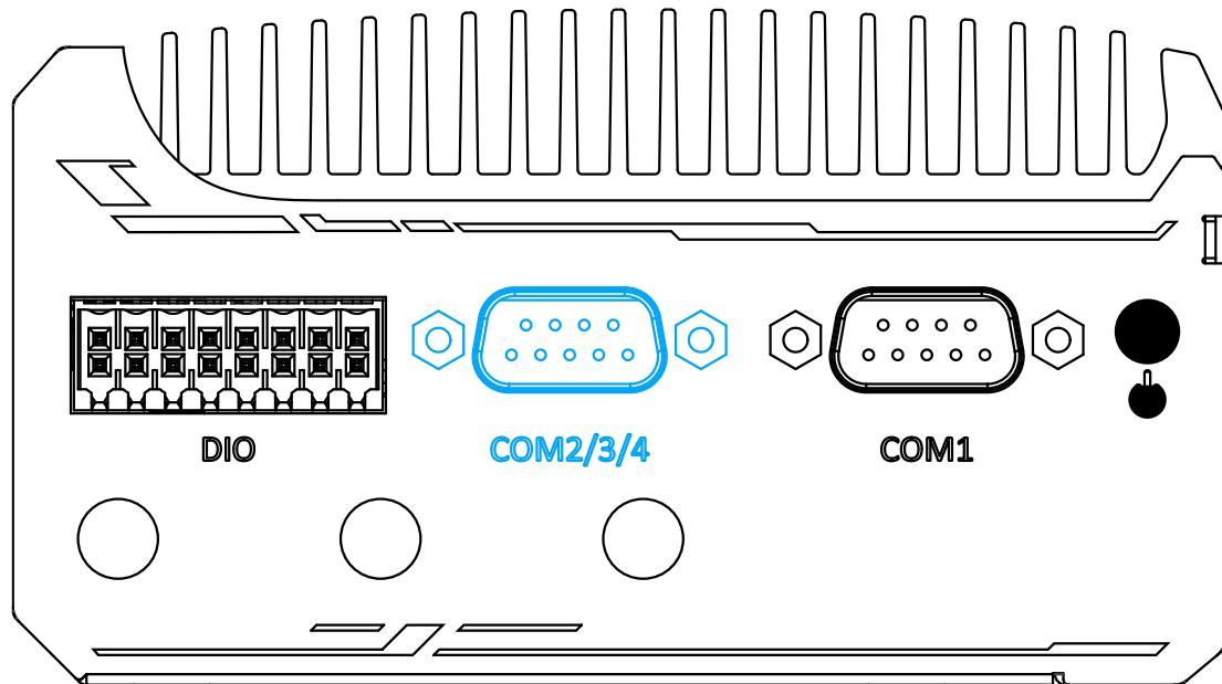
Implemented using industrial-grade ITE8786 Super IO chip (-40 to 85°C) and provide up to 921600 bps baud rate, the D-Sub male connector (COM2/ 3/ 4) can be configured in the BIOS as single RS-422/ 485 port (COM2) or three 3-wire RS-232 ports (COM2/COM3/COM4). Please refer to [COM2/ 3/ 4 Port Configuration](#) for configuring operation mode. An optional 1-to-3 Y-cable is available to connect three RS-232 devices.
