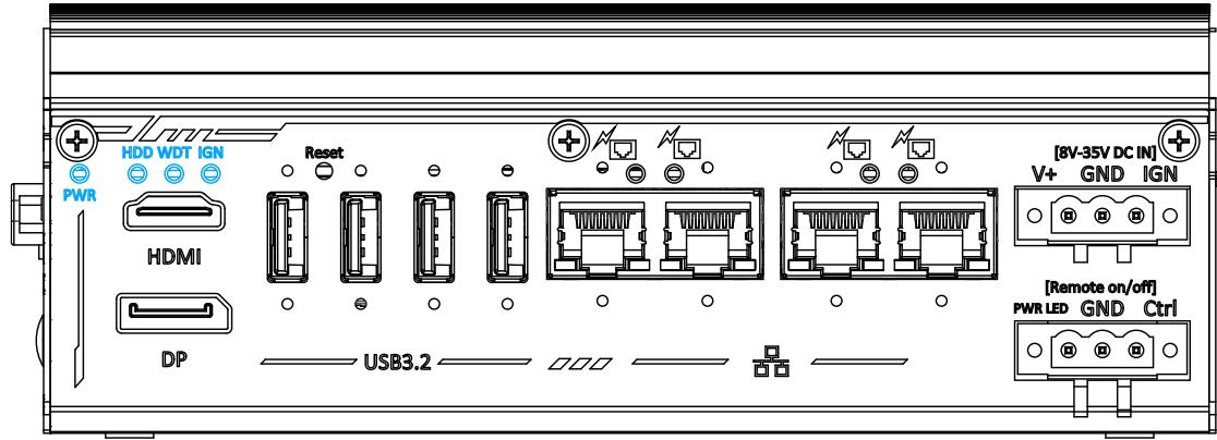
There are three LED indicators on the front panel: HDD, WDT and IGN. The descriptions of these LEDs are listed in the following table.
