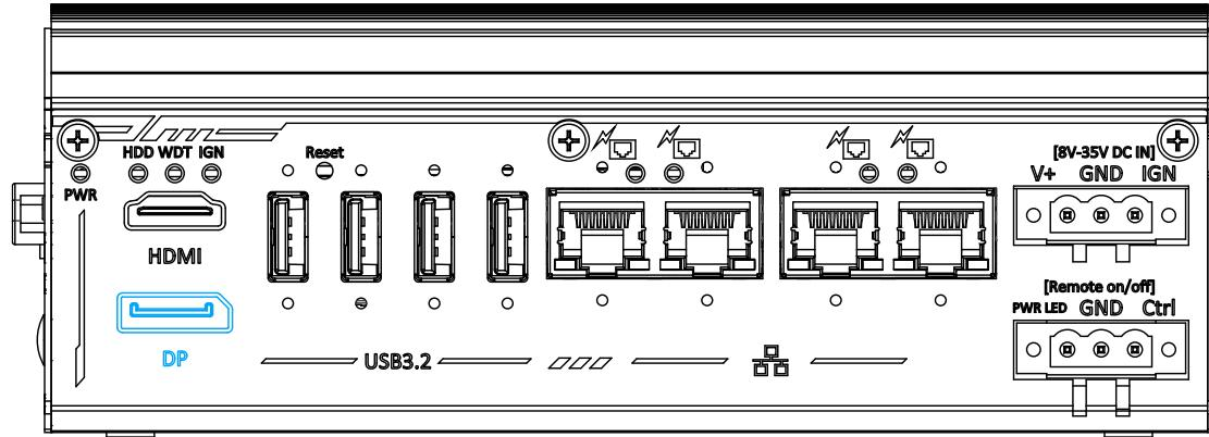
The system has a DisplayPort (DP) output which is a digital display interface that mainly connect video source and carry audio to a display device. When connecting a DP, it can deliver up to 4K UHD (4096 x 2160 @ 60Hz) in resolution. The system is designed to support passive DP adapter/ cable. You can connect to other display devices using DP-to-HDMI cable or DP-to-DVI cable.
