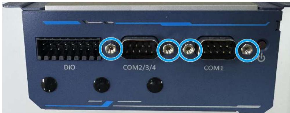
5. Separate the IO and bottom panel from the system
