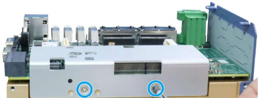
8. With external panels and DRAM/ M.2 heat spreader removed, you are ready to install internal components.
