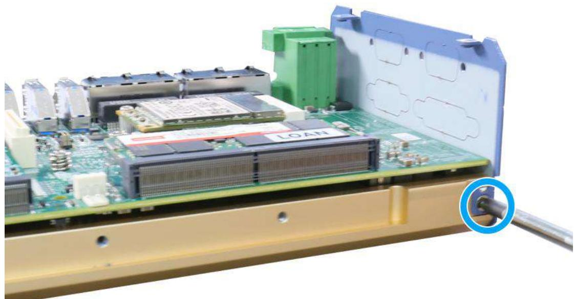
4. Remove the screws indicated and replace with stand-off hex bolt screws.
