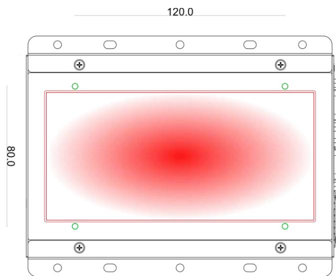
2. Find a flat spot on a metallic surface (eg. Inside of an enclosure wall), position the system approximately at the center, and secure with screws.
