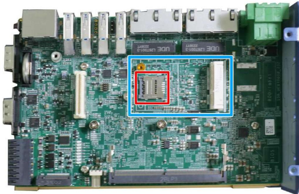
3. If you are installing a 4G/ 3G wireless module that requires a SIM, please install the SIM card first. Otherwise go to the next step. Push the SIM slot holder in the direction shown and flip open the holder to place the SIM into the slot.
