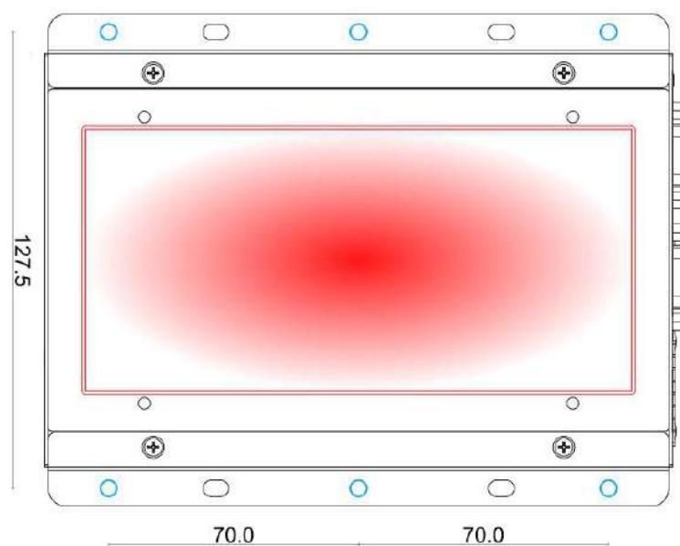
3. Find a flat spot on a metallic surface (eg. Inside of an enclosure wall), position the system approximately at the center, and secure with screws.
