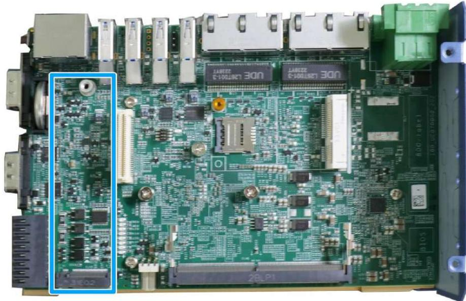
3. Insert the M.2 SSD into the slot on a 45° angle.
