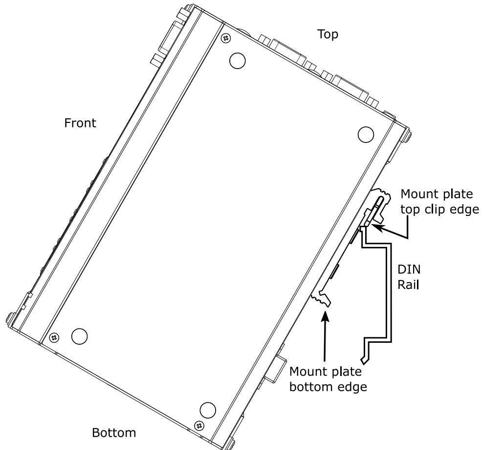
3. Confirm the mount plate has indeed clipped onto the DIN rail for proper fit to complete the installation.
