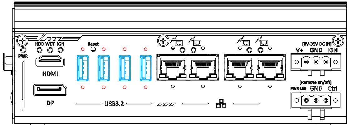
The system's USB 3.2 Gen2x1 ports (10Gbps) are implemented via native xHCI (eXtensible Host Controller Interface) controller and are backward compatible with USB3.2 Gen.1 USB 2.0, USB 1.1 and USB 1.0 devices. UEFI USB is also supported so you can use USB keyboard/ mouse in UEFI shell environment. Indicated in red are screw-lock holes for the corresponding USB port.
