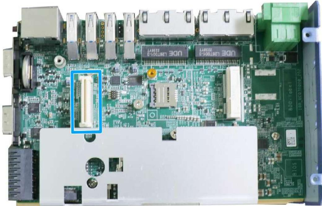
MezIO® is an innovative interface designed for integrating application-oriented I/O functions into an embedded system. It offers computer signals, power rails and control signals via a high-speed connector. MezIO® is also mechanically reliable benefited from its 3-point mounted mezzanine structure. A MezIO® module can leverage these signals to implement comprehensive I/O functions.
