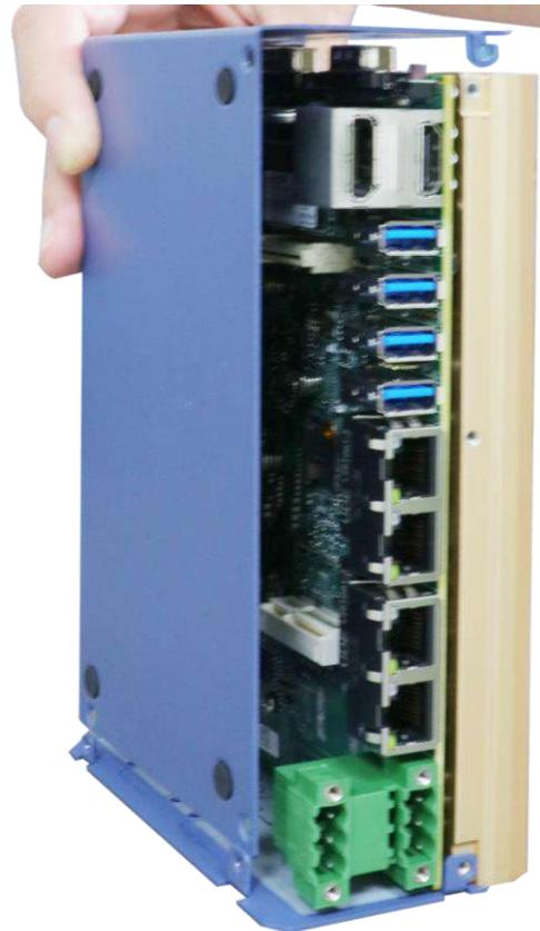
2. Install the front panel and securing it with three (3) screws.
