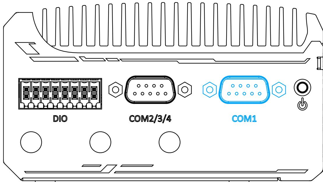
Implemented using industrial-grade ITE8786 Super IO chip (-40 to 85°C) and provide up to 921600 bps baud rate, COM1 is a software-configurable RS-232/422/485 port via 9-pin D-Sub male connector. The operation mode, slew rate and termination of COM1 can be set in BIOS setup utility. The following table describes the pin definition of COM ports.
