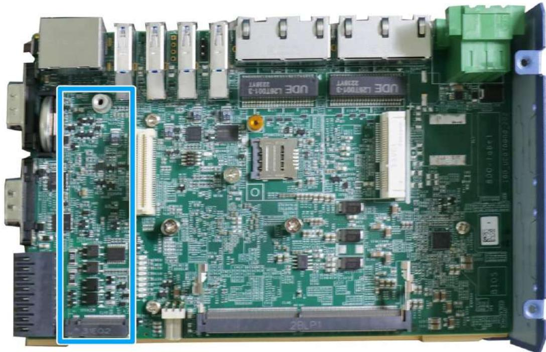
The system has an M key M.2 2280 slot supporting PCIe Gen3 x1 signal for NVMe SSD storage, and it also supports SATA signal for SATA SSD. Users can install an SSD for improved disk read/ write performance over mechanical hard drives or 2.5" SSDs.
