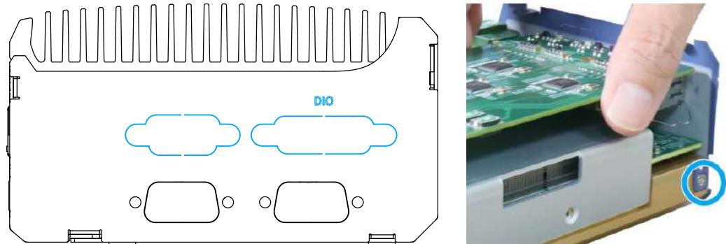
**Remove the corresponding punch out plates (may differ depending on your MezIO® module)**
