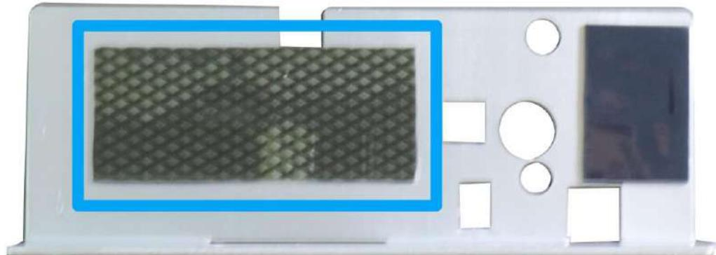
5. Secure the DRAM/ M.2 heatsink spreader onto the side of the system heatsink.
