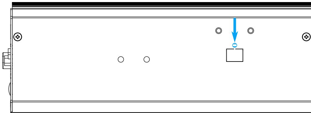
Positioned on the rear panel (opposite the IO panel), indicated by the **blue arrow**, the CMOS Reset button is used to manually reset the motherboard BIOS in case of system halt or malfunction. To avoid unexpected operation, it is purposely placed behind the panel. To reset, please use the tip of a pen, press and hold for at least 5 seconds to reset the BIOS.
