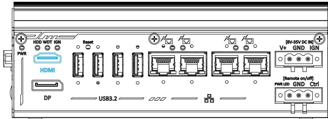
The High-Definition Multimedia Interface (HDMI) port provides uncompressed high-quality digital video and audio transmission between the system and a multimedia display device on a single cable. You can connect to other digital inputs by using a HDMI-to-DVI or HDMI-to-DP cable.
