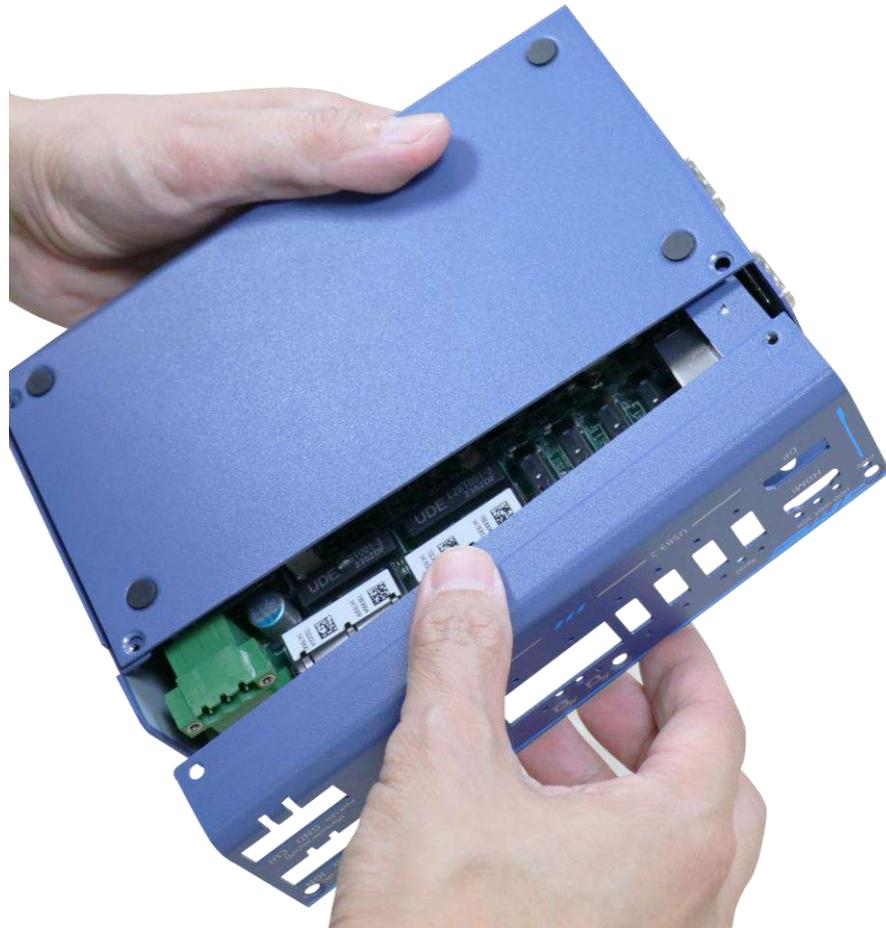
4. Secure the front panel with screws indicated.
