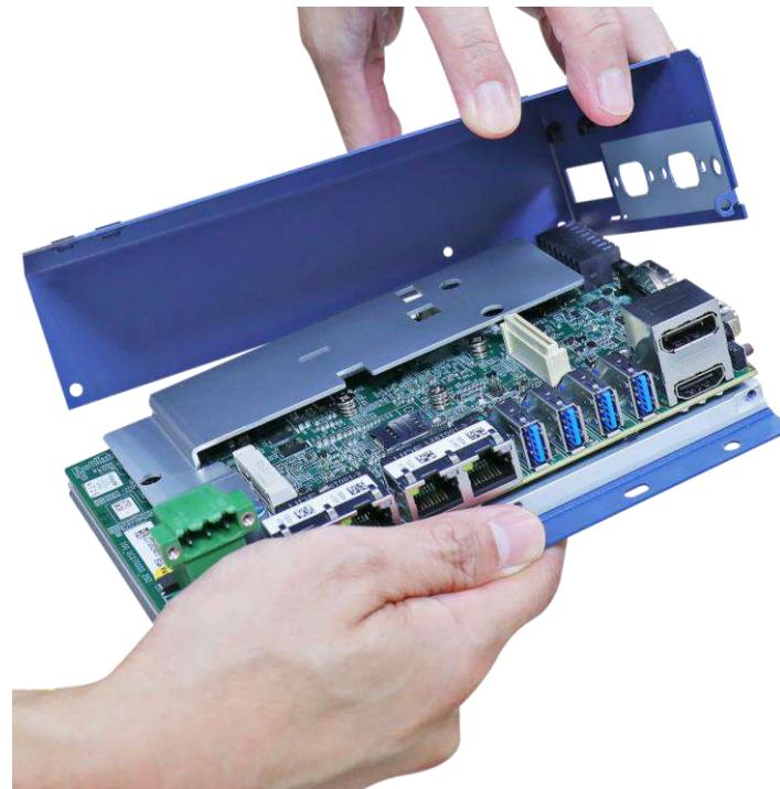
7. Unscrew the two (2) screws to remove the DRAM/ M.2 heat spreader.
