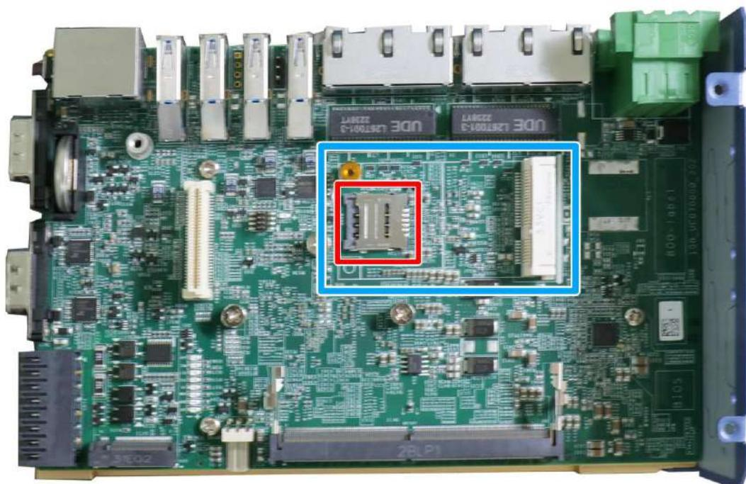
The system provides a full-size mini-PCIe socket (indicated in blue) designed with SIM card (indicated in red) support. With a SIM card installed, your system can access the internet via your network provider's 3G/ 4G network.
