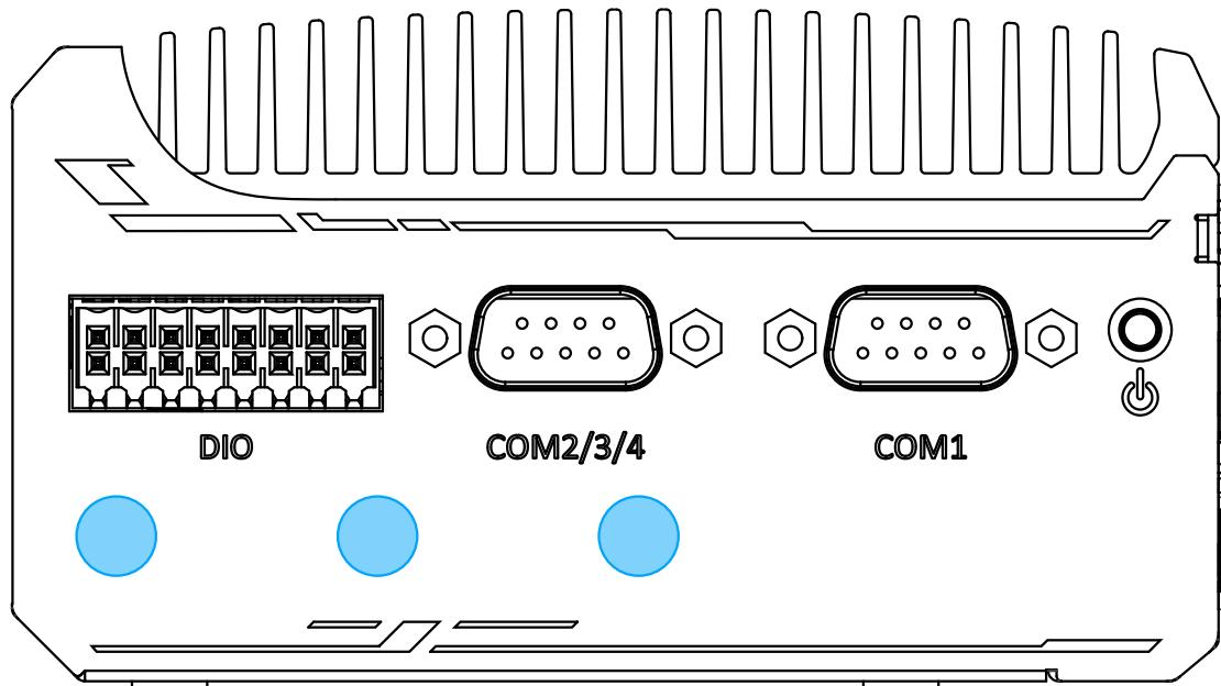
The system offers three SMA antenna openings reserved for SMA antenna installations. Users can take advantage of these three openings when installing mini-PCIe module for wireless communication reception such as 3G, 4G, GPS or WiFi.
