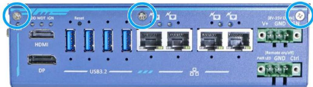
2. Remove the three (3) screws at the bottom.
