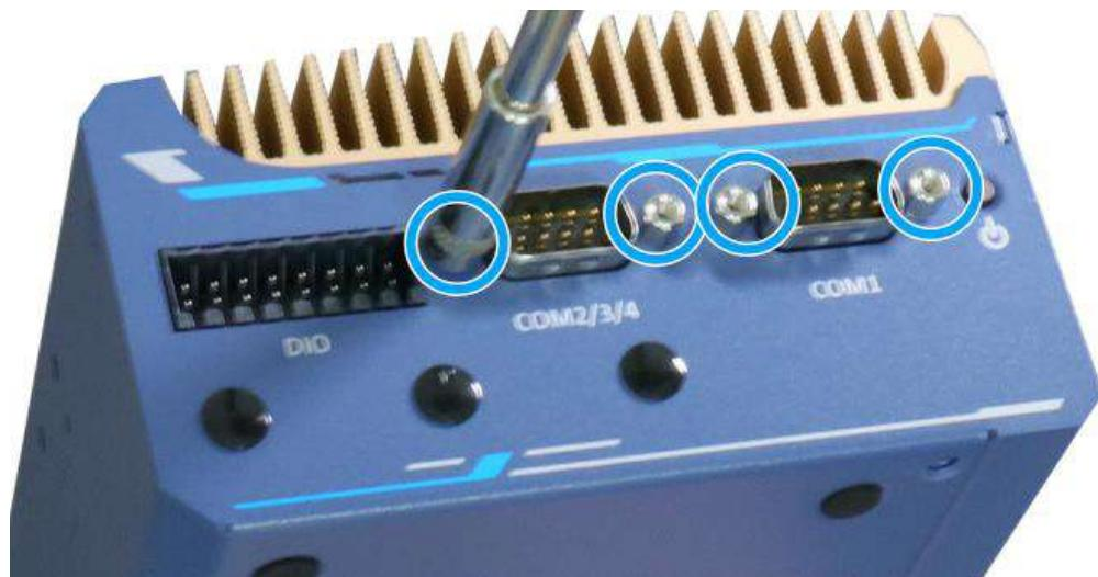
5. Separate the IO and bottom panel from the system
