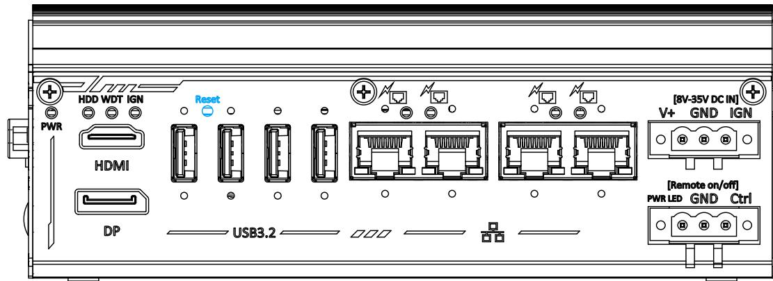
The reset button is used to manually reset the system in case of system halt or malfunction. To avoid unexpected reset, the button is purposely placed behind the panel. To reset, please use a pin-like object (eg. tip of a pen) to access the reset button
