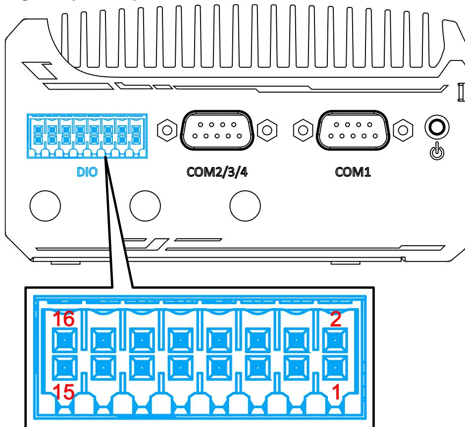
The system provides 4x isolated digital input channels and 4x isolated digital output channels. The DIO functions support polling mode I/O access and DI change-of-state interrupt. Please refer to [Watchdog Timer & Isolated DIO](#) for information on wiring and programming the isolated DIO channels.
