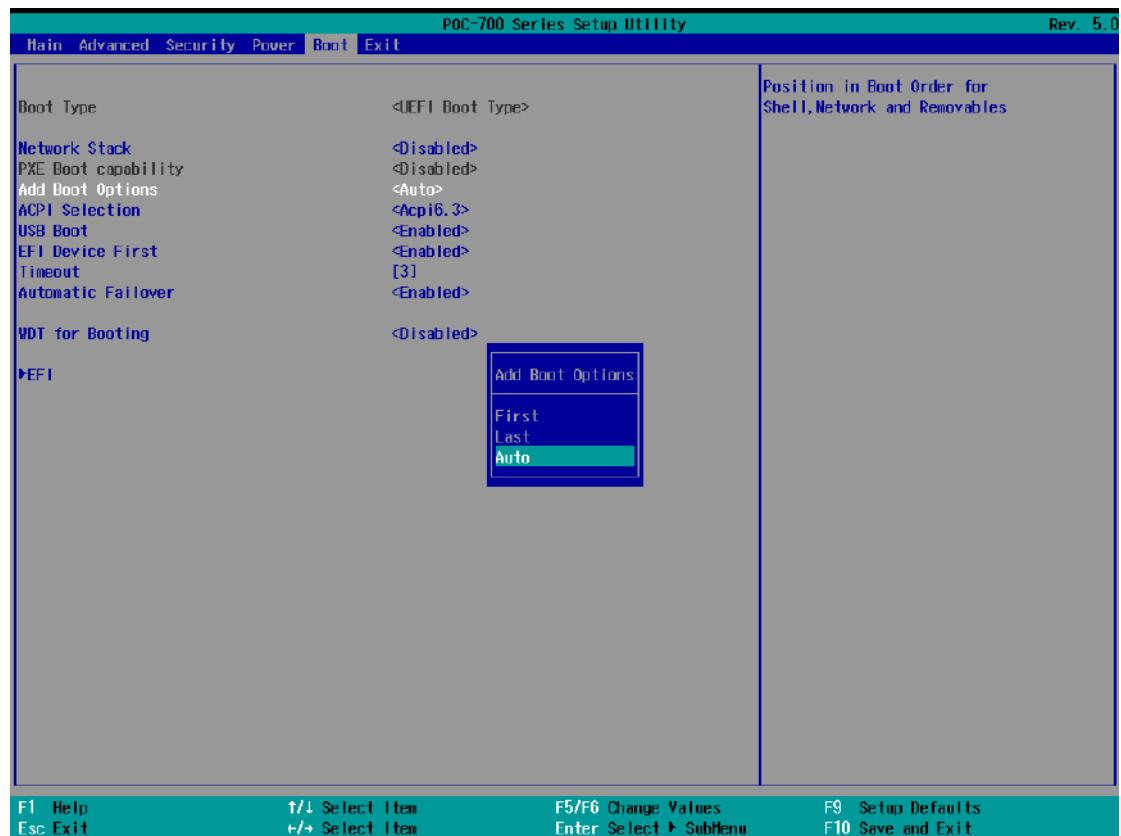
To set the newly-installed boot device as the first or last boot device:
