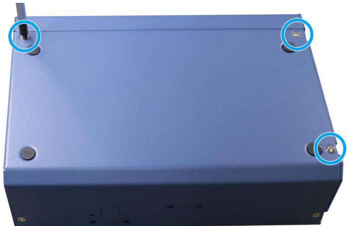
3. Remove the two (2) screws on the read panel.
