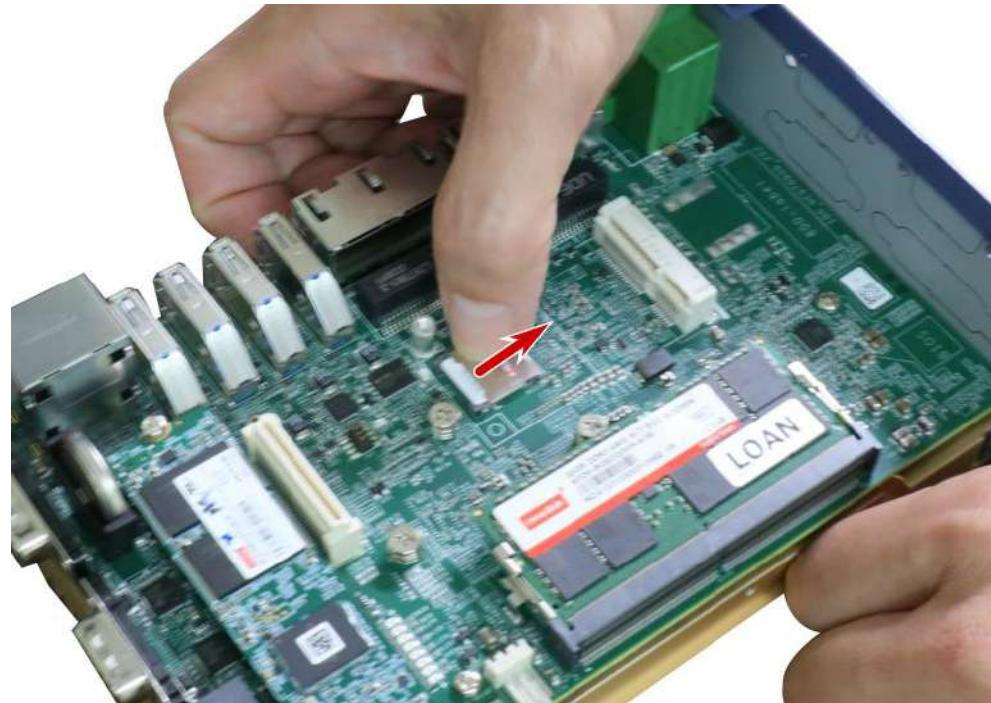
5. **To install**, insert mini-PCIe module's gold finger on a 45 degree angle into the socket, gently press the module down and secure it with a screw.
