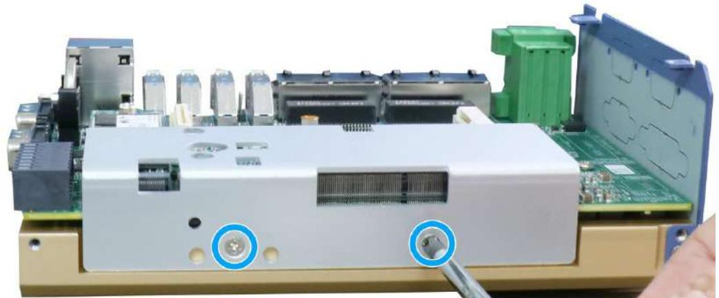
7. With external panels and DRAM/ M.2 heat spreader removed, you are ready to install internal components.
