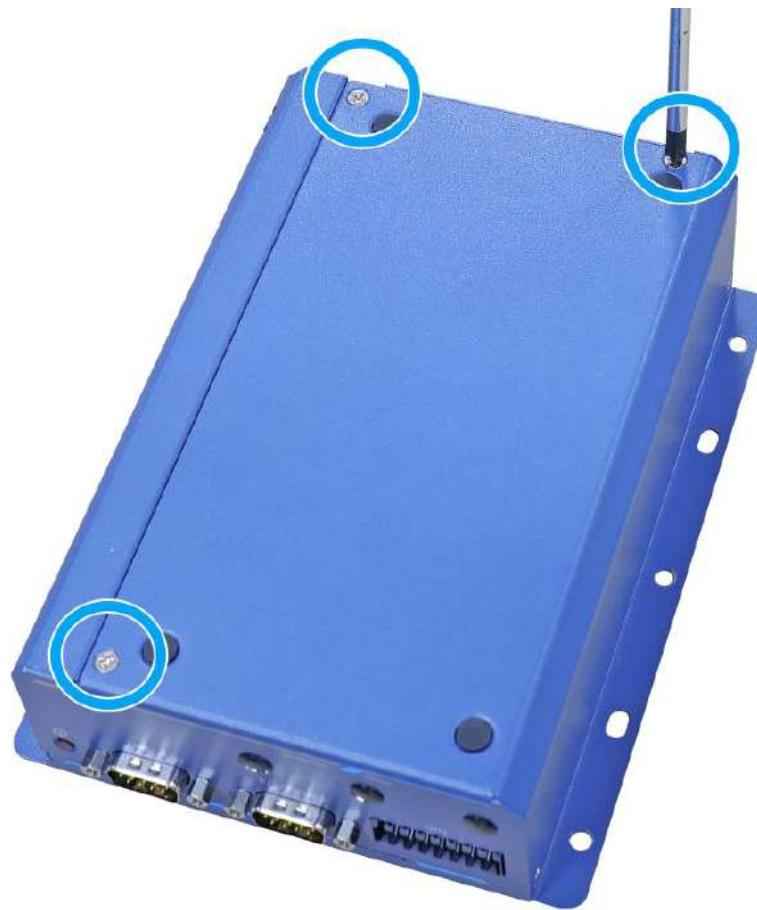
6. Secure the hex bolt screws on the DIO/ COM port panel to complete the enclosure installation.
