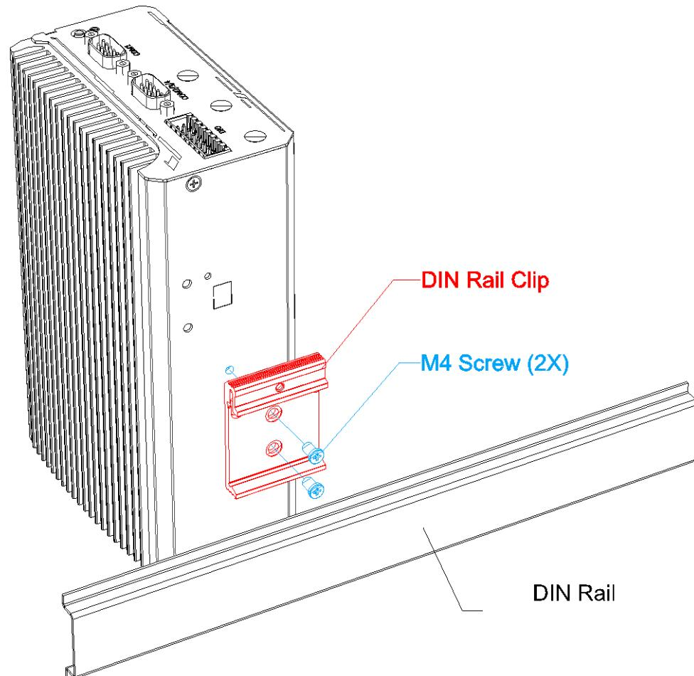
2. To install the DIN rail clip onto the DIN rail, you must come over the top of the DIN rail, tilting, overlap the top clip edge of the DIN rail clip onto the DIN rail first, and then firmly press the bottom-front of the enclosure to clip the bottom edge of the mount plate.
