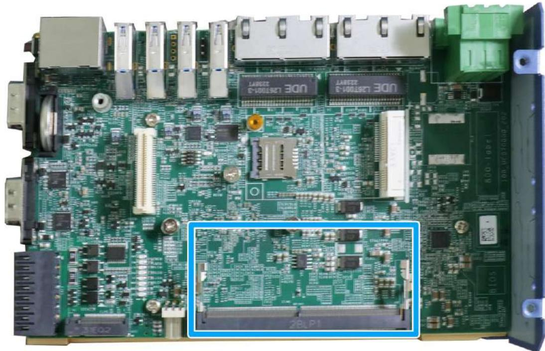
The system supports one SO-DIMM socket for installing DDR5-4800 memory module up to 16GB in capacity.
