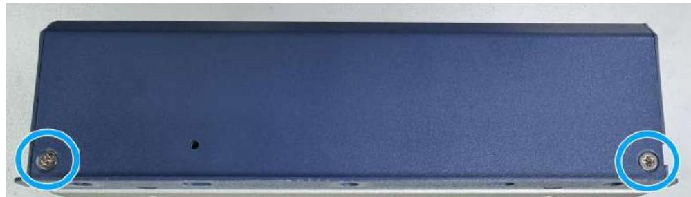
4. Remove the four (4) hex bolt screws on the DIO/ COM port panel.
