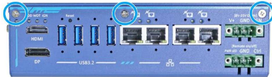
5. Secure the bottom with screws indicated.
