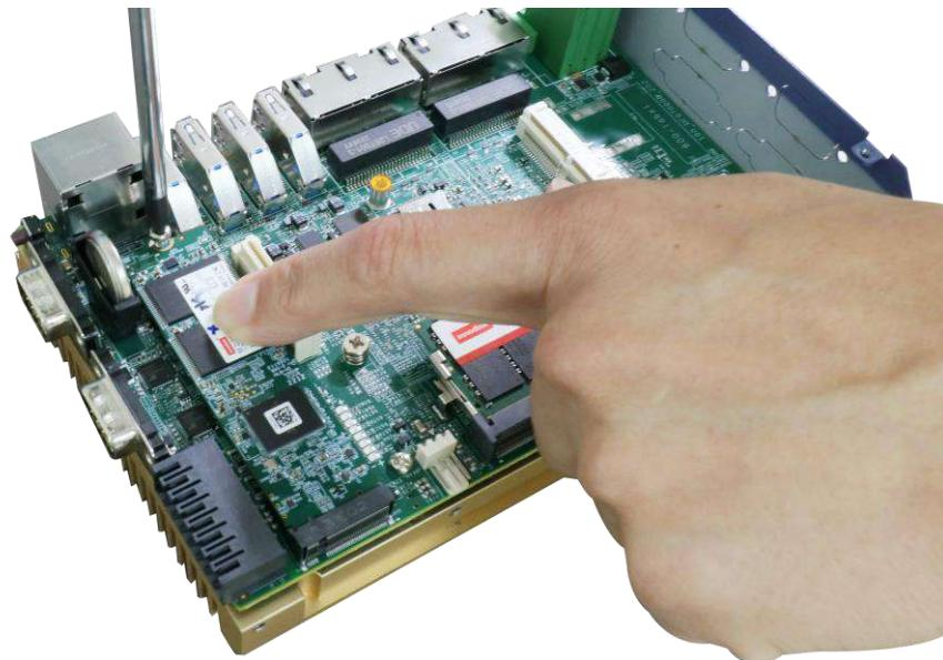
5. Once you have installed the NVMe SSD, you need to reinstall the heat spreader but before you do so, please make sure the protective film on the thermal pads have been removed.
