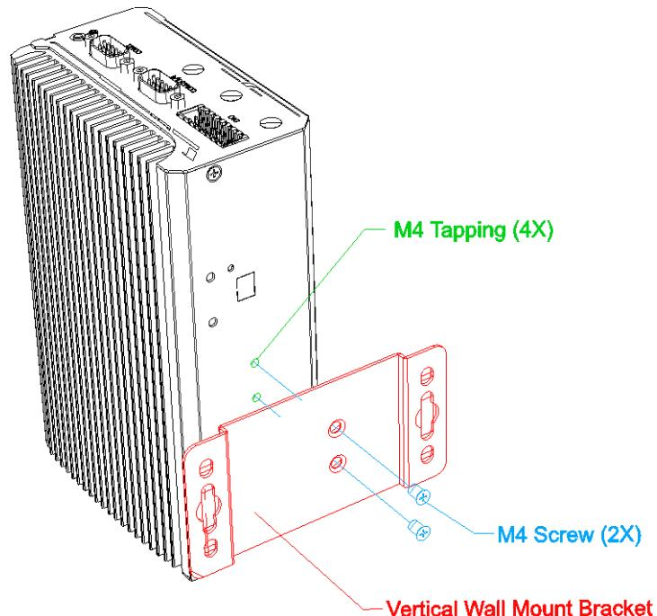
2. Dimension illustration of the install vertical wall mount bracket for you reference.
