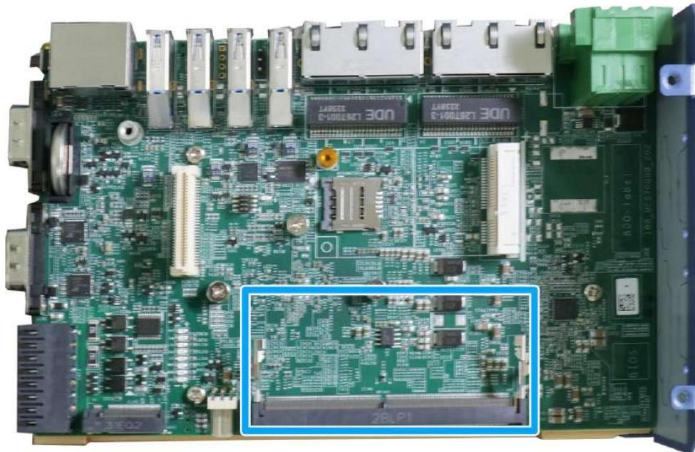
3. **To install**, insert the gold finger end of the SO-DIMM on a 45 degree angle into the slot and gently push the SO-DIMM down until it is clipped-in.
