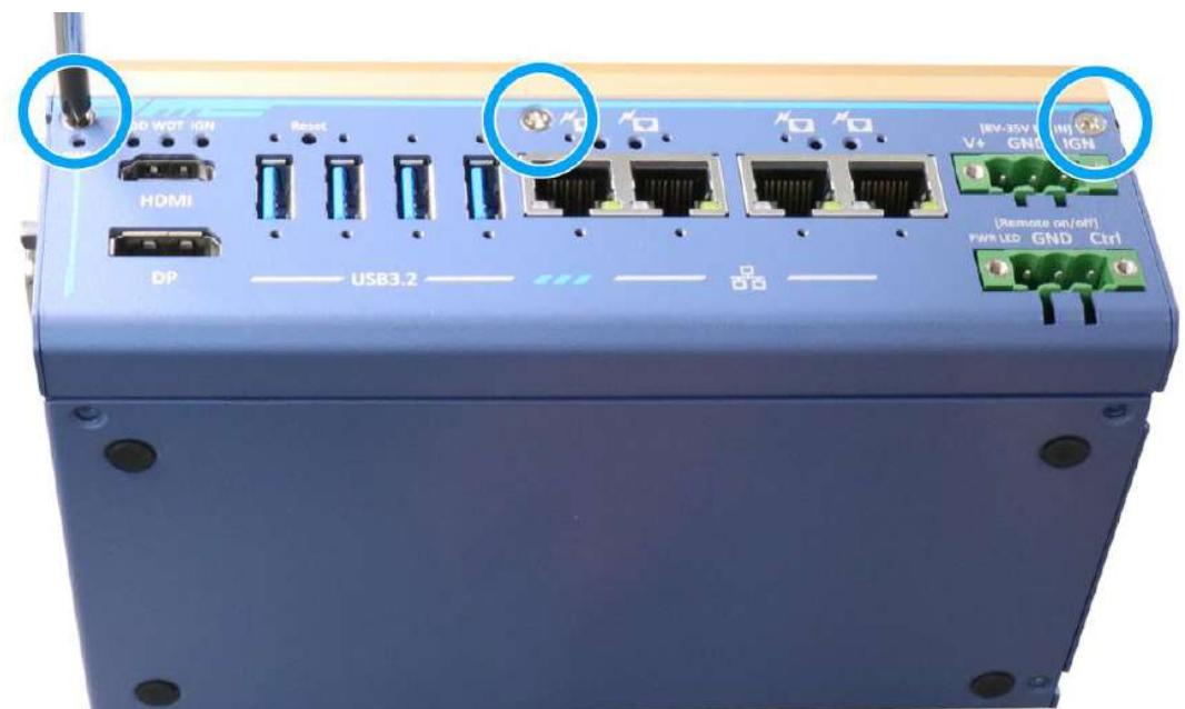
3. Secure the bottom and rear panel with screws.
