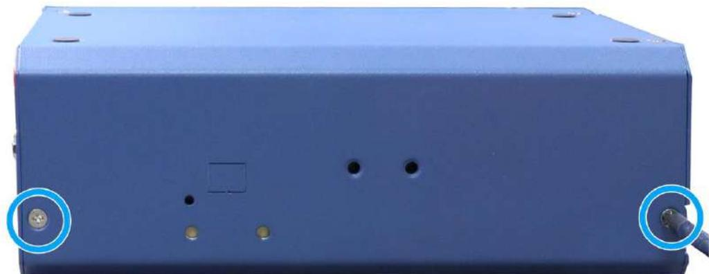
4. Remove the four (4) hex bolt screws on the DIO/ COM port panel.
