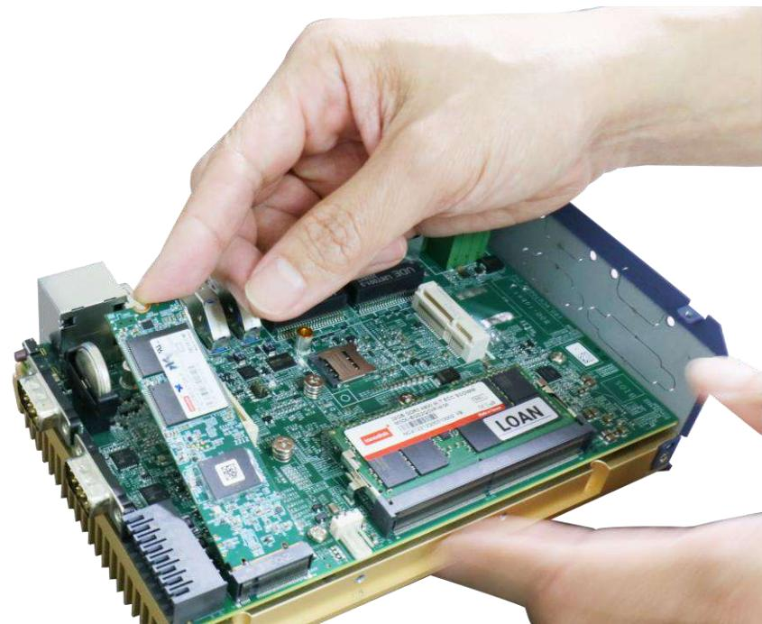
4. Gently push it towards the motherboard and secure the NVMe SSD with the supplied screw.
