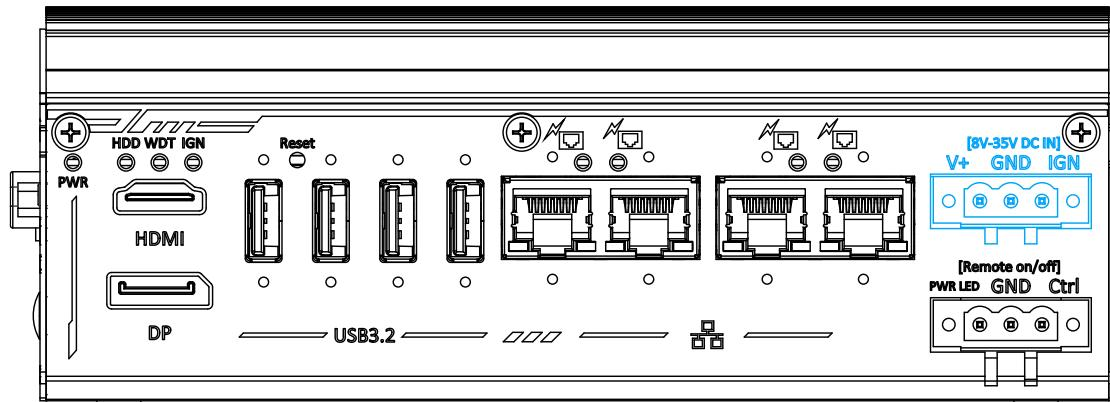
The system accepts a wide range of DC power input from 8V to 35V or 12V to 35V (UL series) via a 3-pin pluggable terminal block, which is fit for field usage where DC power is usually provided. The screw clamping mechanism on the terminal block offers connection reliability when wiring DC power.
