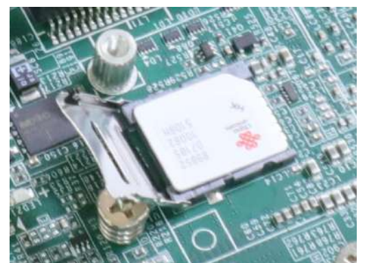
Push the SIM holder in the direction shown Flip open the holder and place SIM
