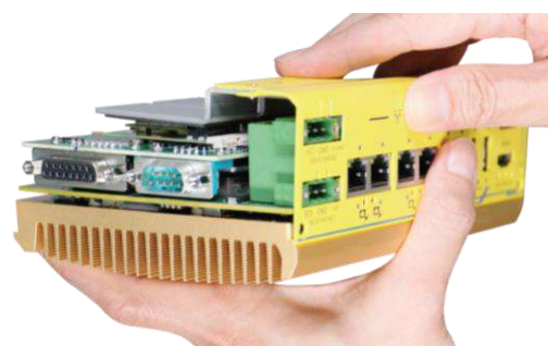
Install I/O panel
