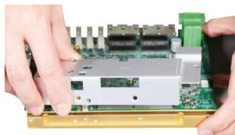
Separate the heat spreader from system
