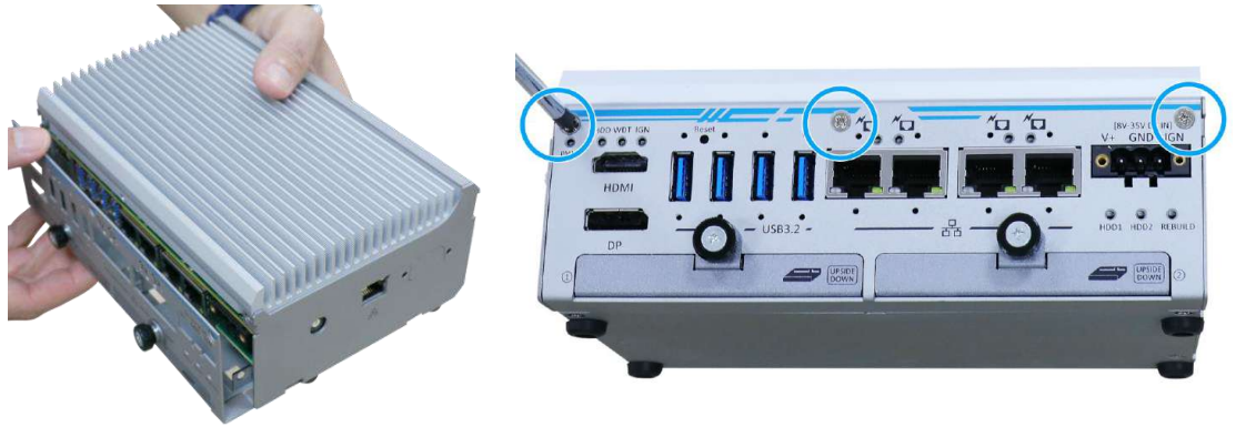
Install front panel
