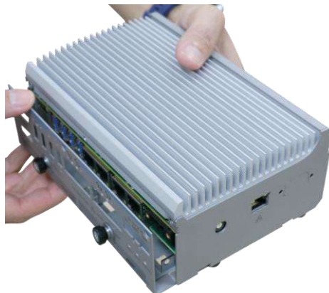
Remove front IO panel
