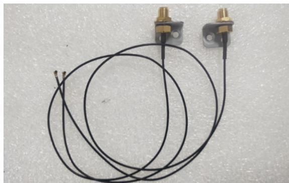
Figure 2.15 Assemble the Bracket with the Antenna Cable
