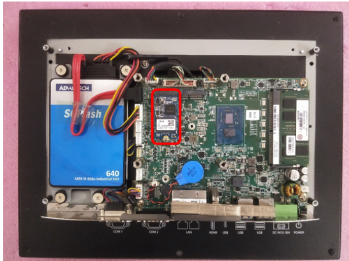
Figure 2.13 Install the M.2 2242 Card on the Motherboard
