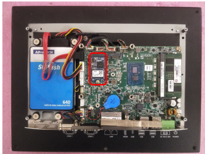
Figure 2.13 Assemble Pillar on Motherboard
