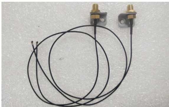
Figure 2.15 Assemble Bracket with Antenna Cable
