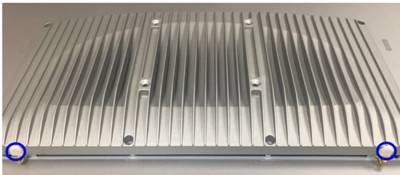
Figure 2.16 Removing plugs for the antennae
