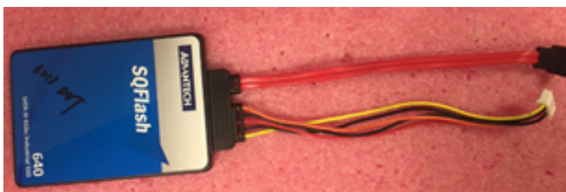
Figure 2.9 SATA cable connected to SATA HDD
