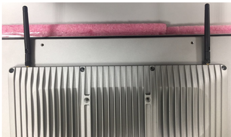
Figure 2.17 Location of external antennae
