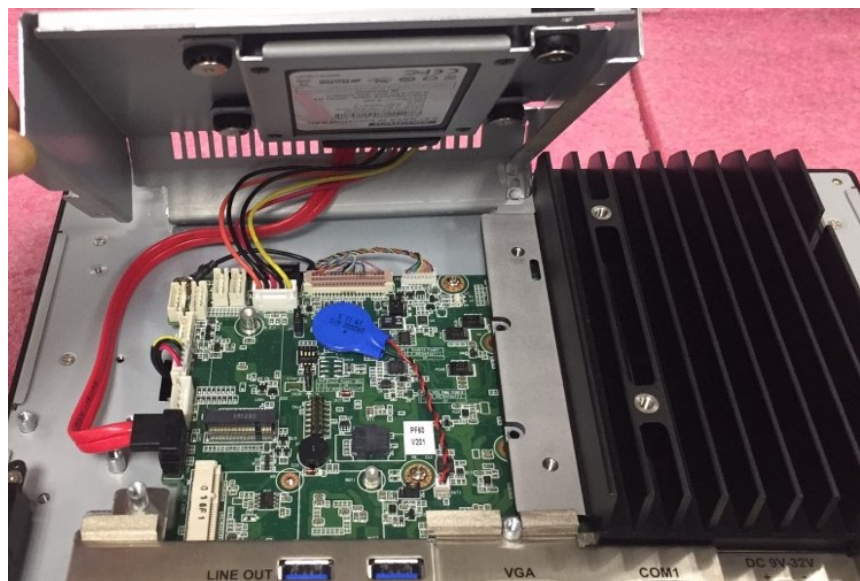
3. Lock the HDD bracket, and connect the HDD cable to the mainboard (see Figure 2.12).
