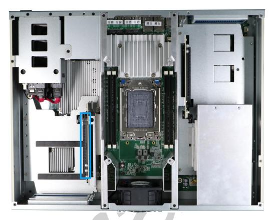
The system has two slots that are PCIe x16 Gen4 8-lanes (indicated in blue) for installing add-on cards, for additional I/O expansion or function cards (eg. frame grabber card).
