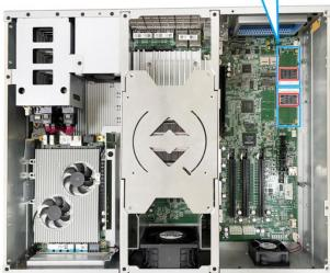
The system provides two mini-PCIe sockets (indicated in blue) that is in compliance with mini-PCIe specification rev. 1.2. This mini-PCIe socket is designed with SIM card (slot indicated in red) support. With a SIM card installed, your system can access the internet via your network provider's 4G/3G network.
