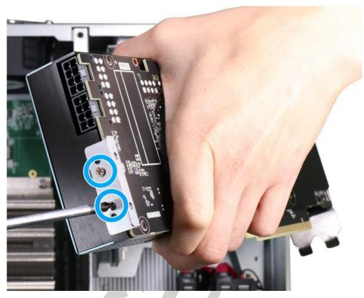
6. Connect the unplugged power cables from the motherboard to the inference accelerator.
