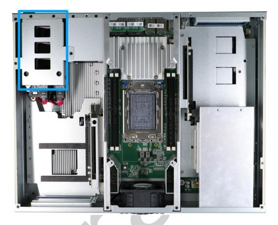
The system provides a 2.5" hard drive cage that can hold up to four 2.5" HDDs/ SSDs with each connected via a Gen3, 6 Gb/s SATA port. The installation trays can be accessed via the I/O panel.
