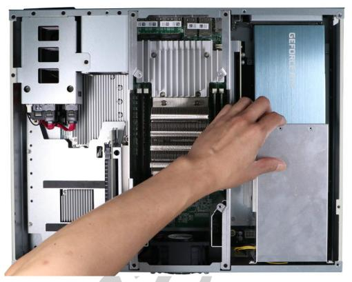
14. Secure the screw on the side of the tunnel duct.
