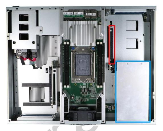
The system features a PCIe x16 slot (indicated in red) and supports an inference accelerator (NVIDIA RTX A6000 or A4500), providing up to 38.7 TFLOPS FP32 or 309.7TFLOPS tensor performance. There is also a dedicated inference accelerator tunnel duct (indicated in blue) optimizing airflow to ensure operation stability.
