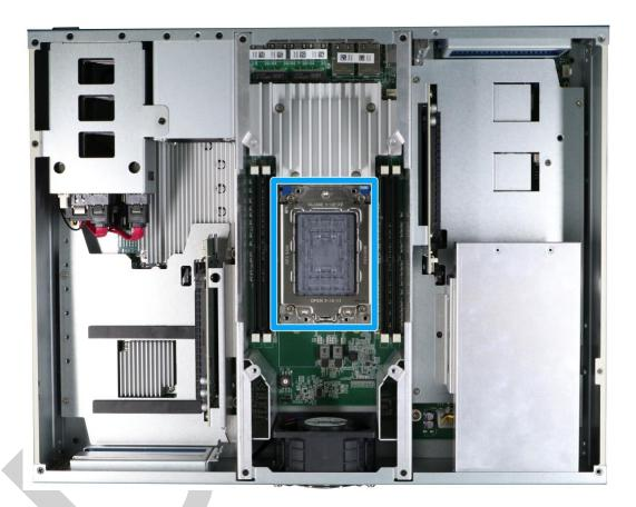
The system supports server-grade AMD EPYC<sup>™</sup> 7003 series processors that are based on Zen-3 and Infinity microarchitecture. With industry leading IO, 7nm manufacturing, integrated on-die security processor, supporting up to 64 cores/ 128 threads while providing up to 32MB L3 cache per core, interleaving multi-channel memory optimization, etc., it delivers one of the best CPU performances in the industry.
