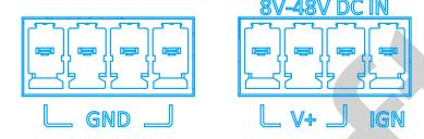
To have ignition power control for in-vehicle usage, you need to supply IGN signal to the system. The IGN input is located on the 3-pin pluggable terminal block (shared with DC power input). Below is the typical wiring configuration for in-vehicle applications.
