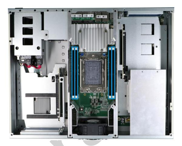
The system supports four registered DDR4 DIMMs up to 3200MHz, and up to 512GB in capacity. When installing the modules, please install into the specific slots accordingly. For details, please refer to the <u>Registered DDR4 Module Installation</u> section.
