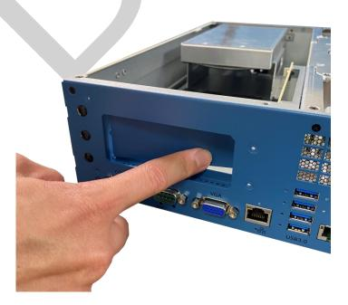
3. To install the inference accelerator, uninstall the tunnel duct by removing the screws shown.
