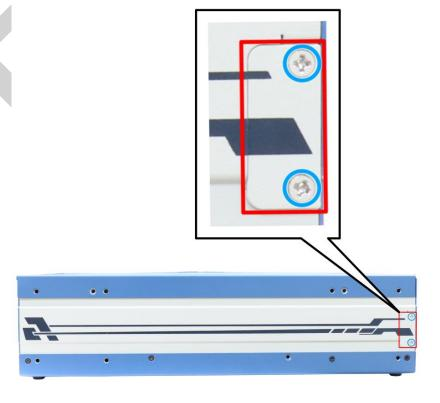
9. Secure the inference accelerator's panel with a screw.
