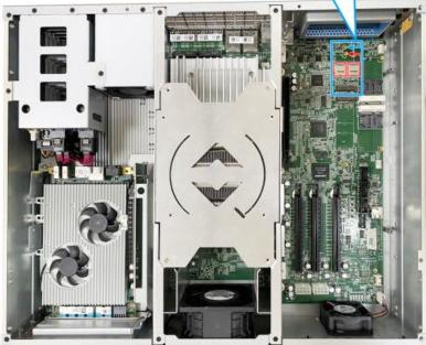
The system has an M.2 3042/3052 slot (indicated in **blue rectangle**) with a 5G/4G SIM slot (indicated in **red rectangle**). A copper standoff is provided for you to secure onto the motherboard into the **red arrow** location for an M.2 3042 module, or into the **blue arrow** location for an M.2 3052 module. By installing a 5G or 4G M.2 module and SIM card, you can access the internet via the provider's network.
