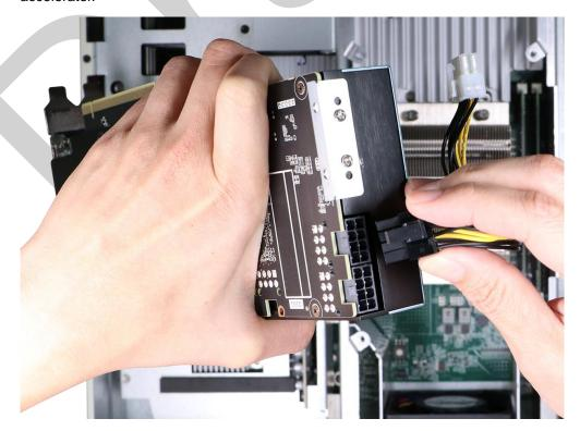
7. With the power cable end facing the fan side, align and insert the goldfingers of the inference accelerator to the PCle x16 slot.
