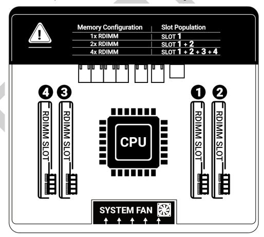
5. To install the memory module, match the goldfinger notch to the position on the slot, insert DRAM's gold fingers into the slot at a perpendicular angle, push the memory module down until clips on the sides clip the module into position.
