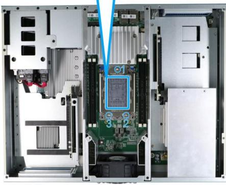
5. Lift the CPU load plate, and gently remove the CPU socket protective cover.
