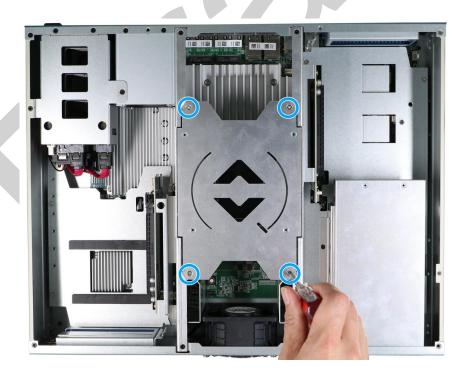
7. Place the enclosure panel back on top of the system.
