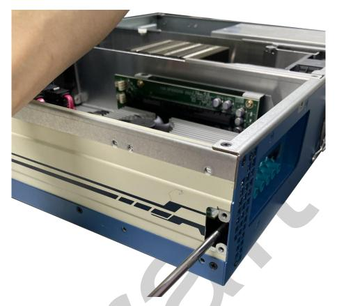
6. For a standard full-size PCIe card, there are L-shaped stopper brackets in the accessory box for securing the add-on card in place. Depending on the size of your add-on card, locate the appropriate screw-holes for placement. Secure two screws to position the stopper bracket in-place.
