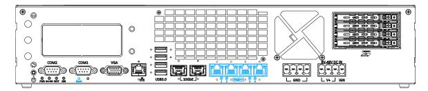
The system offers four GbE ports (in **blue**) that are implemented with Intel I350-AM4 Ethernet controller that supports Wake-on-LAN. There are also panel screw fix holes (indicated in **red**) for a firm and secure connection.
