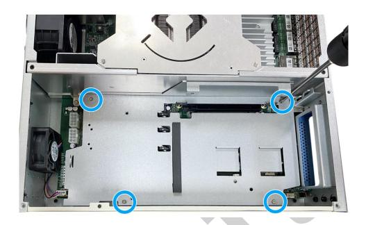
12. Gently wiggle and remove the platform, and you should see the system's M.2, mini-PCIe, and SIM slots.
