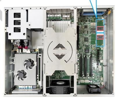
3. Before installing the mPCIe module, you need to insert the mini-SIM card. Slide the SIM slot holder and lift the SIM card holder. Insert the mini-SIM card (pins facing up), shut the SIM holder and slide it to lock the SIM card in-place.
