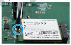
5. Clip on the IPEX-to-SMA cable to the module and secure the antenna to the front or rear panel. Please refer to the module's manual for clip-on connection.
