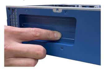
3. Take the PCIe card out of its box/ static bag, align and insert the goldfingers into the PCIe slot. There are two slots available, it is recommended to install into the bottom slot first.
