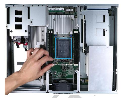
6. Gently pull the **blue tab** (indicated by the **red arrows**) to lift the CPU frame rail (indicated in **green**).
