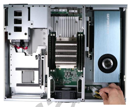
12. Secure the L-shape stopper at the end of the inference accelerator.
