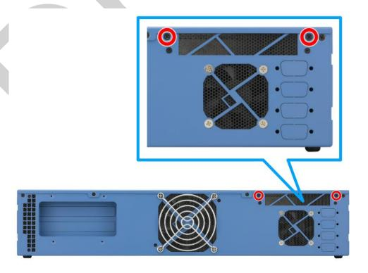
9. With the duct removed, remove the four screws holding the PCIe riser card.
