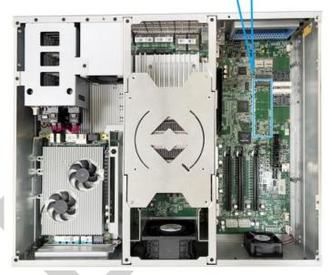
The system has an x4 PCIe M.2 2280 slot for you to install an NVMe SSD for the fast read/ write performance. An NVMe SSD offers significant performance advantages over 2.5" SSDs.
