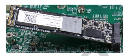
3. Gently press down and secure the module with an M2.5 P-head screw.
