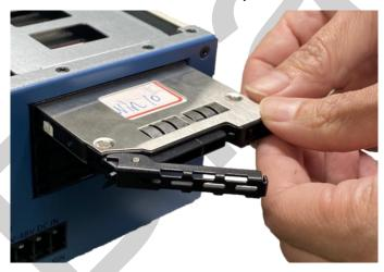
4. Gently place and push the tray back into the enclosure to complete the disk drive installation. Please repeat steps 1 to 4 if you need to install disk drives into other trays.
