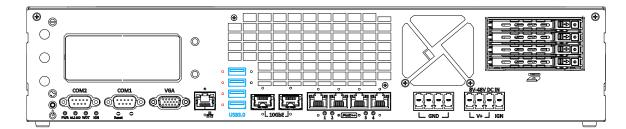
The system's USB 3.2 Gen1x1 ports (5Gbps) are backward compatible with USB 2.0, USB 1.1 and USB 1.0 devices. UEFI USB is also supported so you can use USB keyboard/mouse in UEFI shell environment. Indicated in **red** is a screw-lock hole for the corresponding USB port.
