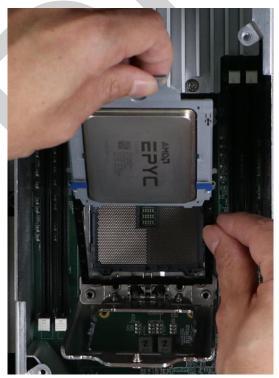
Insert into CPU frame rail
