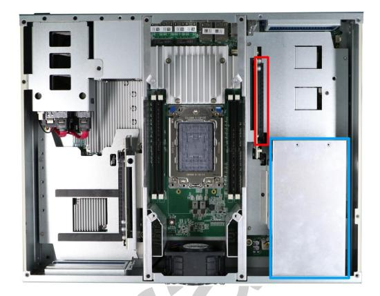
The system has a PCIe x16 (indicated in **red**) that supports an NVIDIA A6000 or A4500 inference accelerator to provide up to 38.7 TFLOPS FP32 or 309.7TFLOPS tensor performance. There is also a dedicated inference accelerator bracket (indicated in **blue**).
