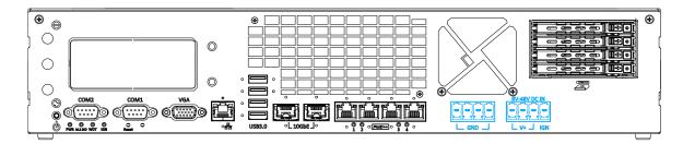
The system accepts a wide range of DC power input from 8 to 48V via dual 4-pin pluggable terminal blocks, fit for field usage where DC power is usually provided. The screw clamping mechanism on the terminal block offers connection reliability when wiring DC power.
