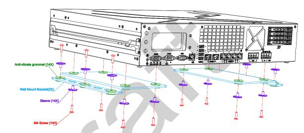
3. View of the installed bracket onto the system.
