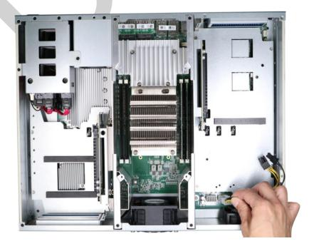
5. Take the inference accelerator out of its box/ static bag, and attach the L-shape stopper to the power connector end of the inference accelerator.
