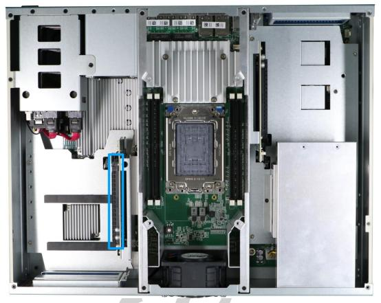
The system has two slots that are PCIe x16 Gen4 8-lanes (indicated in blue) for installing add-on cards, for additional I/O expansion or function cards such as a frame grabber card.
