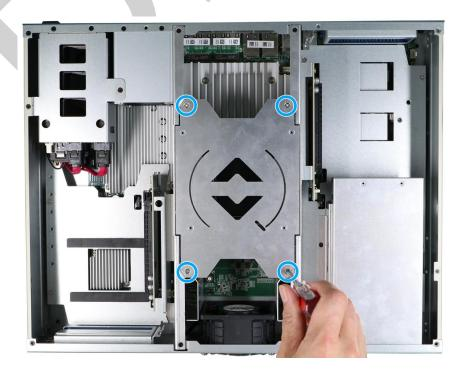
7. To access the mini-PCle and M.2 slots, remove the internal screws for the tunnel duct.
