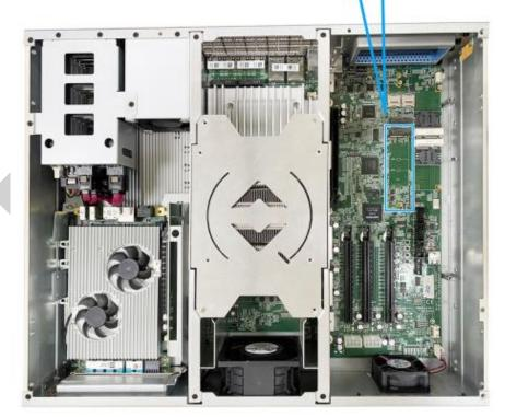
The system has a x4 PCIe M.2 2280 slot for you to install an NVMe SSD for the fast read/write performance. An NVMe SSD offers exceptional performance over 2.5" SSDs. For installation, please refer to the following instructions.
