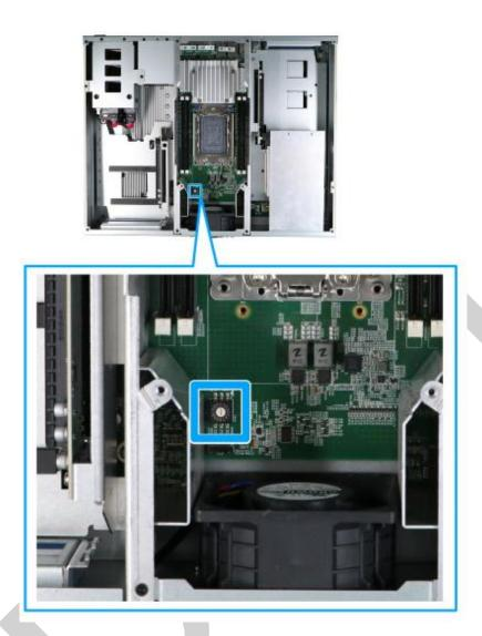
The ignition power control switch features multiple modes for pre and post ignition settings. Please refer to the section <u>Ignition Power Control</u> for details.
