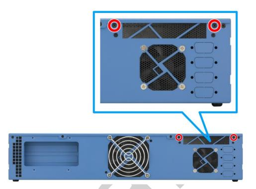
6. Secure the CPU/ DRAM cover if you removed it for installation.
