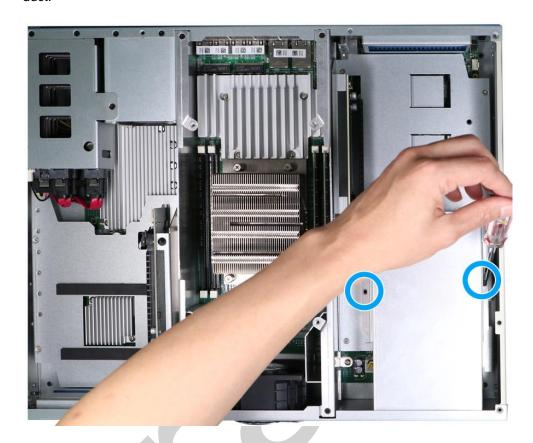
8. Remove the screws holding the tunnel duct at the rear, and remove the duct itself.
