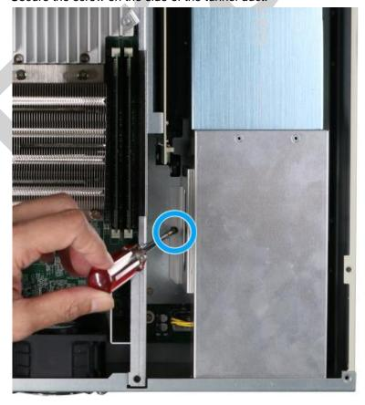
15. Secure the external screws for the tunnel duct on the rear panel to complete the inference accelerator installation.
