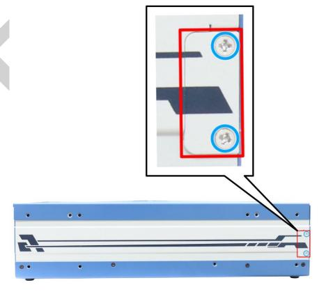
5. Secure the PCle card panel with a screw through the trap door.
