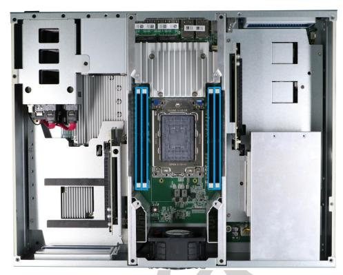
There are four DIMM memory slots (indicated in **blue**) on the motherboard that supports a total maximum of registered 512GB DDR4-3200. Please follow the procedures below to install the memory modules.
