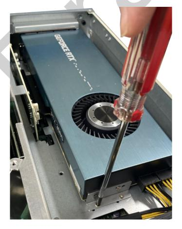
13. Place the tunnel duct back onto the inference accelerator and secure the screws indicated.
