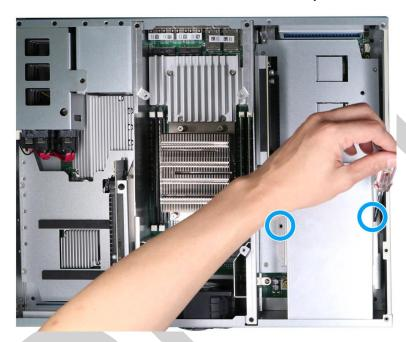
Screw on the side of the tunnel duct
