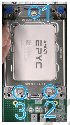
10. Remove the thermal paste protection film on the bottom of the CPU heatsink, lower the CPU heatsink onto the CPU/ socket, and secure the four screws. Make sure the screws are tightened gradually in the following order to ensure even pressure.
