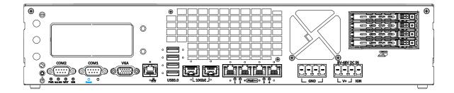
The reset button is used to manually reset the system in case of system halt or malfunction. To avoid unexpected reset, the button is purposely placed behind the panel. To reset, please use a pin-like object (eg. tip of a pen) to access the reset button
