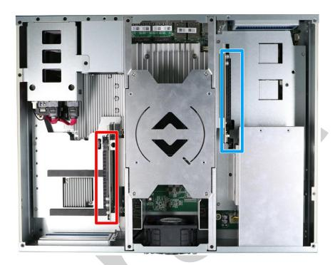
6. To access the CPU socket and DRAM slots, remove the four screws indicated and lift the cover.
