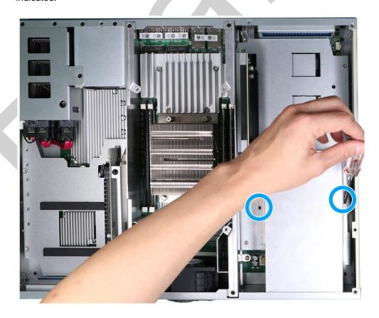
5. Secure the external screws for the tunnel duct.
