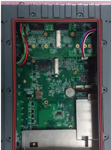
O-ring seated properly in the groove
