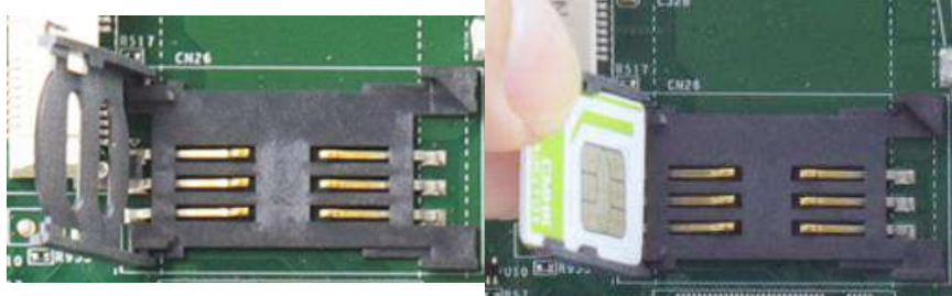
Slide and lift SIM card holder
