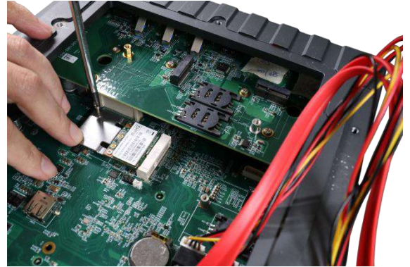
Secure the module with a screw
