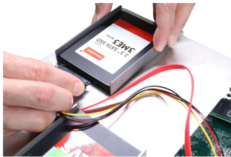
Disconnect the SATA/ power connector
