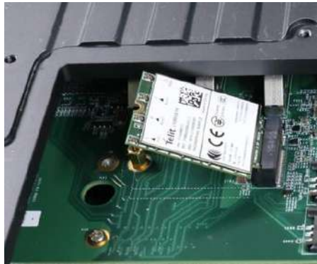
Insert into slot on a 45 degree angle
