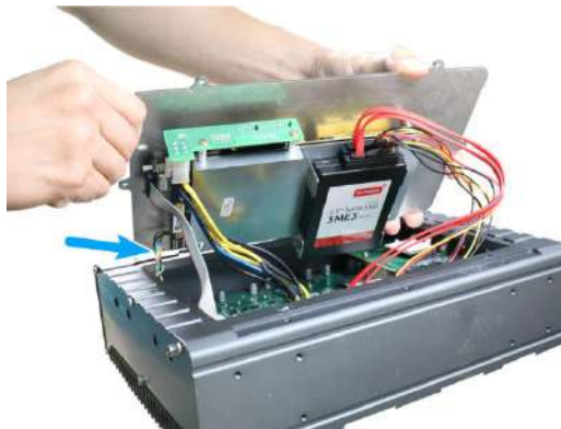
Connect the 4-pin power connector
