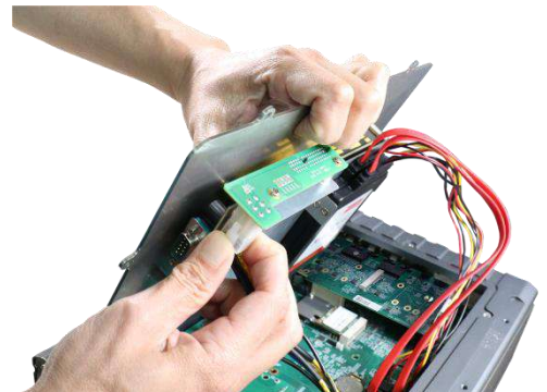
Unplug the 4-pin ATX connector
