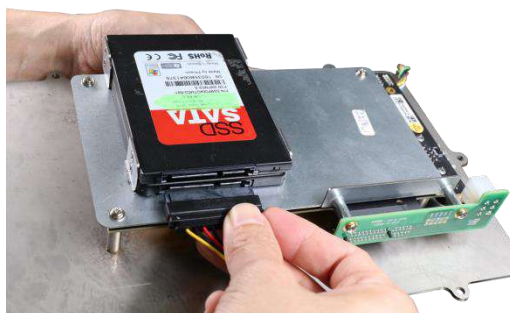
Connect the bottom hard drive first
