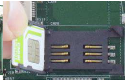
Insert SIM card with pins facing up
