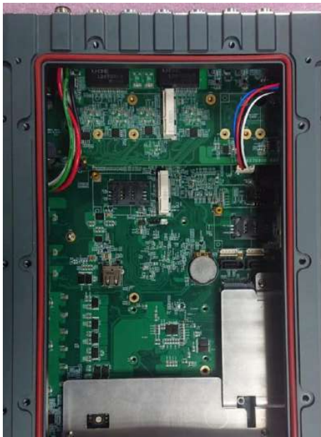
O-ring seated properly in the groove
