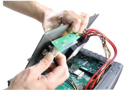
Plug in the 4-pin ATX connector
