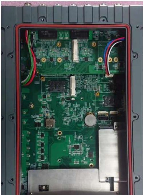
O-ring seated properly in the groove
