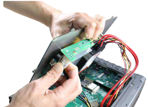
Unplug the 4-pin ATX connector
