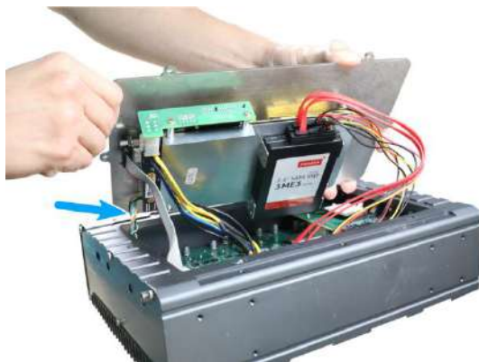
Disconnect the 4-pin power connector
