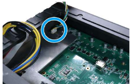
Unplug the 4-pin ATX connector
