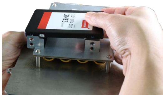
Place hard drive in between brackets
