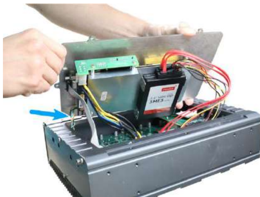
Disconnect the 4-pin power connector
