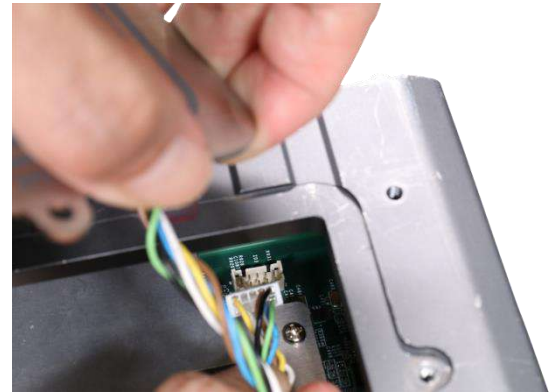
Connect from the motherboard side
