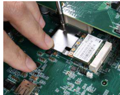
Secure the module with a screw
