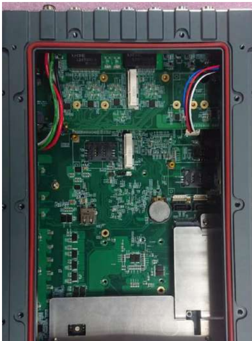
O-ring seated properly in the groove
