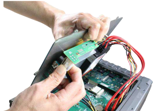
Unplug the 4-pin ATX connector
