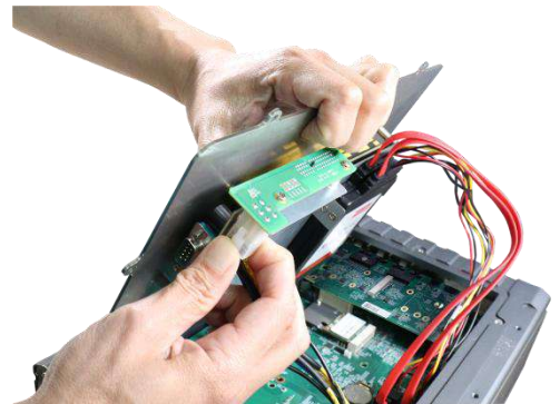
Unplug the 4-pin ATX connector
