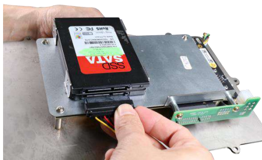
Connect the bottom hard drive first
