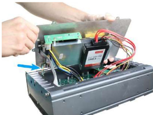
Disconnect the 4-pin power connector
