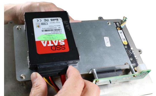
Then connect the hard drive on top (if installed)
