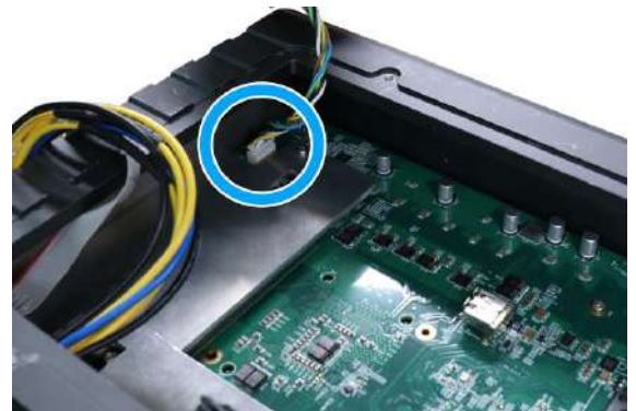
Unplug the 4-pin ATX connector
