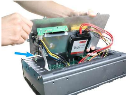
Connect the 4-pin power connector
