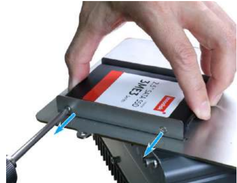
Remove screws on both sides of the hard drive
