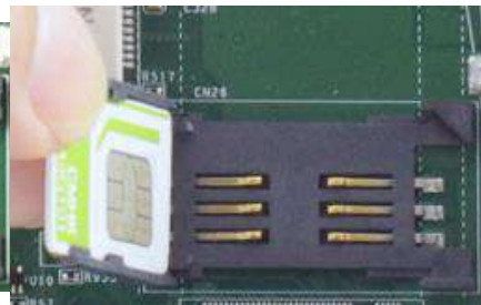
Insert SIM card with pins facing up
