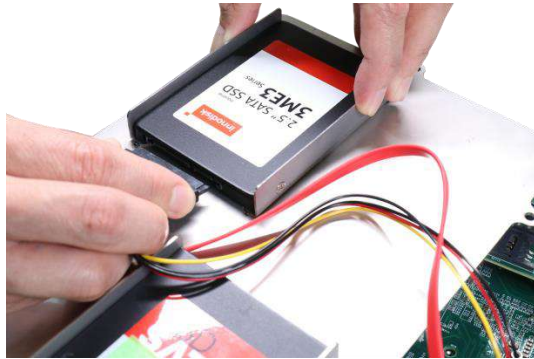
Disconnect the SATA/ power connector
