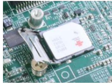
Flip-open the holder and place SIM
