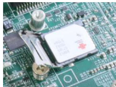
Flip-open the holder and place SIM
